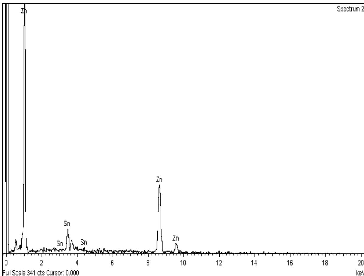
Figure 7. EDS analysis of the plated surface of sample in Fig.3 (iv)
