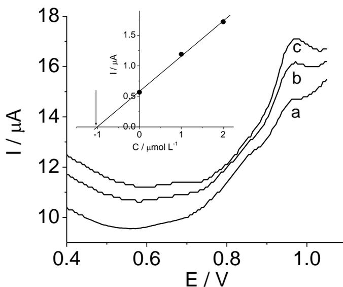
**Figure 8.** Determination of *Carbendazim* in spiked Labe river sample. Adsorptive stripping differential pulse voltammetric curves obtained for spiked river water sample (curve **a**) and successive standard additions of *Carbendazim* (curves **b** and **c**). The inset shows the corresponding analytical plot.
