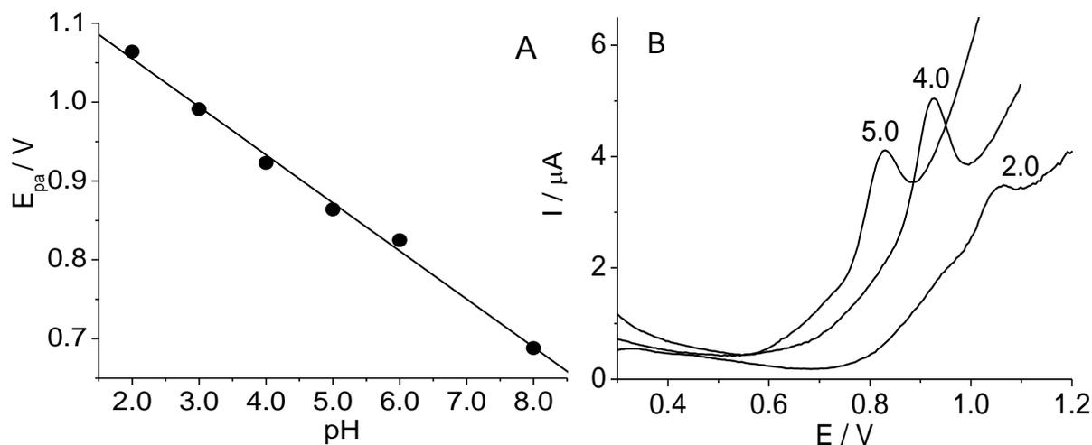
**Figure 2.** pH dependence of the *Carbazepim* oxidation signal recorded with TCP-CPE: A)  $E_{pa}$ -pH plot based on CV curves recorded in Britton-Robinson buffer from pH 2.0 to 8.0 while  $\nu = 100 \text{ mV s}^{-1}$ , containing  $3 \cdot 10^{-5} \text{ mol L}^{-1}$  MBC and B) Illustrative DPAdSV curves (deposition potential,  $-0.35 \text{ V}$ ; deposition time, 120 s; equilibrium time, 5 s; Britton-Robinson buffers (pH 2.0, 4.0, and 5.0)).
