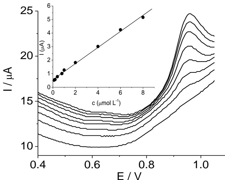
**Figure 7.** Adsorptive stripping differential pulse voltammograms recorded at TCP-CPE and in the presence of  $3.6 \cdot 10^{-5} \text{ mol L}^{-1}$  HPCD for different concentrations of *Carbendazim* in Britton-Robinson buffer (pH 4.0). The corresponding calibration plot is shown in the inset.  $E_{\text{acc}} -0.35 \text{ V}$ ,  $t_{\text{acc}} 120 \text{ s}$ ,  $t_{\text{ep}} 5 \text{ s}$ .
