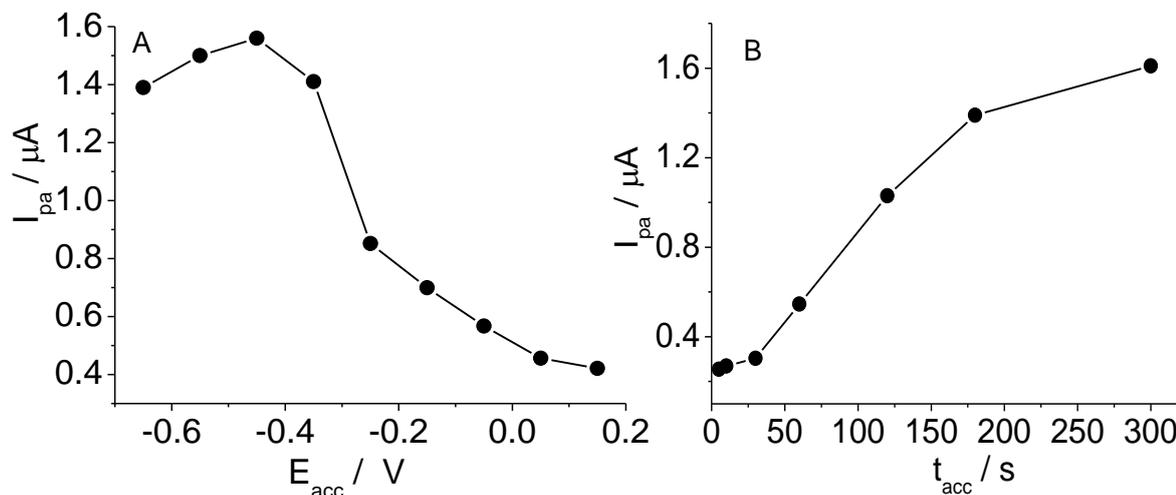
**Figure 5.** Key parameter optimization for adsorptive stripping differential pulse voltammetric determination of MBC ( $3 \cdot 10^{-6}$  mol L $^{-1}$ ) in Britton–Robinson buffer pH 4.0: A) Influence of  $E_{acc}$  on  $I_{pa}$  values 120 s  $t_{acc}$  and B) Effect of  $t_{acc}$  at  $E_{acc} = -0.35$  V. All other DPAdSV variables are as those in Fig 2.
