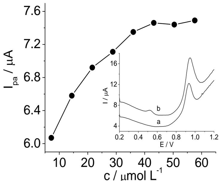
**Figure 6.** Dependence of  $I_{pa}$  height of MBC on the concentration of 2-hydroxypropyle- $\beta$ -cyclodextrin in Britton-Robinson buffer pH 4.0. Inset:  $1 \cdot 10^{-5} \text{ mol L}^{-1}$  MBC (curve a), and  $1 \cdot 10^{-5} \text{ mol L}^{-1}$  MBC +  $3.6 \cdot 10^{-5} \text{ mol L}^{-1}$  (curve b).  $E_{acc} = -0.35\text{V}$ ,  $t_{acc} = 120 \text{ s}$ .
