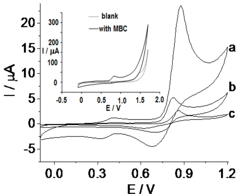
**Figure 1.** Cyclic voltammograms of *Carbendazim* at sub-millimolar level in Britton–Robinson buffer (pH 8.0) on CPEs based on different binders: a) tricresyl-phosphate, b) mineral oil, c) silicone oil. Inset: cyclic voltammograms of blank Britton–Robinson buffer pH 8.0 (dotted line) and  $5.2 \times 10^{-4} \text{ mol L}^{-1}$  *Carbendazim* (full line) obtained by TCP-CPE.  $\nu = 100 \text{ mV s}^{-1}$ .
