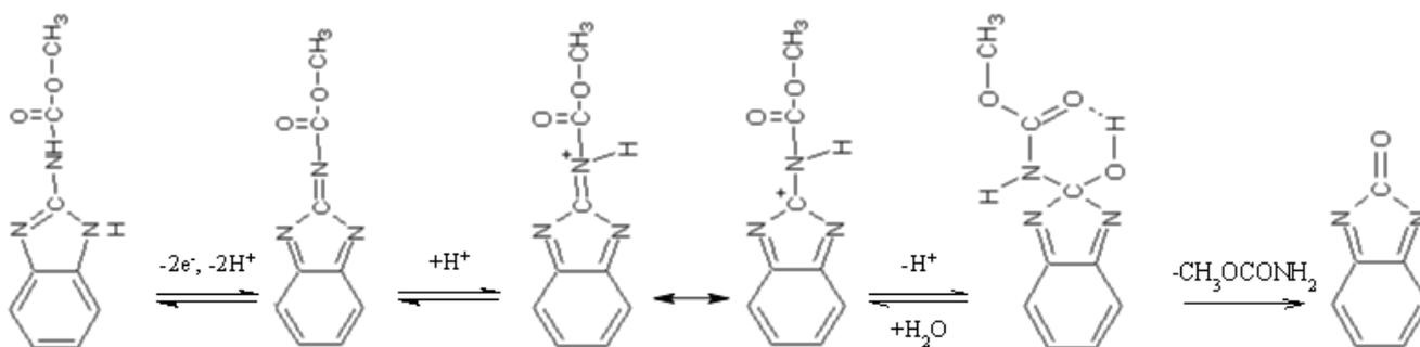
**Figure 4.** Oxidation mechanism of *Carbendazim* at TCP-CPE in Britton-Robinson buffer (pH 4.0).
