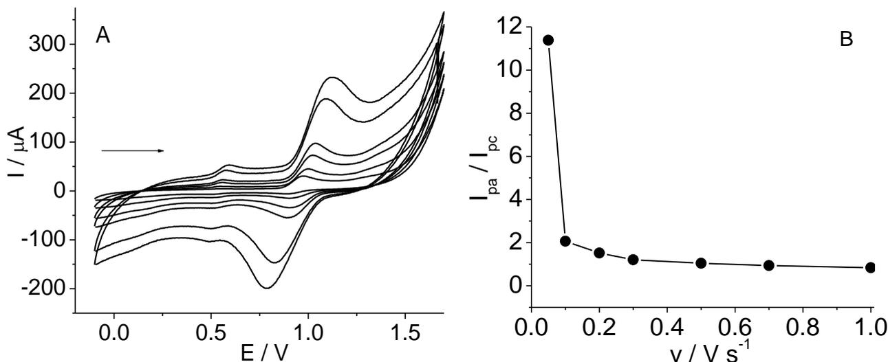
**Figure 3.** Effect of the CV scan rate for oxidation peak of *Carbendazim* ( $5.2 \cdot 10^{-4} \text{ mol L}^{-1}$ ) and its counterpart in Britton-Robinson buffer solution (pH 4.0) obtained with TCP-CPE: A) Scan rates: 50, 100, 200, 300, 500, 700 and 1000  $\text{mV s}^{-1}$  and B) Ratio of  $I_{pa}$  and  $I_{pc}$  recorded at the appropriate different scan rates.
