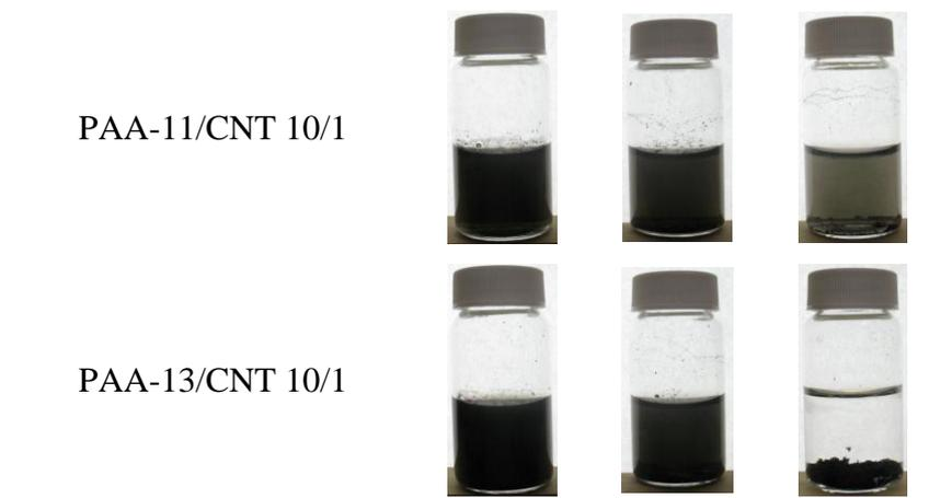
**Figure 1.** Photos (taken immediately, 24 h, and 48 h after 10 min of sonication) of the PAA-pH/CNT 10/1 dispersion in 10 mL of water of different pH.
