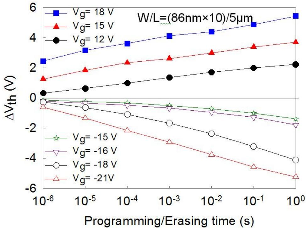
Figure 4. Program and erase (P/E) characteristics of the NWs TANOS devices.
