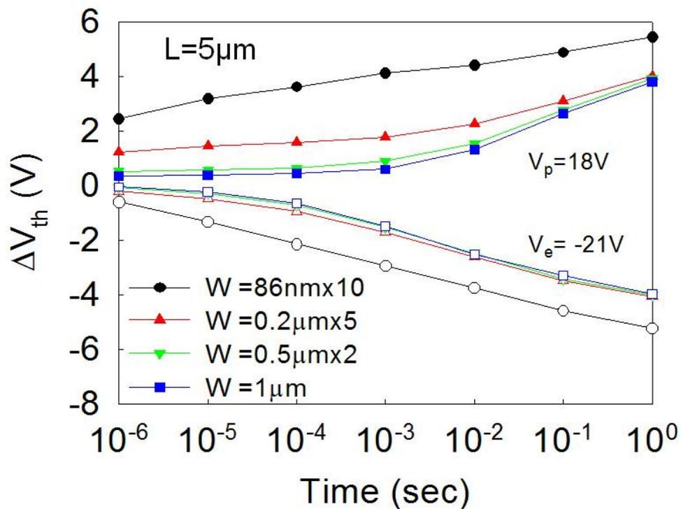
Figure 5. Program and erase characteristics of various different channel width and length TANOS devices
