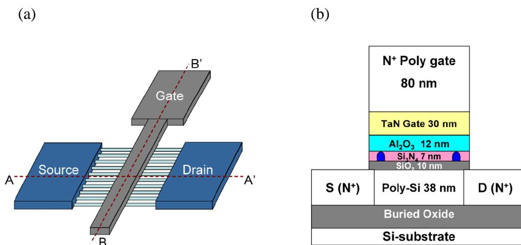
**Figure 1.** (a) Top view scheme of the Pi-gate NWs TANOS NVM. (b) Cross-section scheme of TANOS device along A-A' direction.
