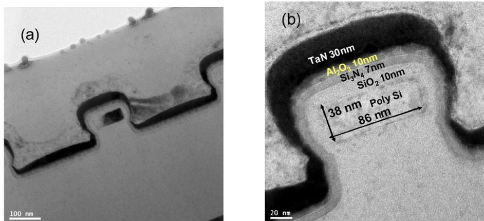
**Figure 2.** (a) TEM image of Pi-gate NWs TANOS NVM structure. (b) Magnification TEM image of figure 2(a). The stacked gate dielectric are SiO<sub>2</sub> = 10 nm / Si<sub>3</sub>N<sub>4</sub> = 7 nm / Al<sub>2</sub>O<sub>3</sub> = 12 nm, and each poly-Si NW width is 86 nm.
