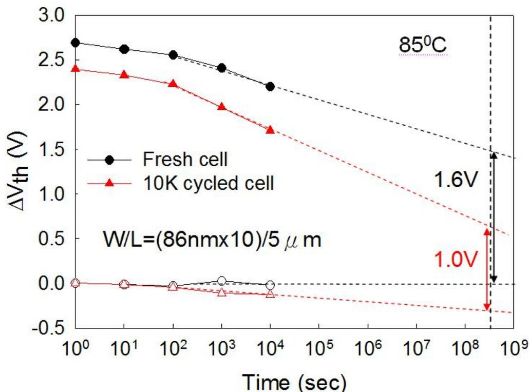
**Figure 7.** Retention characteristics of Pi-gate NWs TANOS NVM.
