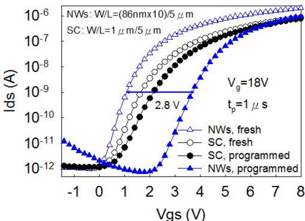
**Figure 3.**  $I_{ds}$ - $V_{gs}$  curve of the poly-Si NWs and the single-channel (SC) TANOS memories.
