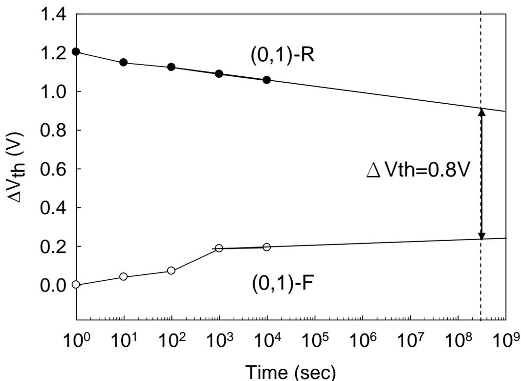
**Figure 10.** Bit-D retention characteristics of Pi-gate NWs TANOS NVM.
