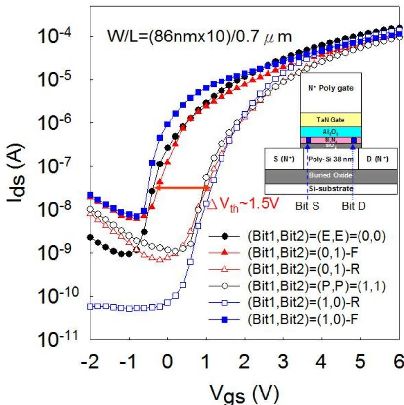
**Figure 9.** The two-bit  $I_d - V_g$  curves of Pi-gate NWs TANOS NVM. As an example (Bit-S, Bit-D)-read mode = (0,1)-R denotes Bit-S in its erased state and Bit-D is programmed under reverse read. High  $V_{th}$  is obtained under R-read.
