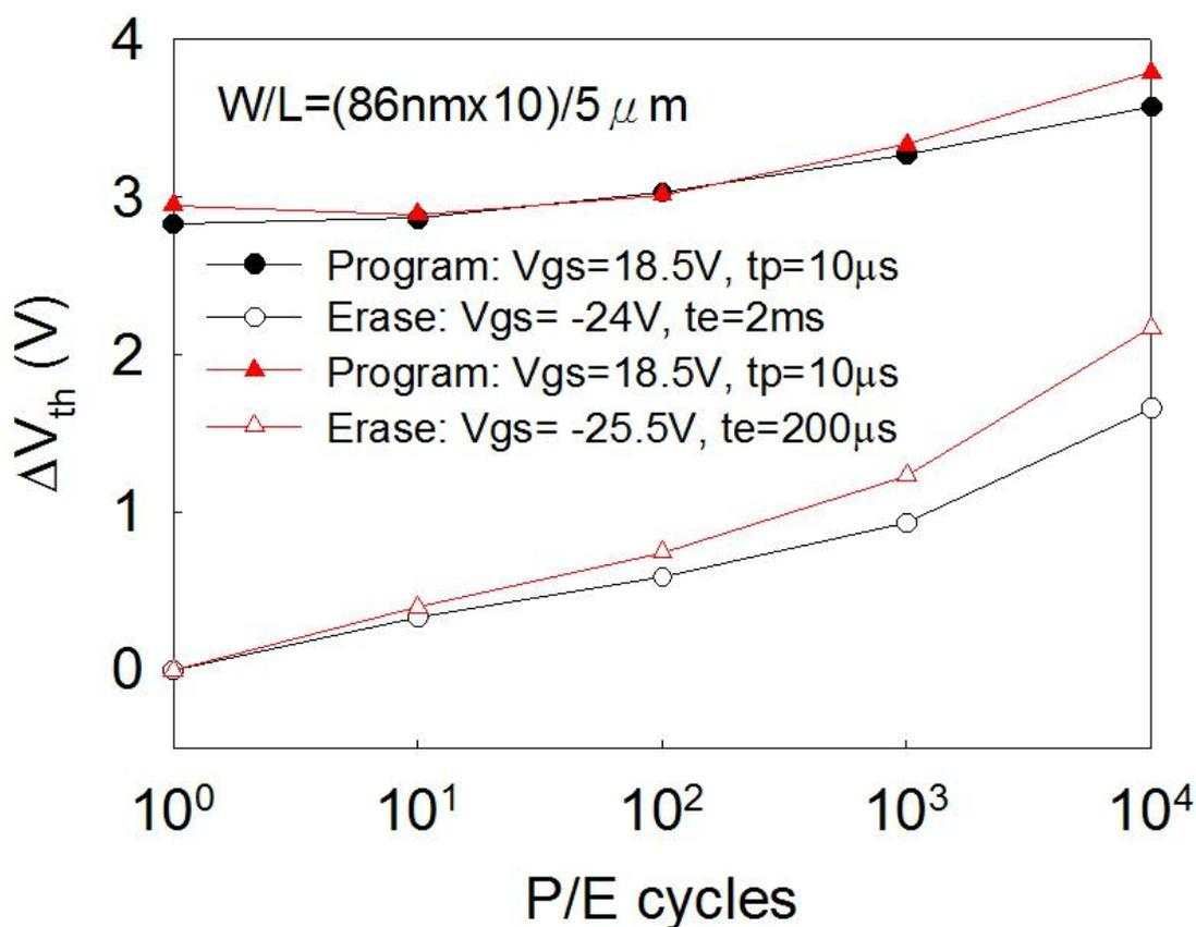
Figure 6. Endurance characteristics of Pi-gate NWs TANOS NVM.
