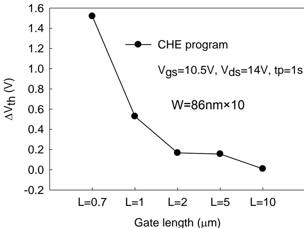
**Figure 8.** Threshold voltage shift ( $\Delta V_{th}$ ) of the Pi-gate NWs TANOS NVM for different gate length (L).
