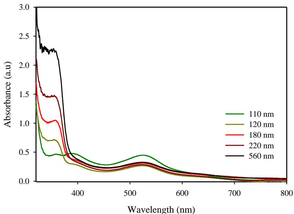
**Figure 4.** UV-VIS optical absorption spectra of quasi ZnO nanorods coated with N719 dye with various thicknesses
