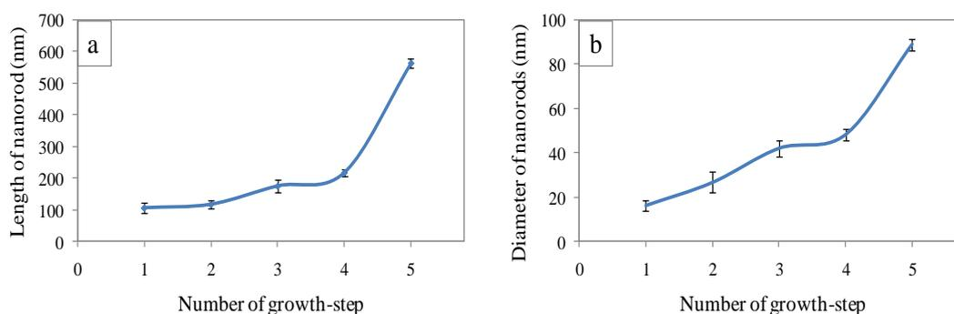
**Figure 3.** a) Variation of length and b) diameter of ZnO nanorods with number of growth steps
