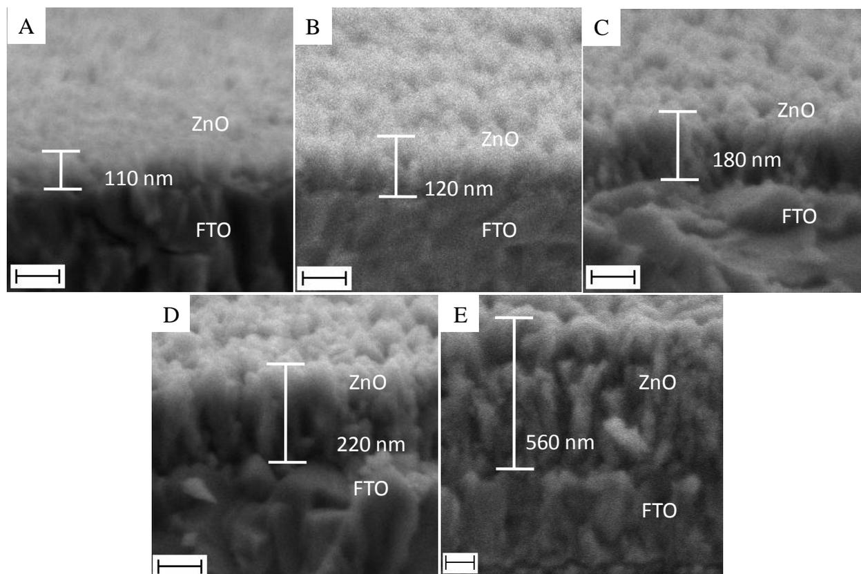
**Figure 2.** Cross sectional FESEM micrograph of  $\text{ZnO}$  nanorod via multiple growth step: A) 1× growth step, B) 2× growth steps, C) 3× growth steps, D) 4× growth steps and E) 5× growth steps. Scale bar 100 nm
