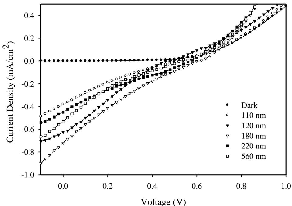
**Figure 5.**  $J$ - $V$  curves of the dye sensitized solar cell of FTO/ZnO-dye/electrolyte/platinum
