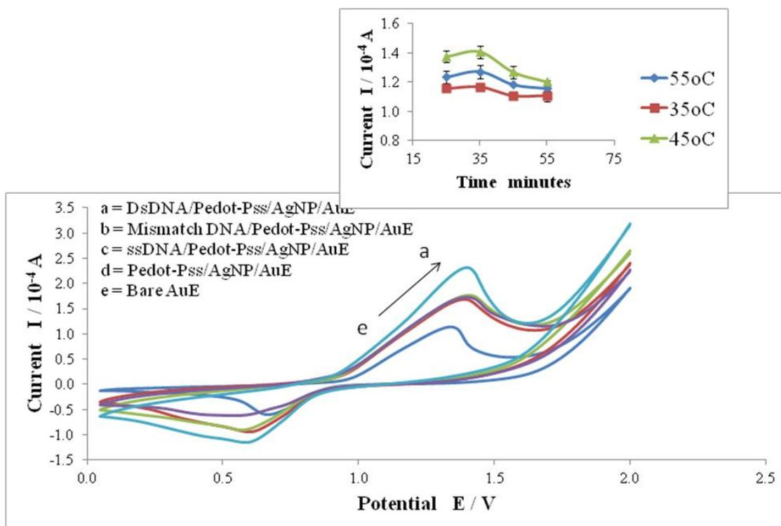
**Figure 3.** Redox signals for (a) dsDNA/PEDOT-PSS/AgNPs/AuE, (b) mismatch DNA/PEDOT-PSS/AgNPs/AuE, (c) ssDNA/PEDOT-PSS/AgNPs/AuE, (d) PEDOT-PSS/AgNPs/AuE, (e) bare AuE at scan rate 100 mV/s
