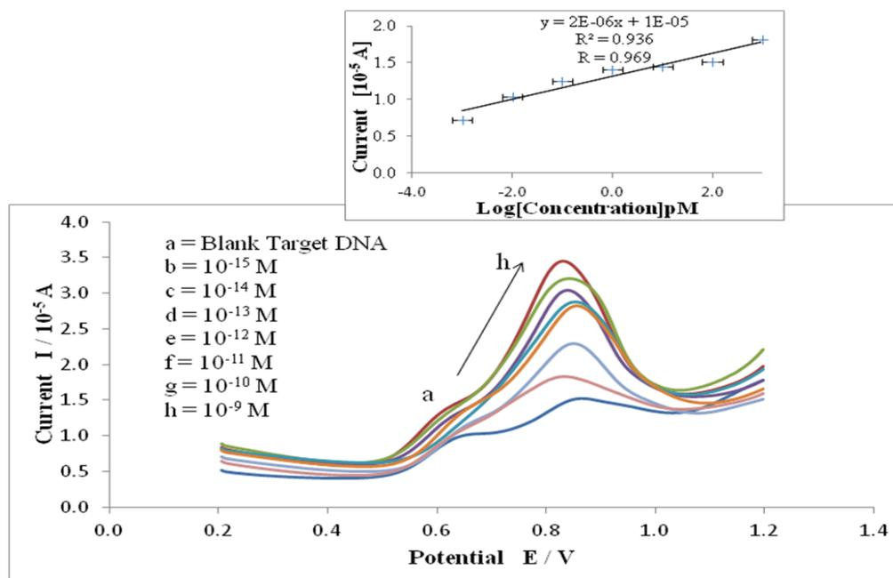
**Figure 4.** Differential pulse voltammograms (DPV) of the electrochemical analysis of the probe DNA on a nanocomposite platform showing current drop to target DNA concentration of (a) blank, (b)  $1.00 \times 10^{-15}$  M, (c)  $1.00 \times 10^{-14}$  M, (d)  $1.00 \times 10^{-13}$  M, (e)  $1.00 \times 10^{-12}$  M, (f)  $1.00 \times 10^{-11}$  M, (g)  $1.00 \times 10^{-10}$  M, (h)  $1.00 \times 10^{-9}$  M at scan rate 100mV/s.
