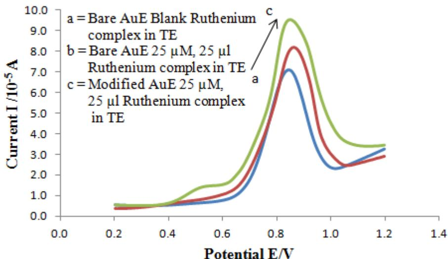
**Figure 2.** DPV carried out in TE buffer of (a) bare AuE without, (b) bare AuE with, (c) modified AuE with Ruthenium complex
