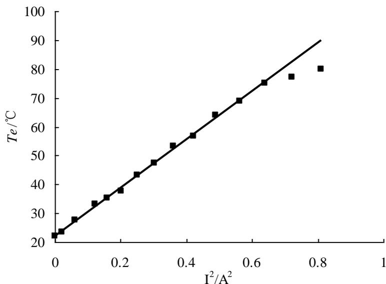
**Figure 1.** Relationship between the square of the heating current ( $I^2$ ) and  $T_e$ .
