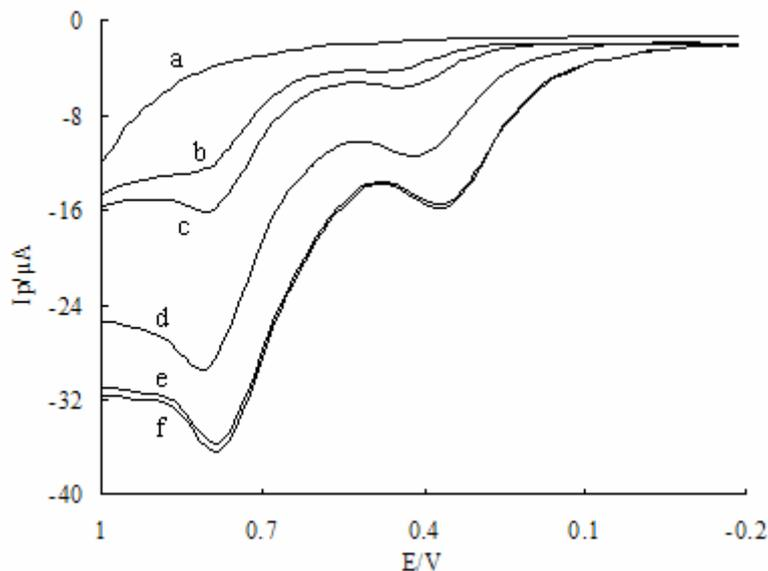
**Figure 4.** SWVs of hydrolyzing product of cephalixin at different electrode temperatures. a, 22 °C; b, 40 °C; c, 50 °C; d, 60 °C; e, 70 °C; f, 75 °C; Other conditions are the same as in Fig. 2.
