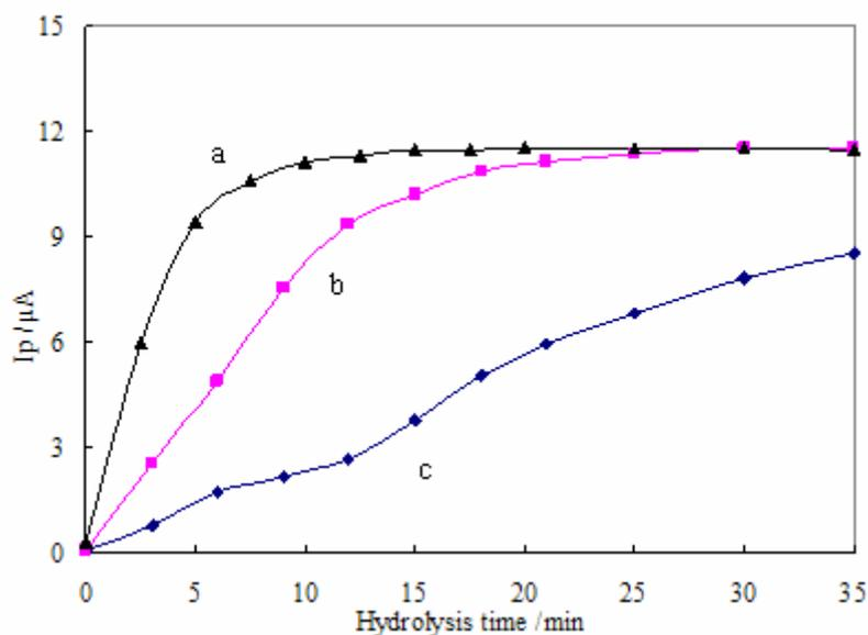
**Figure 5.** Plots of the peak current vs. heating time. a, 70 °C by HGCE; b, 100 °C by oil bath; c, 70 °C by oil bath; Other conditions are the same as in Fig. 2.
