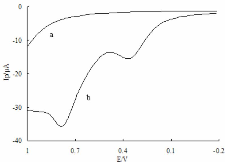
**Figure 2.** SWVs of cephalosporin before (a) and after (b) its hydrolysis. [cephalosporin]=10  $\mu\text{mol}\cdot\text{L}^{-1}$ ; SW frequency, 50Hz; SW pulse amplitude, 45mV; detect buffer, PBS (pH=11.73, 0.2  $\text{mol}\cdot\text{L}^{-1}$ ); hydrolysis time, 15 min; hydrolysis medium, NaOH(0.1  $\text{mol}\cdot\text{L}^{-1}$ ).
