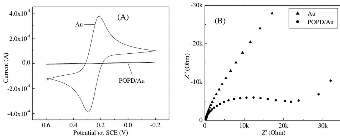
**Figure 1.** (A) Cyclic voltammograms of Au and PoPD/Au electrodes in 20 mmol/L  $K_3Fe(CN)_6$ , 20 mmol/L  $K_4Fe(CN)_6$  + 0.5 mol/L KCl solution at scan rate 50 mV/s. (B) Nyquist plots for Au, PoPD/Au electrode in the same solution as above measured at fixed DC potential 0V (vs. SCE) with amplitude 5 mV. The frequency range is 100 KHz ~ 10 mHz.
