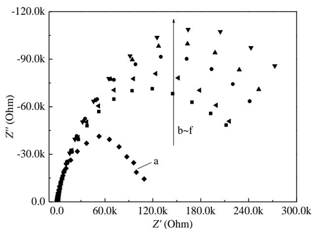
**Figure 2.** Nyquist plots of immunosensor at different processes, (a)Au, (b)PoPD/Au, (c)GA-PoPD/Au, (d)Ab/GA-PoPD/Au, (e)BSA-Ab/GA-PoPD/Au, (f) Ag/BSA-Ab/GA-PoPD/ Au.
