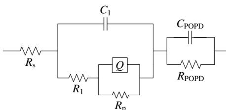
**Figure 4.** Equivalent circuit of interface modeling of biomolecular recognition for the immunosensor.
