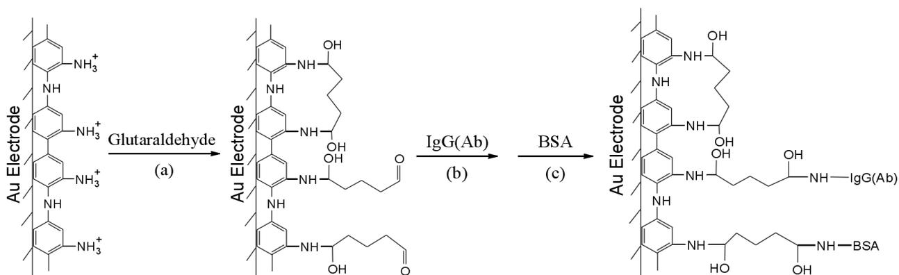
**Figure 3.** Schematic diagram for reaction mechanism during immunosensor assembly procedure.
