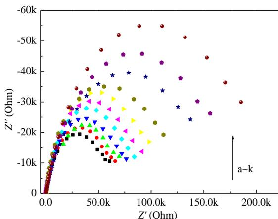
**Figure 5.** Nyquist plots for Ag/BSA-Ab/GA-PoPD/Au electrode after incubating the immunosensor in IgG solution with concentration of 0 (a), 0.1 (b), 1 (c), 3 (d), 5 (e), 7 (f), 10 (g), 60 (h), 450 (i), 750 (j), 1000 (k) ng/mL, respectively.
