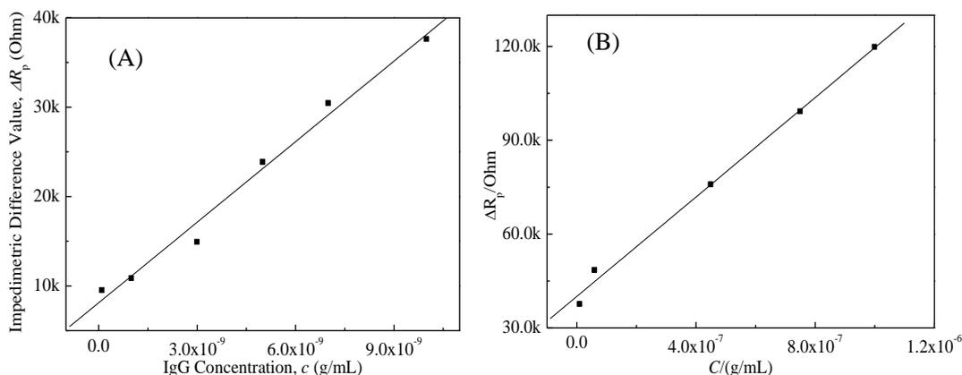
**Figure 6.** (A) Calibration plot for IgG concentration ranging from 0.1 to 10 ng/mL. (B) Calibration plot for IgG concentration ranging from 10 to 1000 ng/mL.
