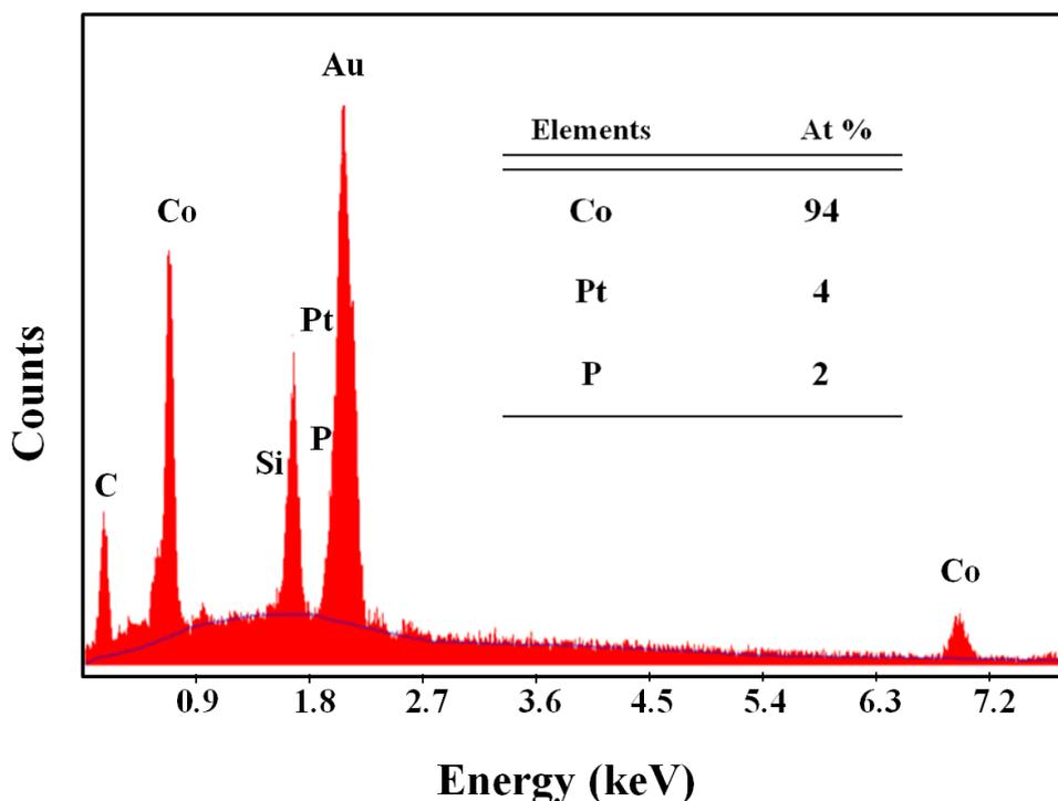
**Figure 2.** Energy dispersive spectrums of CoPtP/ Au multisegmented nanowires ( Inset table shows the elemental composition of CoPtP nanowires )
