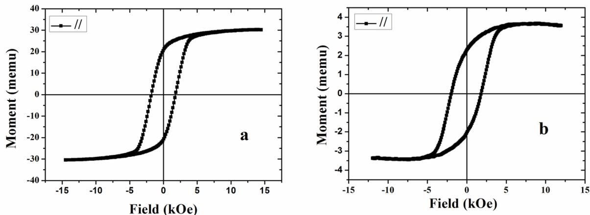
**Figure 3.** Hysteresis loops measured at room temperature of (a) CoPtP nanowires (b) CoPtP/Au multisegmented nanowires
