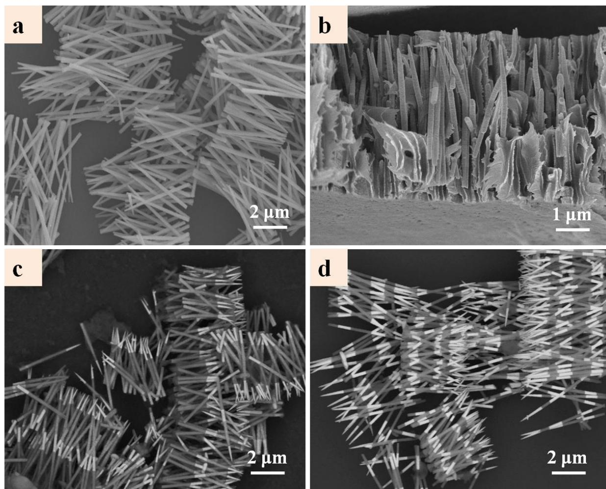
**Figure 1.** FE-SEM image of CoPtP nanowires (a) after removal of the membrane (b) cross-sectional view of the membrane with nanowires, Backscattering images of CoPtP/Au nanowires (c) four segmented (d) six segmented
