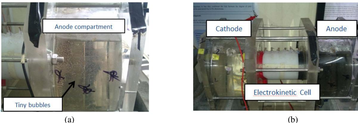
**Figure 3.** Tiny bubbles produced in the Anode, (a) in 1 day (b) After 5 days treatment time.
