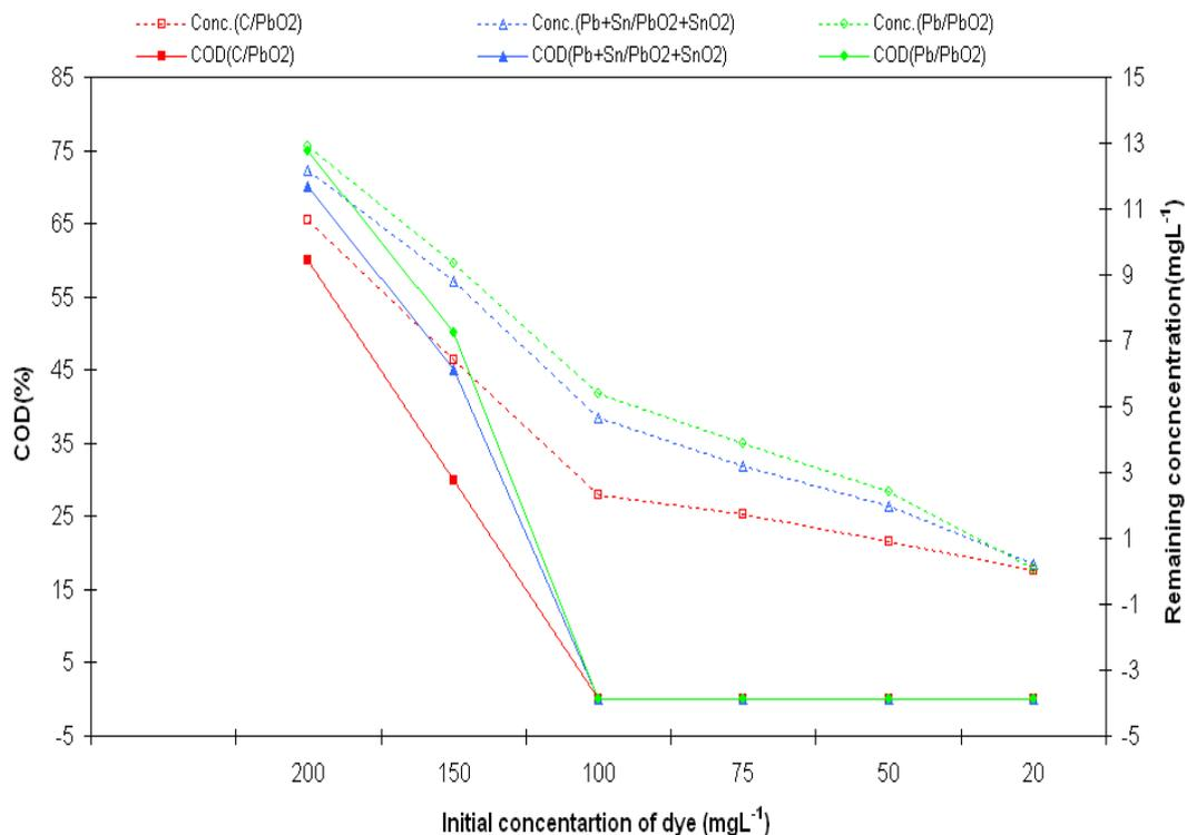
**Figure 6.** The effect of initial concentration on RO7 and COD removal using C/PbO<sub>2</sub>, Pb+Sn/PbO<sub>2</sub>+SnO<sub>2</sub> and Pb/PbO<sub>2</sub> electrodes.
