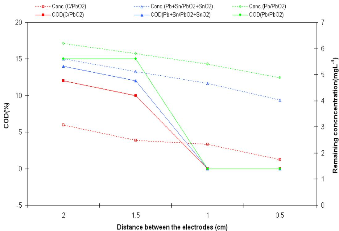
**Figure 7.** The effect of distance between the cathode and anode on RO7 and COD removal using C/PbO<sub>2</sub>, Pb+Sn/PbO<sub>2</sub>+SnO<sub>2</sub> and Pb/PbO<sub>2</sub> electrodes.
