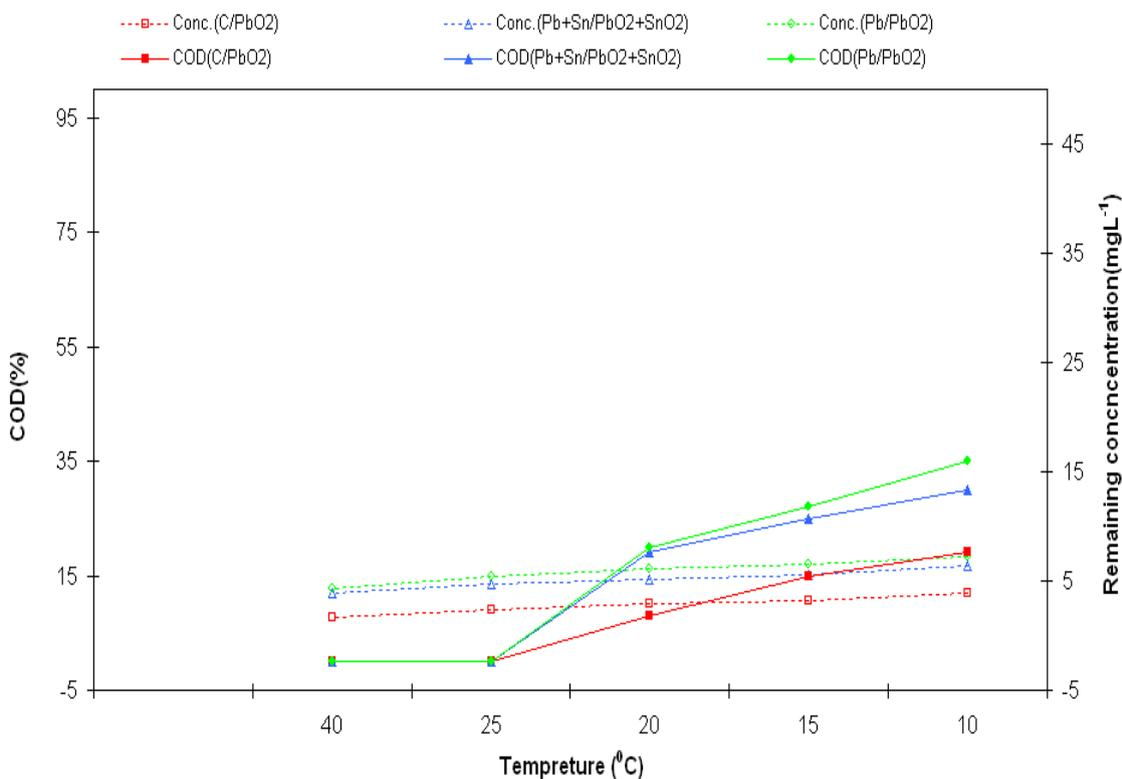
**Figure 5.** The effect of temperature on RO7 and COD removal using C/PbO<sub>2</sub>, Pb+Sn/PbO<sub>2</sub>+SnO<sub>2</sub> and Pb/PbO<sub>2</sub> electrodes.
