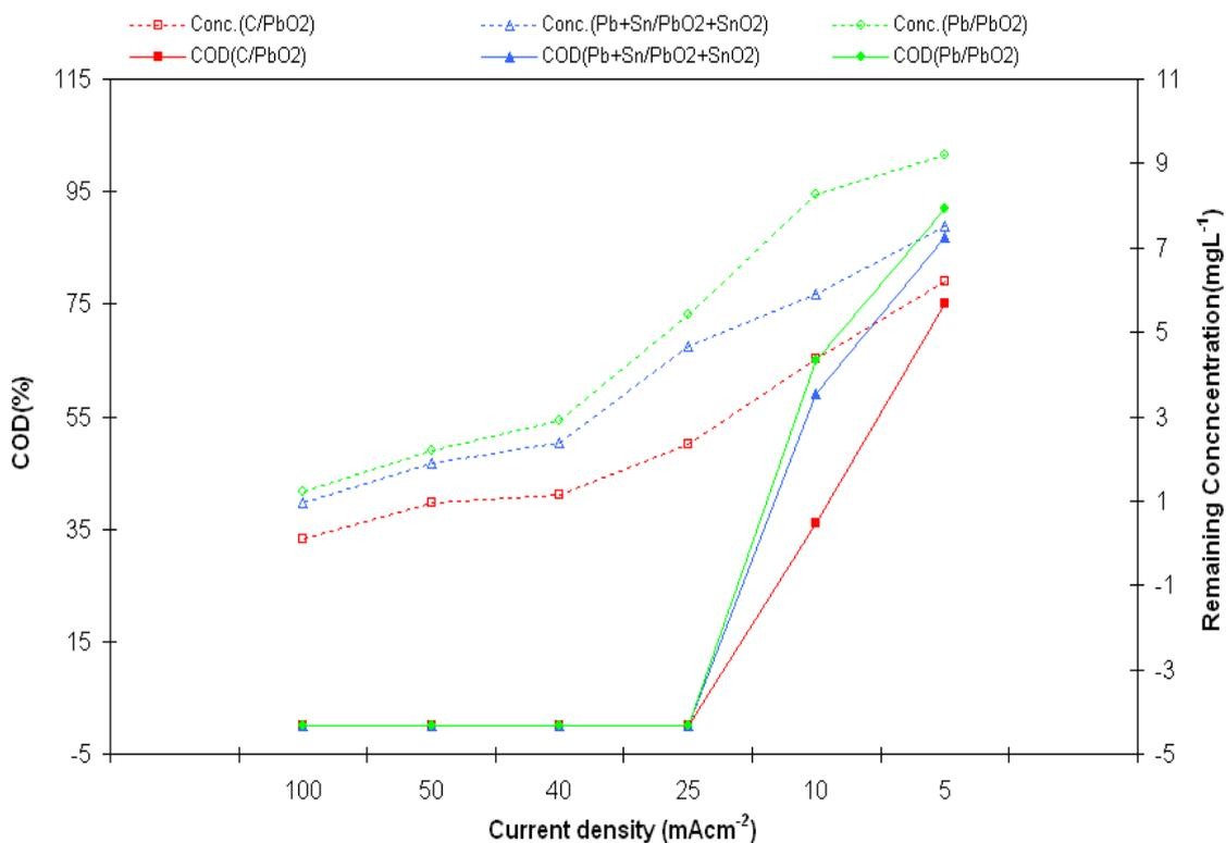
**Figure 3.** The effect of current density on RO7 and COD removal using C/PbO<sub>2</sub>, Pb+Sn/PbO<sub>2</sub>+SnO<sub>2</sub> and Pb/PbO<sub>2</sub> electrodes.
