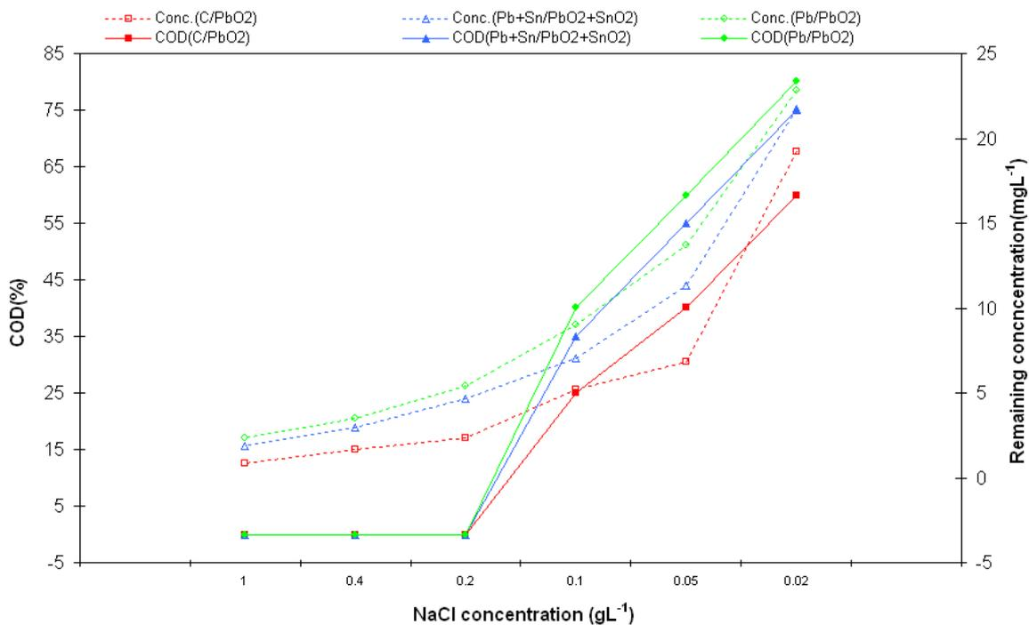
**Figure 2.** The effect of NaCl concentration on RO7 and COD removal using C/PbO<sub>2</sub>, Pb+Sn/PbO<sub>2</sub>+SnO<sub>2</sub> and Pb/PbO<sub>2</sub> electrodes.
