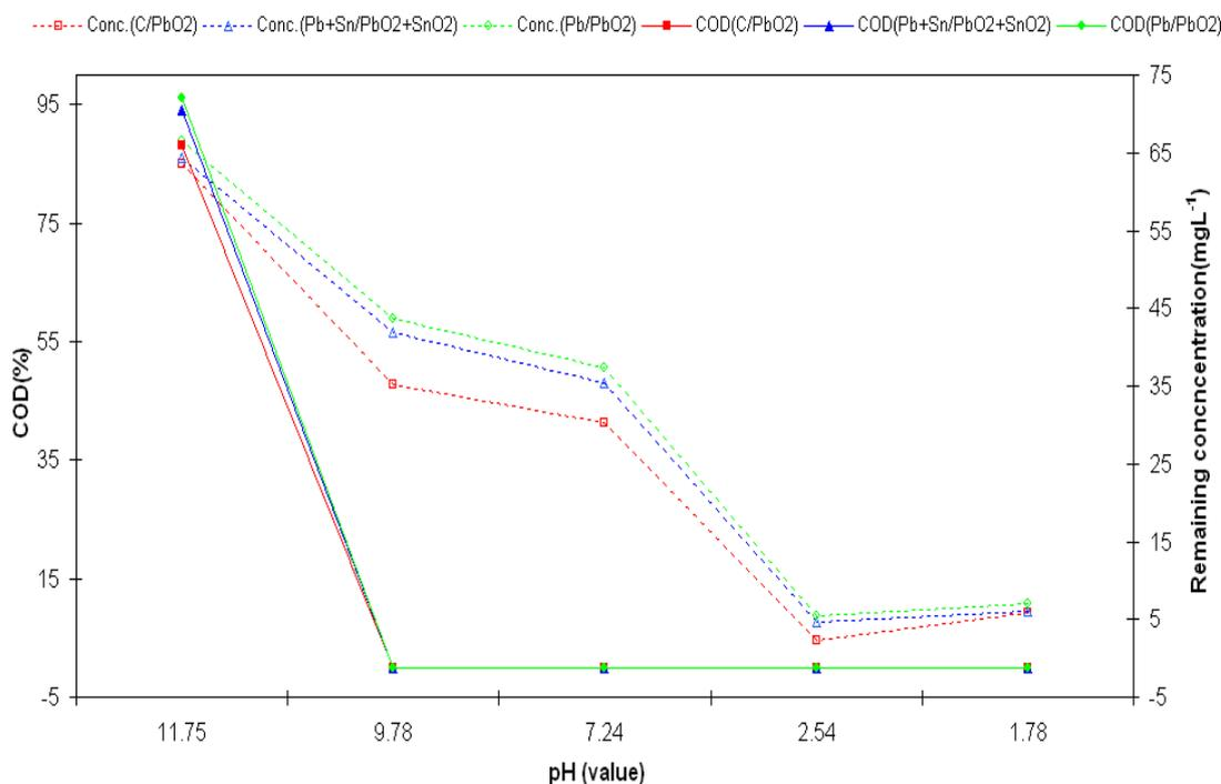
**Figure 1.** The effect of pH on RO7 and COD removal using C/PbO<sub>2</sub>, Pb+Sn/PbO<sub>2</sub>+SnO<sub>2</sub> and Pb/PbO<sub>2</sub> electrodes.
