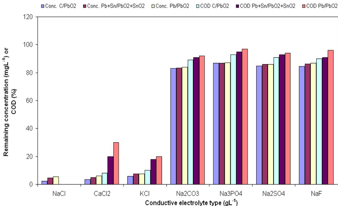
**Figure 4.** The effect of the conductive electrolyte type on RO7 and COD removal using C/PbO<sub>2</sub>, Pb+Sn/PbO<sub>2</sub>+SnO<sub>2</sub> and Pb/PbO<sub>2</sub> electrodes.
