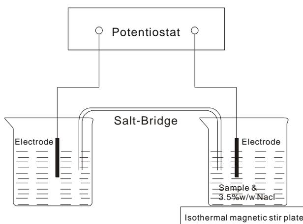
**Figure 1.** Schematic diagram of the micro-electrolysis device
