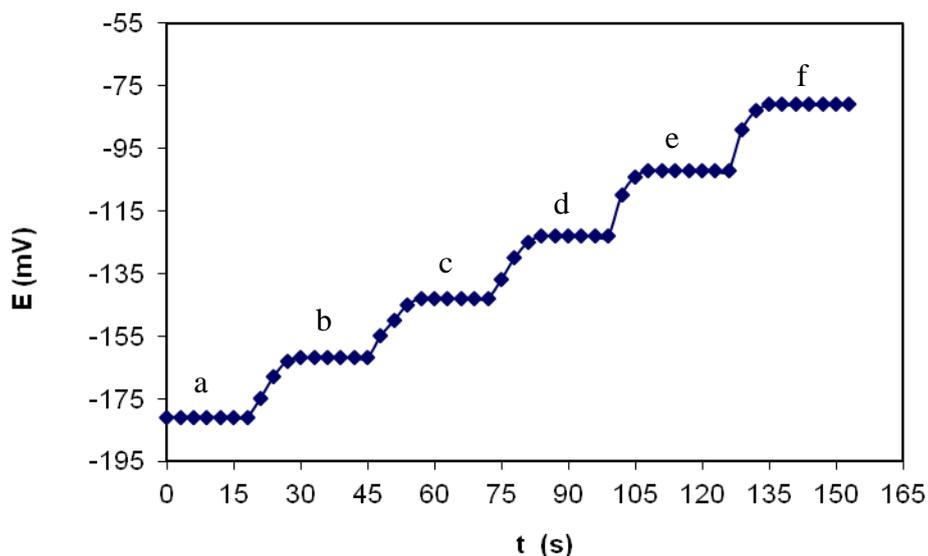
**Figure 4.** The practical response time of the Dy(III) membrane sensor for step changes in the Dy(III) concentration: (a)  $1.0 \times 10^{-7}$  mol L<sup>-1</sup>, (b)  $1.0 \times 10^{-6}$  mol L<sup>-1</sup>, (c)  $1.0 \times 10^{-5}$  mol L<sup>-1</sup>, (d)  $1.0 \times 10^{-4}$  mol L<sup>-1</sup>, (e)  $1.0 \times 10^{-3}$  mol L<sup>-1</sup>, (f)  $1.0 \times 10^{-2}$  mol L<sup>-1</sup>.
