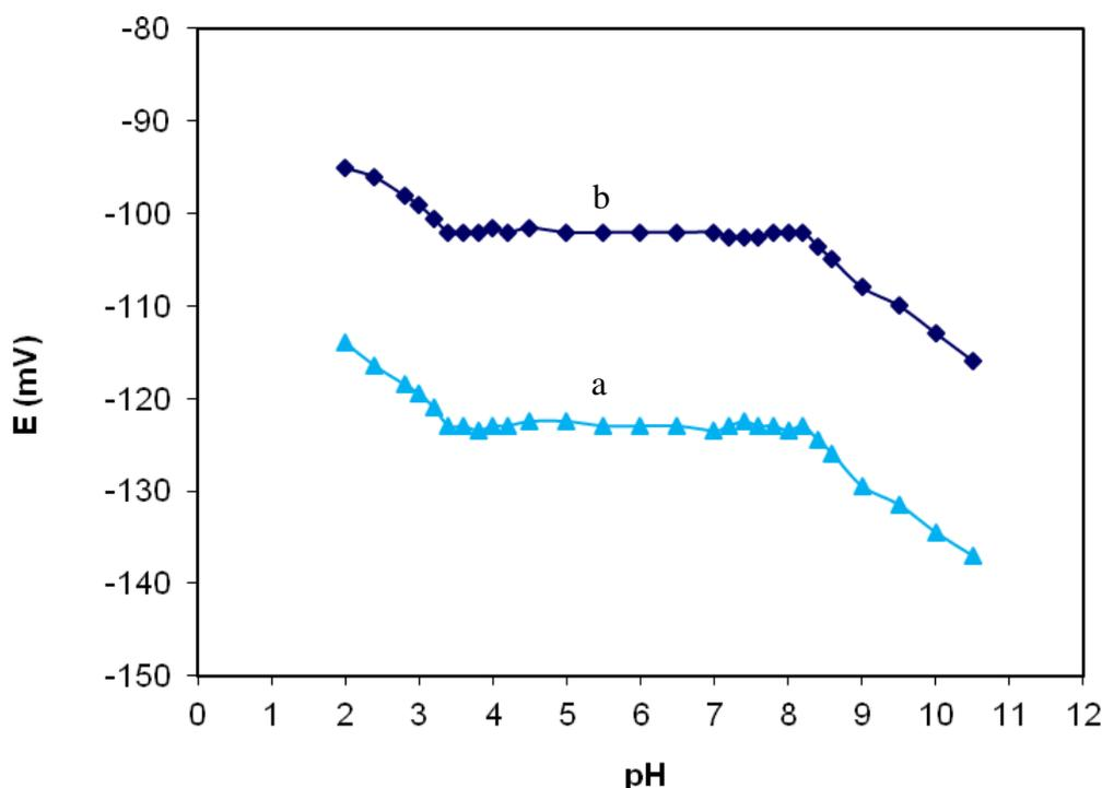
**Figure 5.** pH effect on the potential response of the Dy(III) membrane sensor based on DPDP in the test solutions of Dy(III) ions: (a)  $1.0 \times 10^{-4}$  mol L<sup>-1</sup>, (b)  $1.0 \times 10^{-3}$  mol L<sup>-1</sup>.
