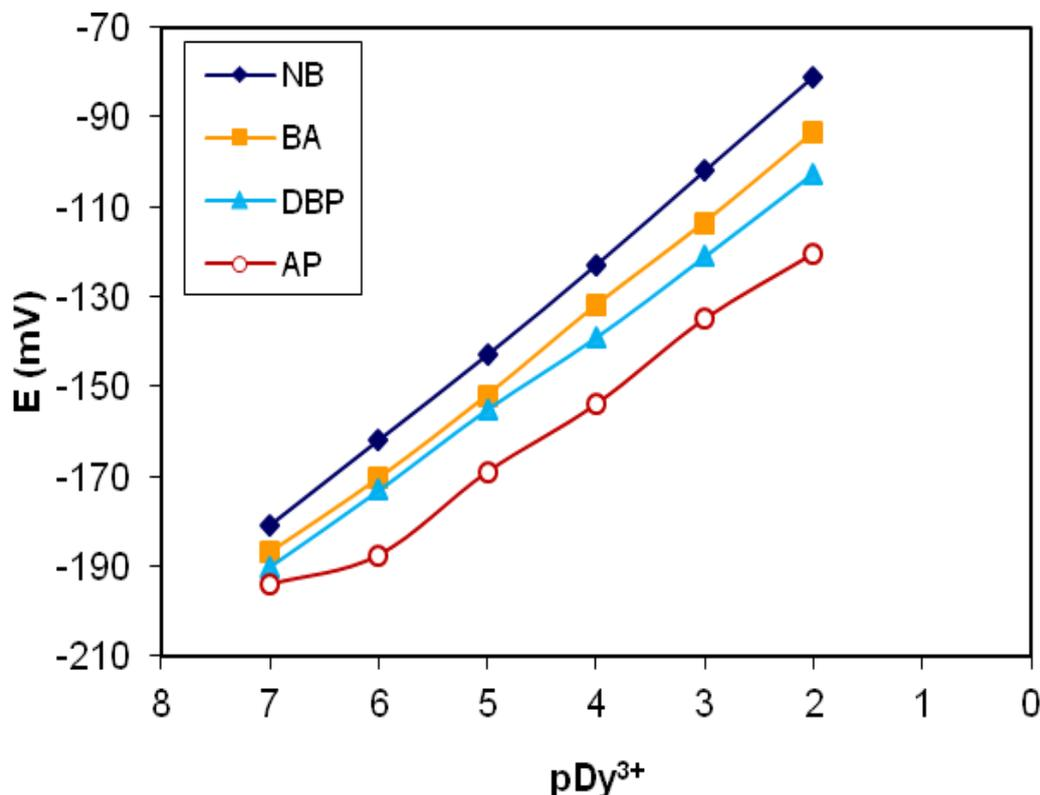
**Figure 2.** The potential responses of the Dy(III) membrane ISEs prepared with different plasticizers.
