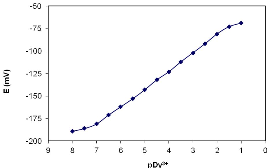
**Figure 3.** The Calibration curve of the Dy(III) membrane sensor based on DPDP.
