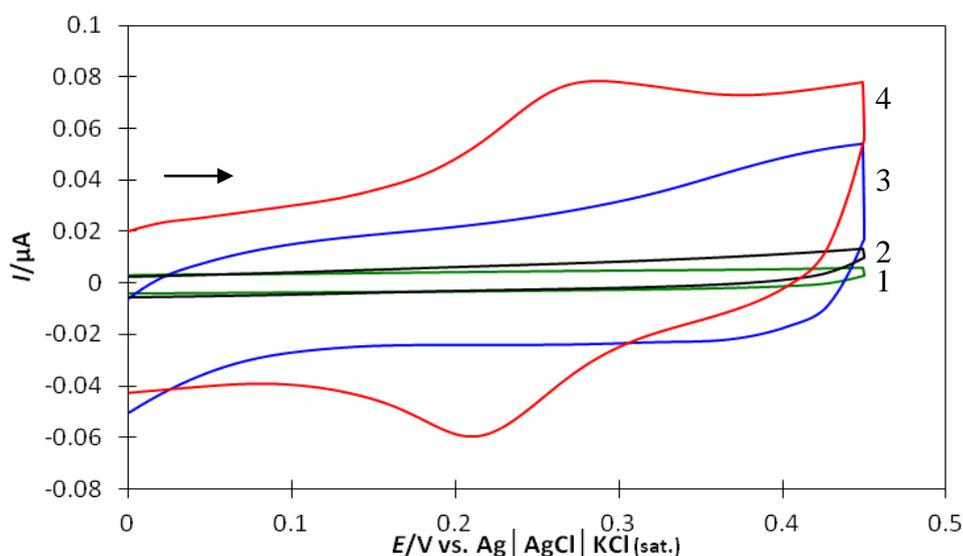
**Figure 3.** CVs obtained at bare AuE (1), ASOM-physically immobilized AuE (2), Apo-ASOM-immobilized AuE (3) and ASOM-immobilized AuE (4) in 5.0 mM PBS (pH 7.0) under  $\text{N}_2$  gas atmosphere.  $\nu = 10 \text{ mV/s}$ .
