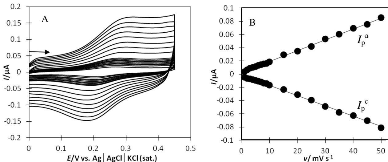
**Figure 4.** (A) CVs obtained for ASOM-immobilized AuE at different scan rates (1, 2, 3, 4, 5, 6, 7, 8, 9, 10, 15, 20, 25, 30, 35, 40, 45 and 50  $\text{mV/s}$  from inner to outer). (B) Plots of anodic and cathodic peak currents (background current-subtracted  $I_p^a$  and  $I_p^c$ , respectively) vs. scan rate (data were taken from Fig. 4A).
