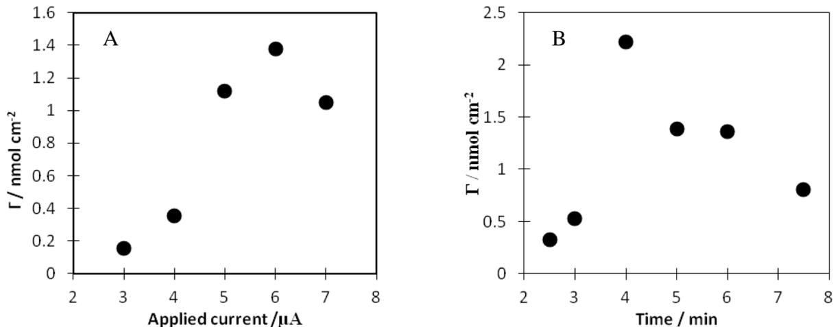
**Figure 2.** Surface coverage ( $\Gamma$ ) of ASOM immobilized on the AuE as a function of (A) the applied current at a constant electrolysis time (5 min) and (B) the electrolysis time at a constant current of  $6 \mu\text{A}$ .
