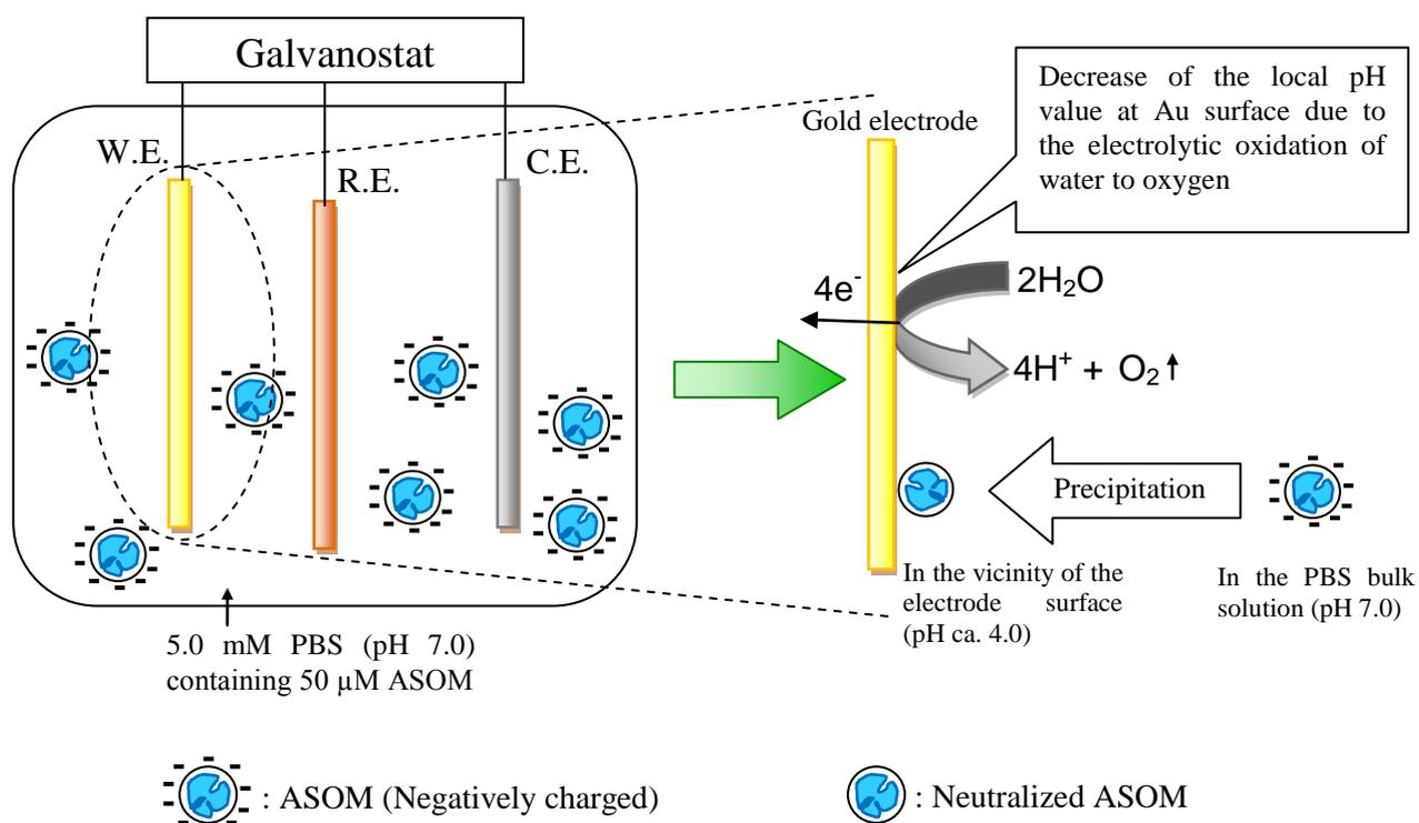
**Figure 1.** Schematic representation of galvanostatic immobilization of ASOM.
