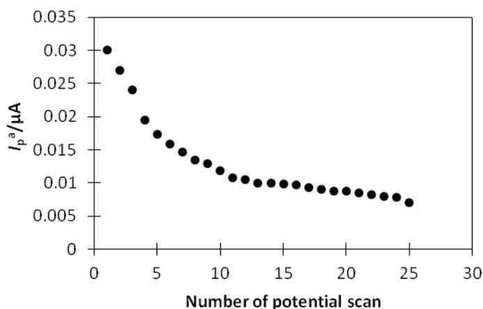
**Figure 5.** Plot of  $I_p^a$  vs. number of potential scan obtained at ASOM-immobilized AuE. Data were obtained by continuous potential cycling between 0 and 0.45 V in PBS(5.0 mM, pH 7.0) under  $\text{N}_2$  atmosphere.  $\nu = 10 \text{ mV/s}$ .
