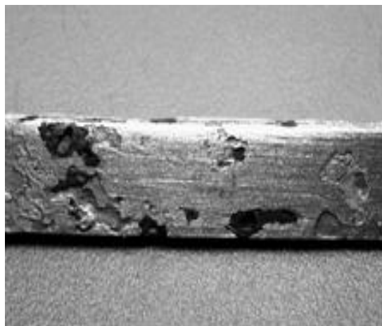
Figure 11. After 90 days of exposure for carbon steel in 1 % NaCl at a temperature of 35 °C.
