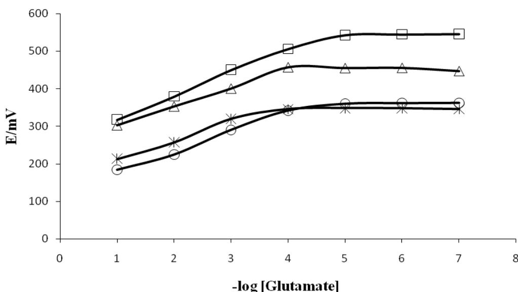
**Figure 3.** Potential response of glutamate membrane sensor based on [4](1)(2,3-Diazabuta-1,3-diene)ferrocenophane at different membrane composition. ( $\Delta$  : membrane No.1, \* : membrane No.2,  $\circ$  : membrane No.3,  $\square$  membrane No.4).
