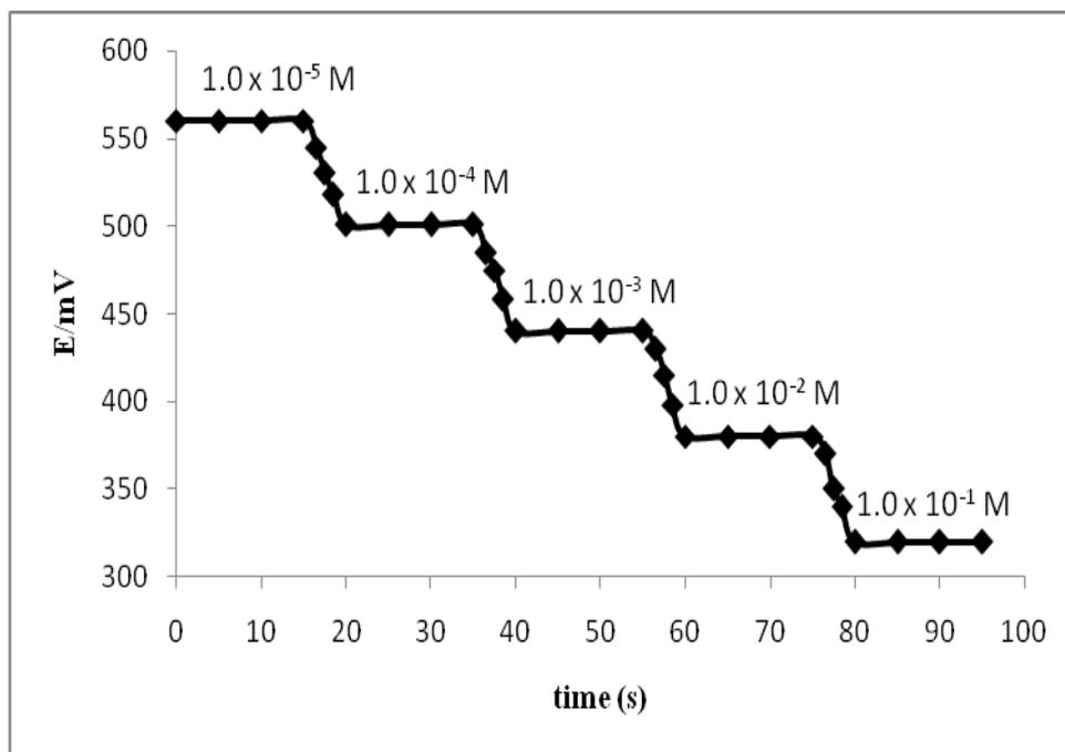
**Figure 4.** The dynamic response study of membrane electrode No. 4
