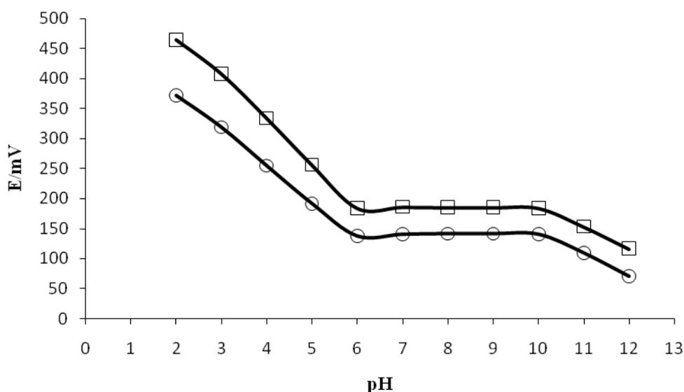
**Figure 5.** Effect of pH at (  $\square$  )  $1.0 \times 10^{-3}$  M and (  $\circ$  )  $1.0 \times 10^{-4}$  M glutamate solutions on the potential response of membrane No. 4.
