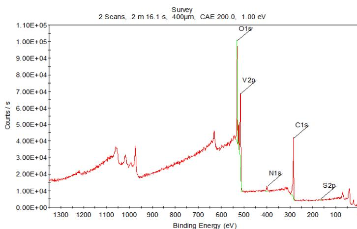
**Figure 6.** XPS survey spectra of carbon felt after 40 cycles
