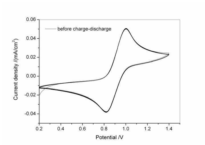
**Figure 1.** CV of the electrolyte (2.0M VOSO<sub>4</sub> + 3.0M H<sub>2</sub>SO<sub>4</sub>) with 3% Tri before charge-discharge.
