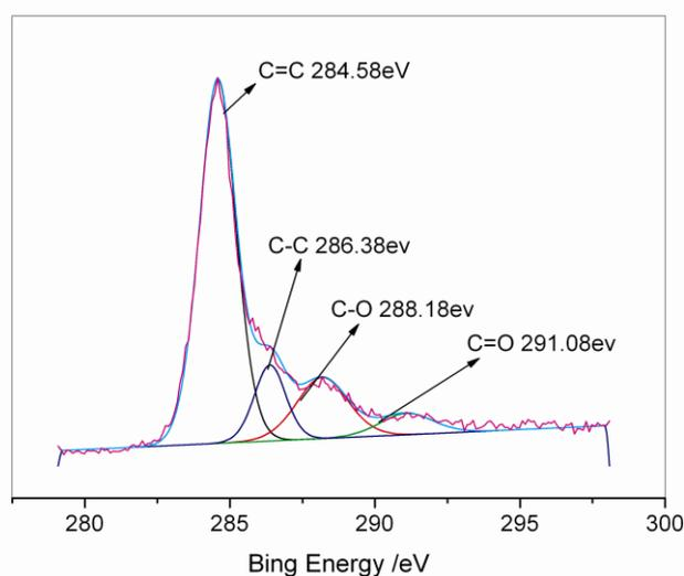
**Figure 7.** XPS C1s peaks of carbon felt after 40 cycles
