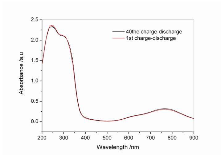
**Figure 5.** UV-vis spectra of electrolyte solutions with Tri additive.
