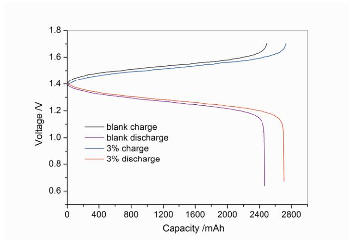
**Figure 3.** charge and discharge curves for blank sample and 3% Tri sample at 40 mA/cm<sup>2</sup>.
