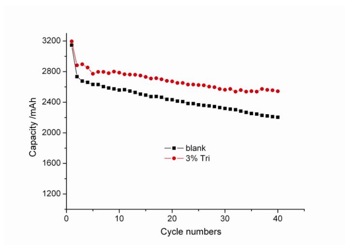
**Figure 4.** Decline discharge capacity of VRB at 40 mA/cm<sup>2</sup>.
