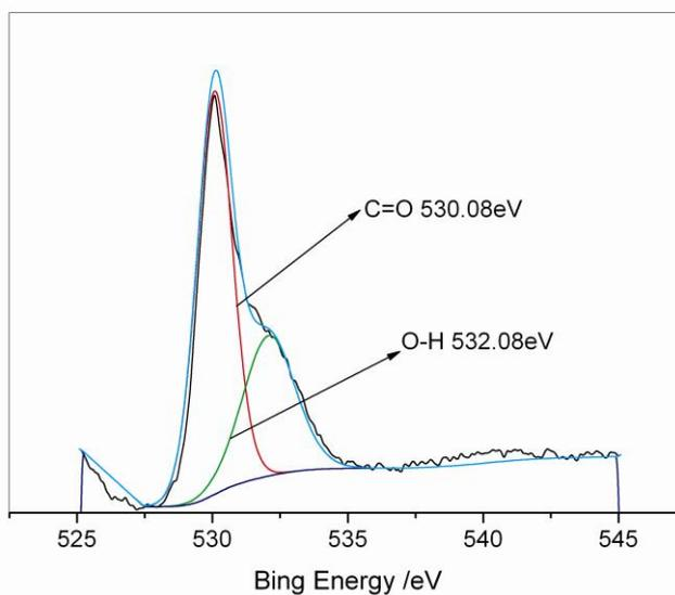
**Figure 8.** XPS O1s peaks of carbon felt after 40 cycles
