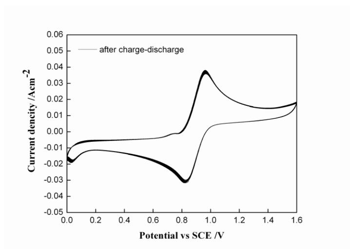
**Figure 2.** CV of the electrolyte (2.0M VOSO<sub>4</sub> + 3.0M H<sub>2</sub>SO<sub>4</sub>) with 3% Tri after charge-discharge.
