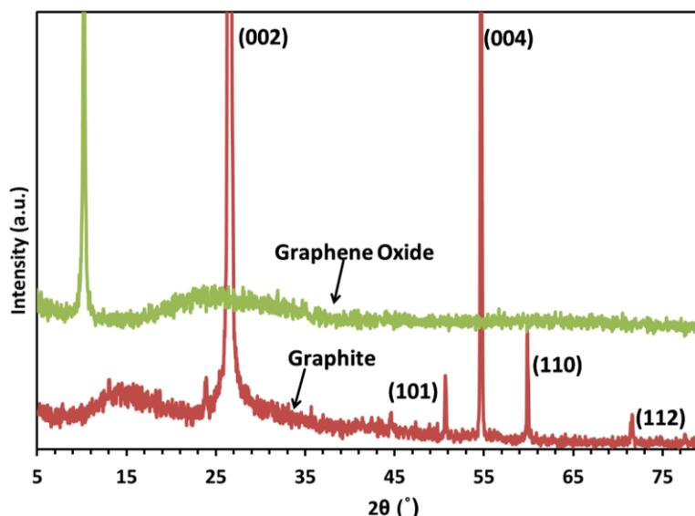
**Figure 3.** XRD patterns of graphite and graphene oxide.
