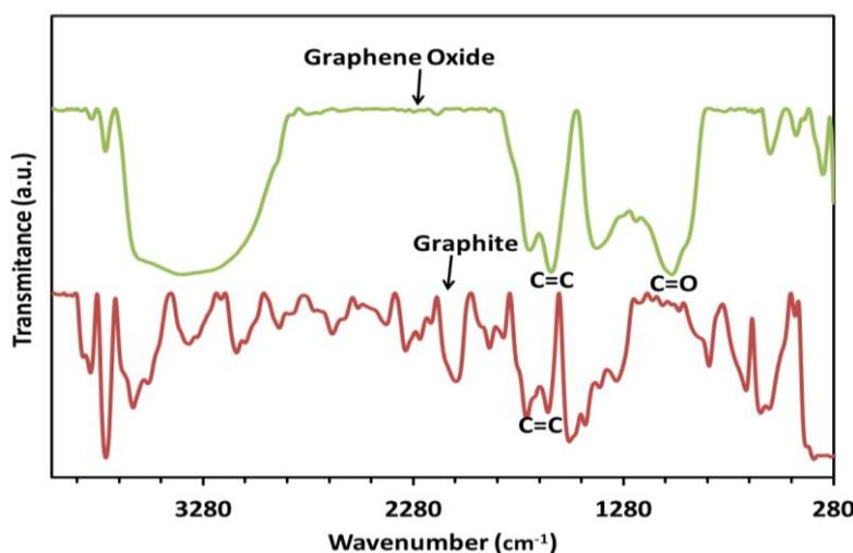
Figure 4. FTIR spectra of graphite and graphene oxide.
