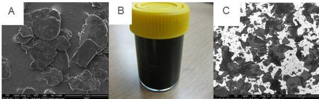
**Figure 2.** (A) FESEM image of graphite, (B) gel-like solution of graphene oxide and (C) FESEM image of graphene oxide.
