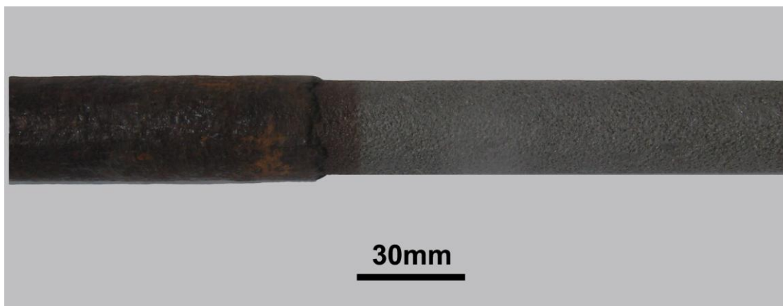
Figure 6. Morphology of bare surfaced rod after one year's exposure at splash zone, left is the upper half without removal of rust; right is the lower half, with rust removed.
