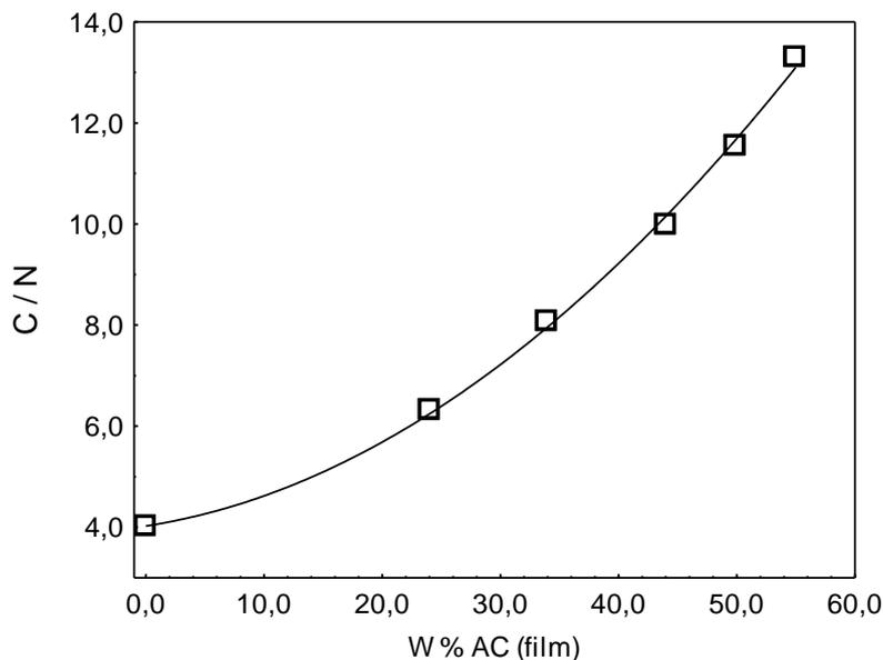
**Figure 1.** C/N dependence on weight percentage of AC in the PPy/AC - composite.
