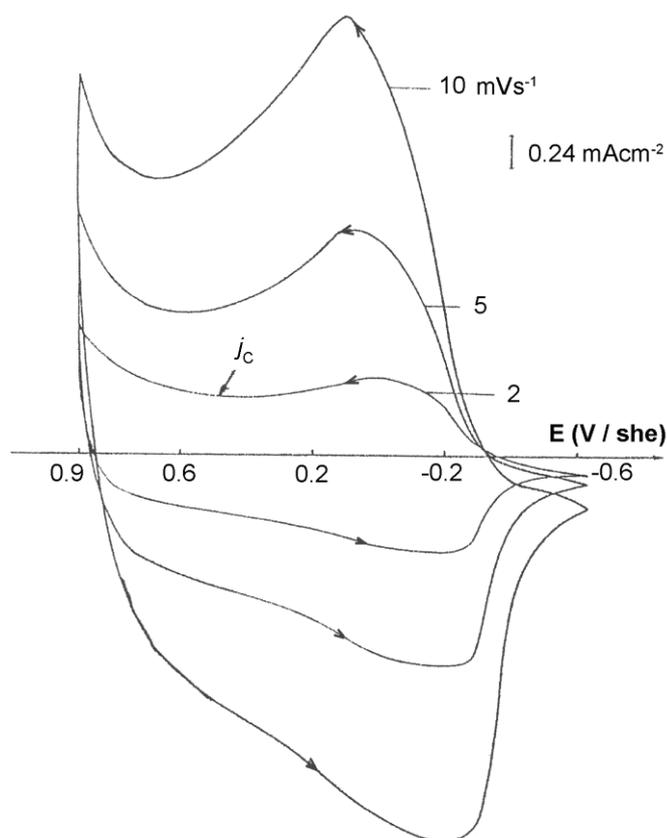
**Figure 2.** Voltammograms for PPy/AC composite film synthesized from 0.1 M Py in 0.5 M NaClO<sub>4</sub> / ACN with  $C_{AC} = 30 \text{ gL}^{-1}$ ;  $j = 1.5 \text{ mAcm}^{-2}$ ;  $Q_{\text{pol.}} = 1,8 \text{ Ccm}^{-2}$ .
