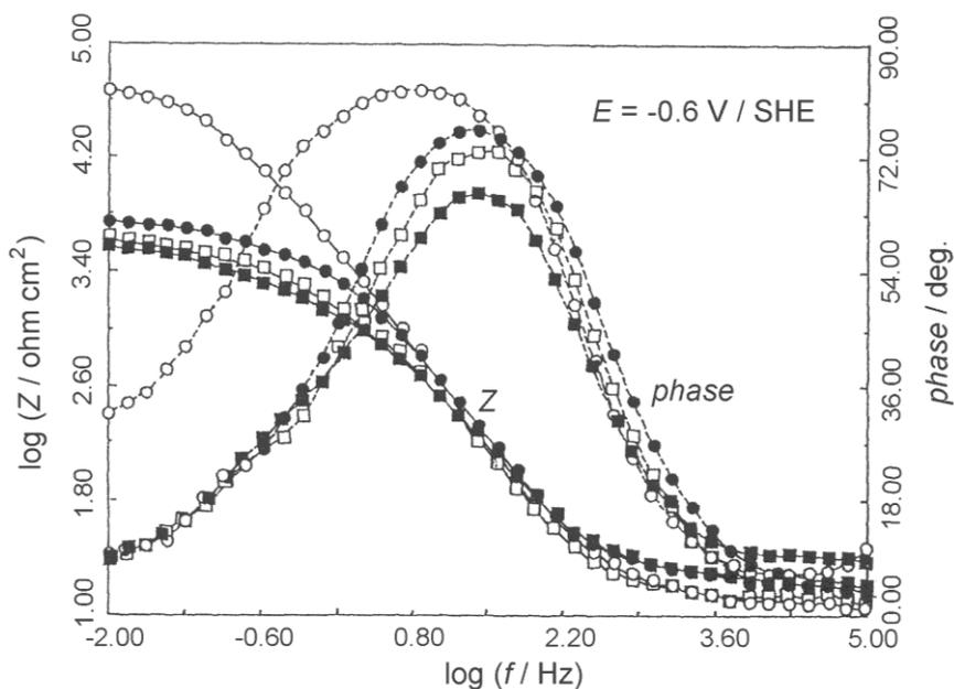
**Figure 7.** Bode plots for PPy – film (-o-) and PPy / AC composites ( $L_{PPy} = 5 \mu\text{m}$ ): (-●-) 10, (-□-) 20, and (-■-)  $50 \text{ gL}^{-1}$  AC in the  $0.5\text{M NaClO}_4 / \text{ACN}$  solution, for reduced (undoped) state.
