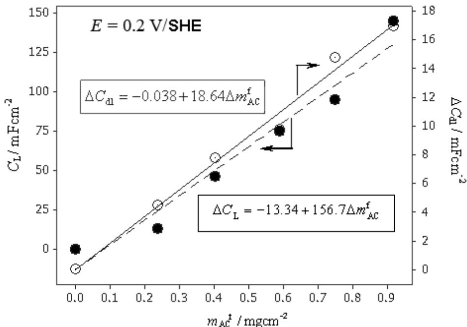
**Figure 11.** Impact of AC particles in the PPy – composite film ( $\text{mgcm}^{-2}$ ) on the limiting capacitance ( $C_L$ ) (-●-) and double layer capacitance ( $C_{dl}$ ) (-○-) – obtained by EIS (Table II).
