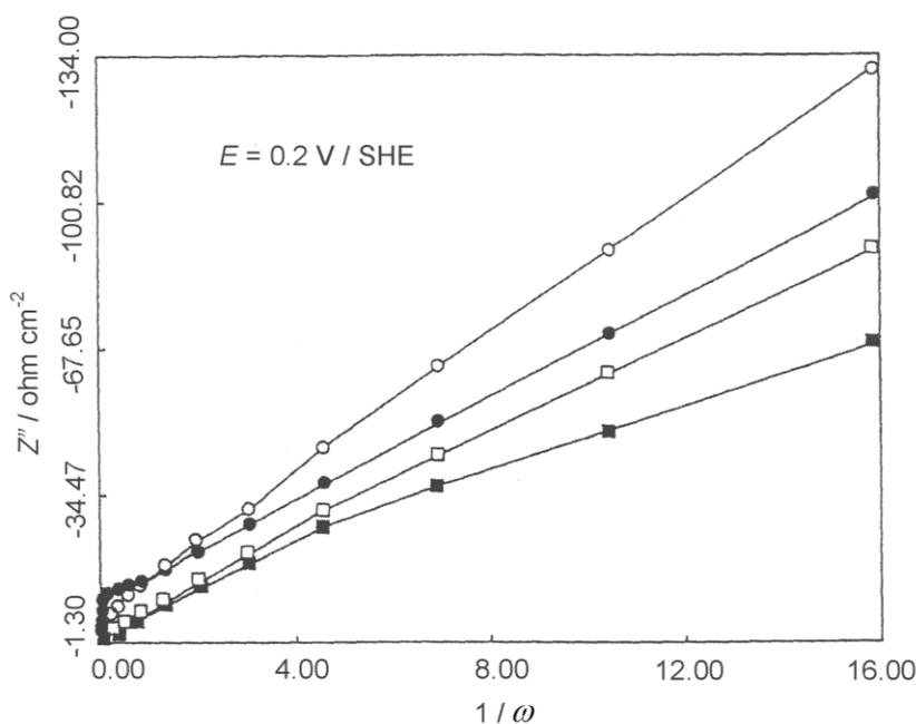
**Figure 5.**  $Z'' - 1/\omega$  plots for PPy (-○-) and PPy / AC composites (Table I): (-●-) 20, (-□-) 30, and (-■-) 50  $\text{gL}^{-1}$  AC in the 0.5M  $\text{NaClO}_4 / \text{ACN}$  solution; for oxidized (doped) state of PPy.
