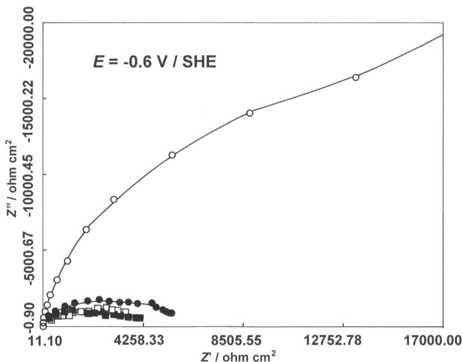
**Figure 10.** Nyquist plot for PPy – film (-o-) and PPy / AC composites ( $L_{\text{PPy}} = 5 \mu\text{m}$ ): (-●-) 10, (-□-) 20, and (-■-) 50  $\text{gL}^{-1}$  AC in the 0.5M  $\text{NaClO}_4$  / ACN solution, in reduced (undoped) state.
