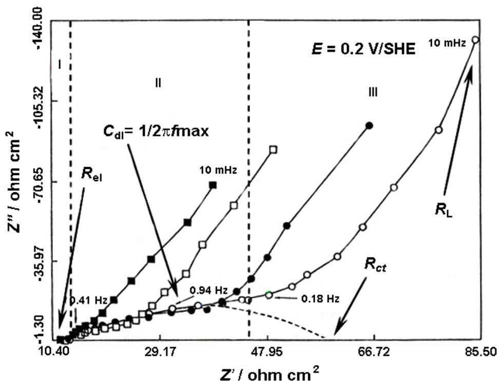
**Figure 9.** Nyquist plot for PPy / AC composites ( $L_{PPy} = 5 \mu\text{m}$ ): (-○-) 10, (-●-) 20, (-□-) 30, (-■-) 40  $\text{gL}^{-1}$  AC in 0.5M  $\text{NaClO}_4$  / ACN solution, in oxidized (doped) state.
