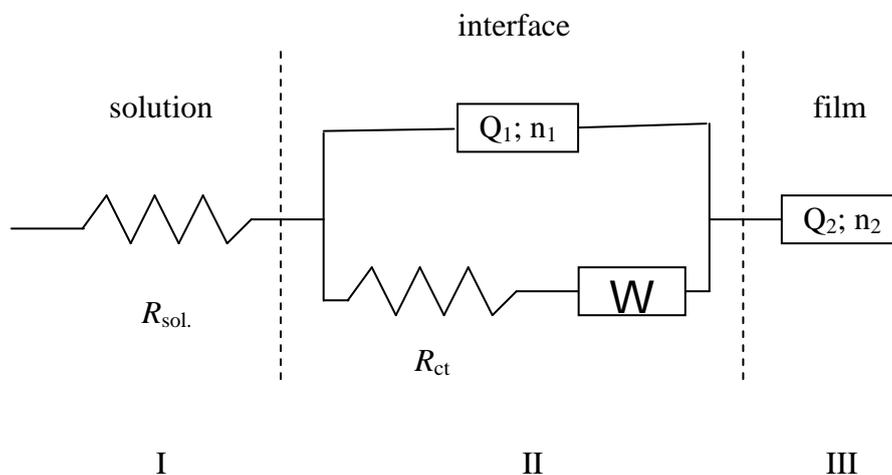
**Figure 6.** Equivalent electrical circuit (EEC), for doped state ( $0.2 \text{ V/SHE}$ ) of PPy and PPy / AC composite films.
