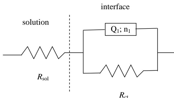
**Figure 8.** Equivalent electrical circuit (EEC), for undoped (-0.6 V/SHE) state of PPy and PPy / AC composite films.
