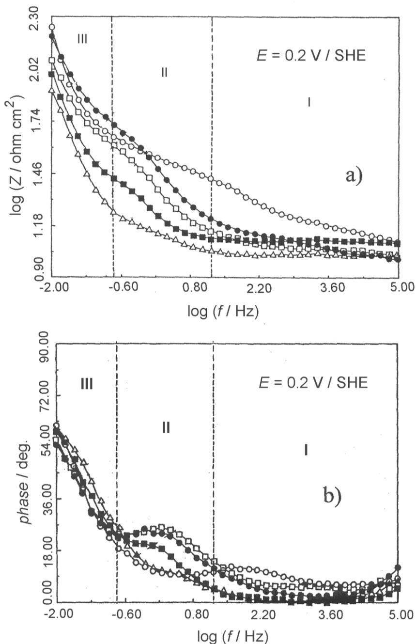
**Figure 4.** Bode plots of PPy – film (-○-) and PPy / AC composites (Table I): (-●-) 10, (-□-) 20, (-■-) 40, and (-△-) 50  $\text{gL}^{-1}$  AC in the 0.5M  $\text{NaClO}_4$  / ACN solution, for oxidized (doped) state (a)  $\log Z - \log f$ ; and (b) Phase –  $\log f$  dependences.
