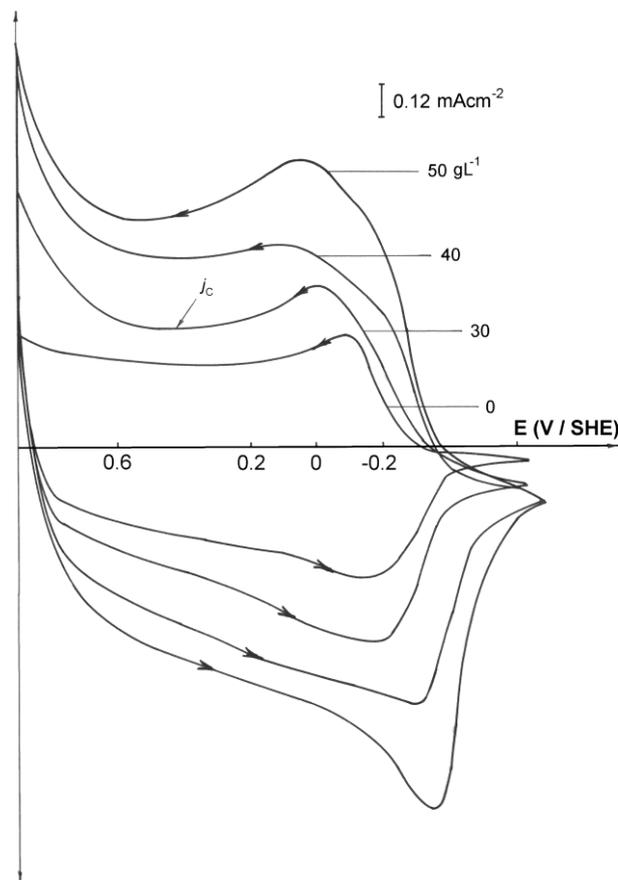
**Figure 3.** Voltammograms for PPY/AC composite film synthesized from 0.1 M Py in 0.5 M NaClO<sub>4</sub> / ACN with  $C_{AC} = 0, 30, 40, 50 \text{ gL}^{-1}$ ; sweep rate =  $2 \text{ mVs}^{-1}$ .
