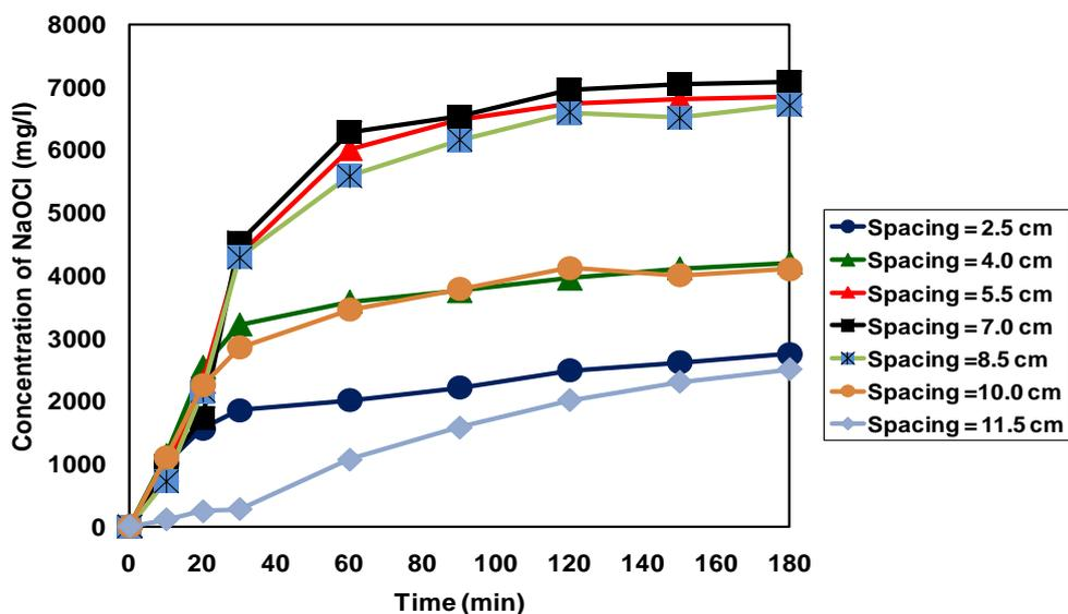
**Figure 5.** Effect of inter-electrode spacing on NaOCl production
