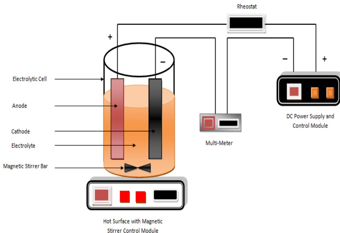
**Figure 1.** Schematic of sodium hypochlorite production electrochemical set-up (not to scale)
