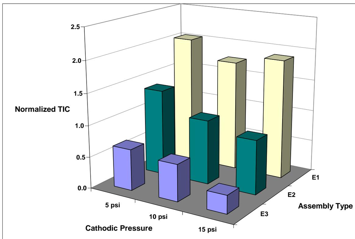
**Figure 5.** Normalized Total Investment Cost for PEMFC prototypes at pressure levels applied
