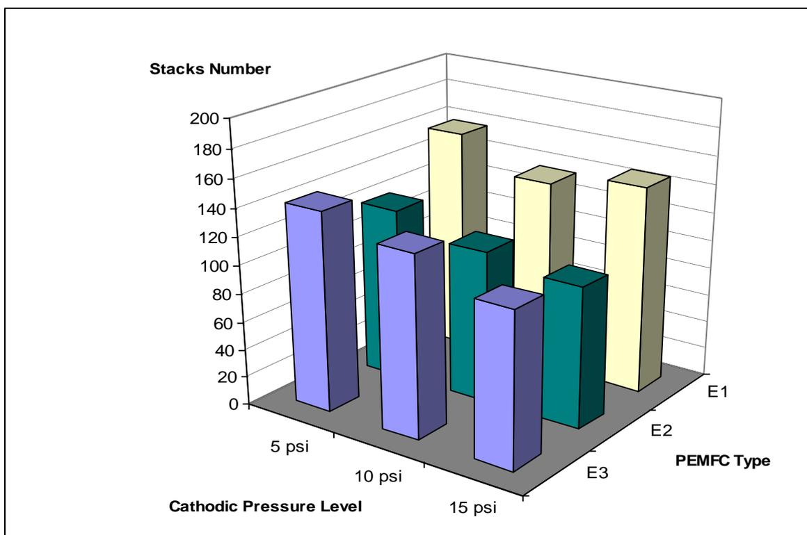
**Figure 4.** Stack number required by design for PEMFC prototypes
