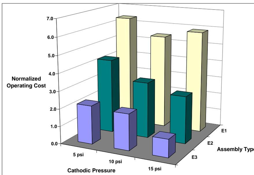
**Figure 6.** Normalized operating cost for PEMFC designs at experimental conditions
