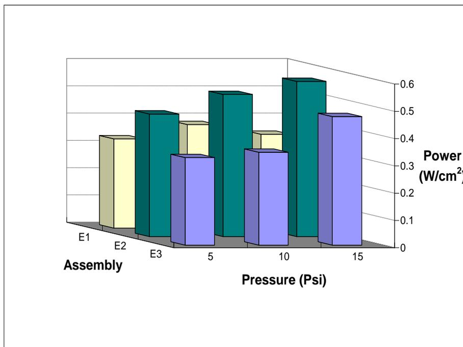
**Figure 1.** Power developed by PEMFC prototypes at different cathodic pressures.
