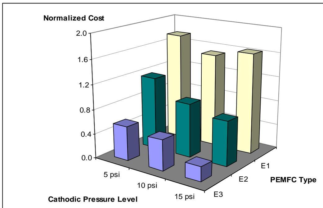
**Figure 2.** Normalized costs for the designed PEMFC stacks in a domestic stationary service at 140 kW-h and 120 V
