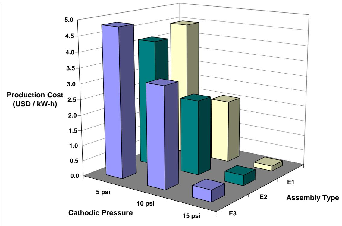
**Figure 7.** Unitary production cost for PEMFC designs at 20 years
