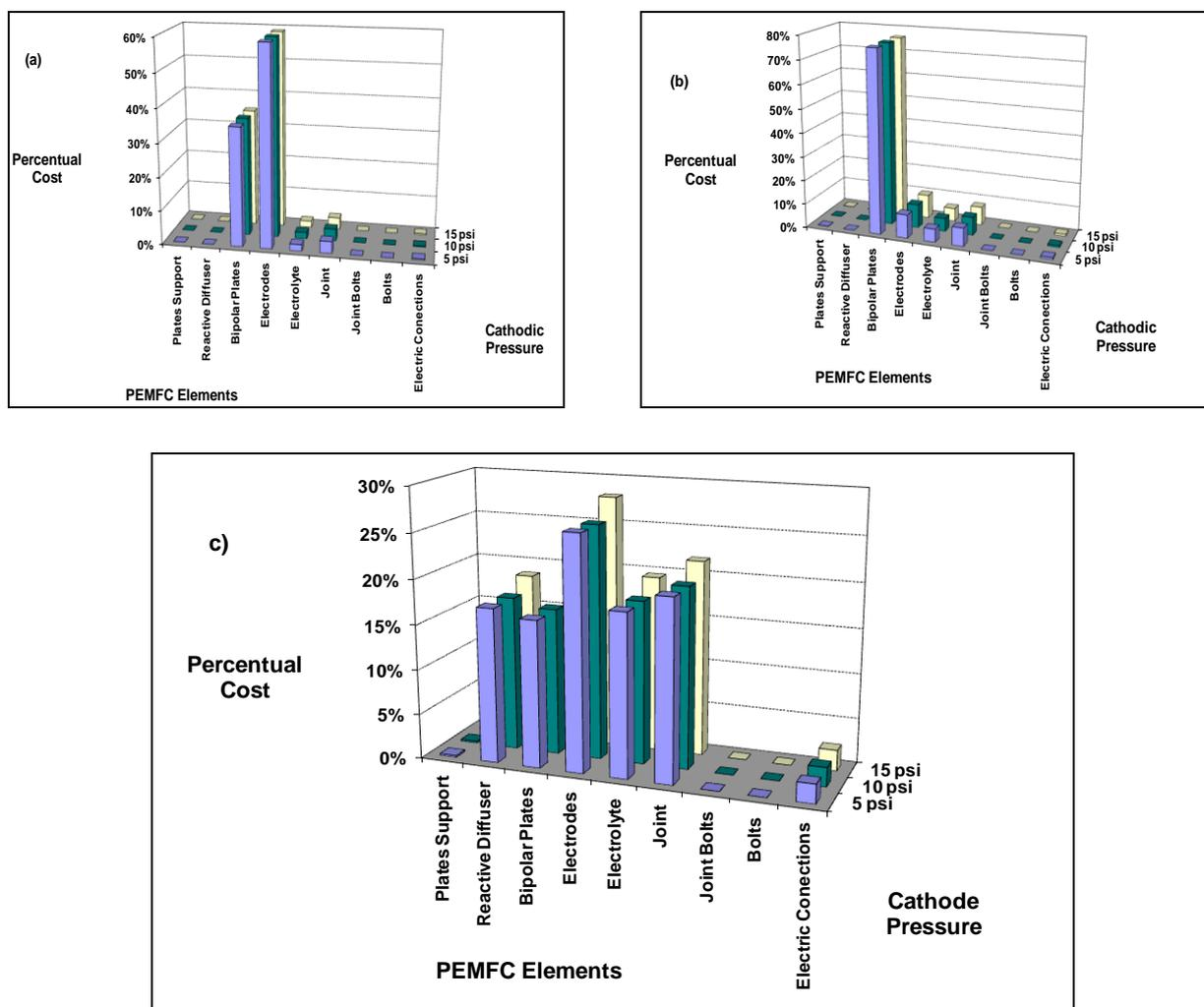
**Figure 3.** Percent costs for PEMFC elements: a) E1, b) E2, and c) E3 at experimental pressure conditions.
