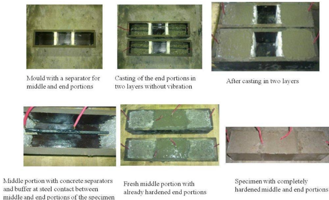
Figure 3. Experimental methodology for avoiding re-corrosion in repaired portion of chloride contaminated concrete.
