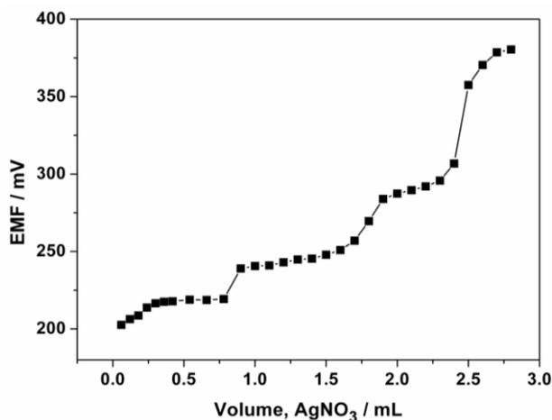
**Figure 3.** Titration curve of the 50 mL mixture of  $\text{Cl}^-$ ,  $\text{Br}^-$  and  $\text{I}^-$  with 0.1 M  $\text{AgNO}_3$  as titration reagent obtained by using  $\text{Ag}^+$ -ISE based on ionophore **L**. The concentration of each ion was  $2.0 \times 10^{-3}$  M.
