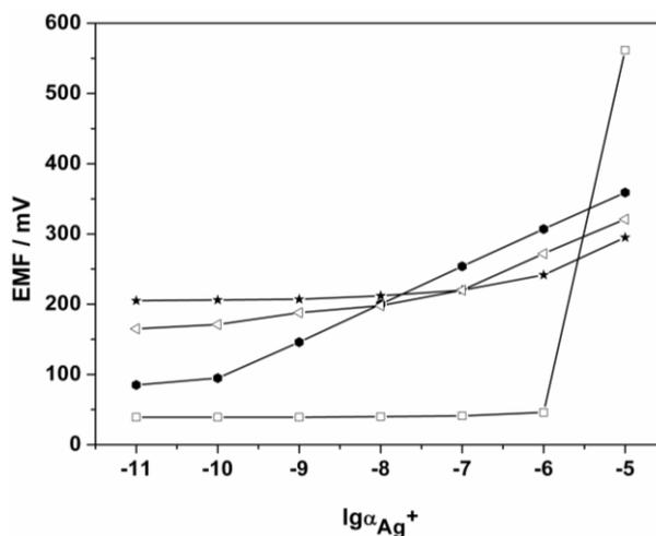
**Figure 1.** Electrodes based on ionophore **L** with different inner solutions: (□)  $1.0 \times 10^{-3}$  M NaCl, (★)  $1.0 \times 10^{-2}$  M NaCl with  $1.0 \times 10^{-5}$  M AgNO<sub>3</sub>, (▽)  $1.0 \times 10^{-3}$  M NaCl with  $1.0 \times 10^{-5}$  M AgNO<sub>3</sub>, and (●)  $1.0 \times 10^{-4}$  M NaCl with  $1.0 \times 10^{-5}$  M AgNO<sub>3</sub>.
