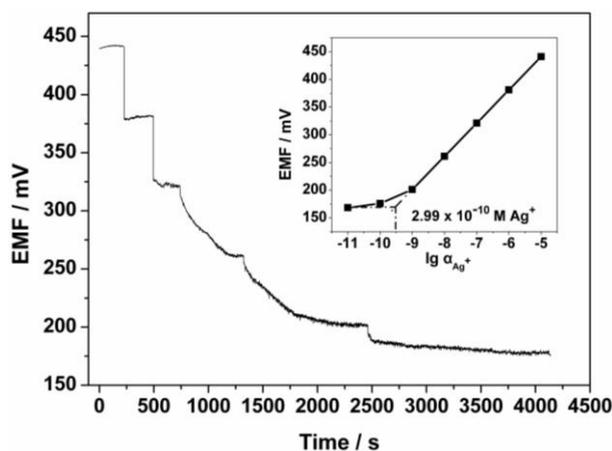
**Figure 2.** Potentiometric EMF response of the lower detection limit  $\text{Ag}^+$ -ISE based on **L**. Insert shows the working range.
