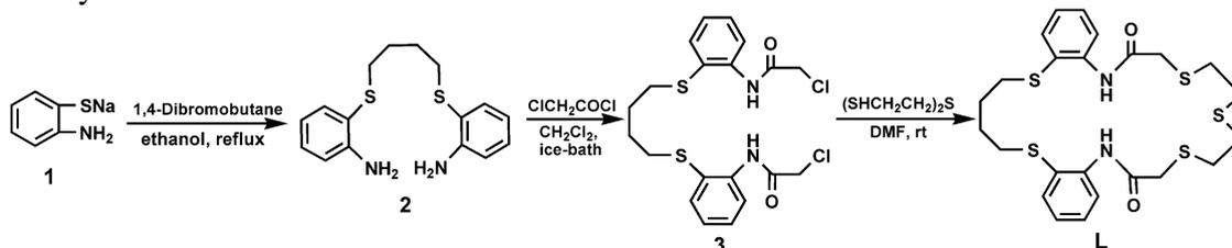
**Scheme 1.** Synthesis route of ionophore **L**.
