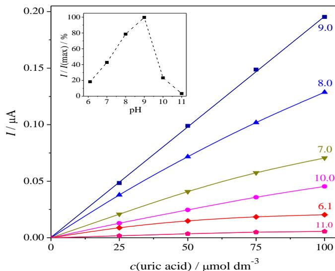
**Figure 3.** Dependence of the biosensor current on the concentration of uric acid at pH values of 6.1, 7.0, 8.0, 9.0, and 10.0. Inset: dependence of the biosensor sensitivity towards uric acid on pH (the sensitivities were normalized with respect to the maximum sensitivity observed at pH 9.0). Supporting electrolyte: 0.1 M Britton-Robinson buffer/0.1 M KCl; operating potential:  $-0.05$  V.
