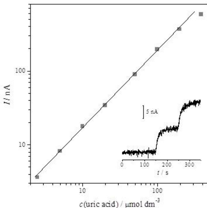
**Figure 4.** Calibration plot for uric acid measured with the uric acid biosensor. Inset: amperometric response of the biosensor upon two successive additions of  $5 \mu\text{M}$  of uric acid. Supporting electrolyte: 0.1 M Britton-Robinson buffer/0.1 M KCl, pH = 9.0; operating potential:  $-0.05$  V.
