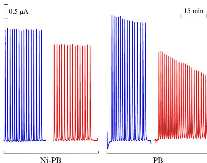
**Figure 2.** Diagrams recorded on  $\text{Ni}^{2+}$ -modified Prussian blue (Ni-PB) and unmodified Prussian blue (PB) upon the injections of 50  $\mu\text{L}$  of 250  $\mu\text{M}$   $\text{H}_2\text{O}_2$  into the carrier stream buffered to pH 7.0 (blue line) and 9.0 (red line). Carrier: 0.1 M Britton-Robinson buffer/0.1 M KCl; flow rate: 0.8 mL/min; operating potential:  $-0.05$  V.
