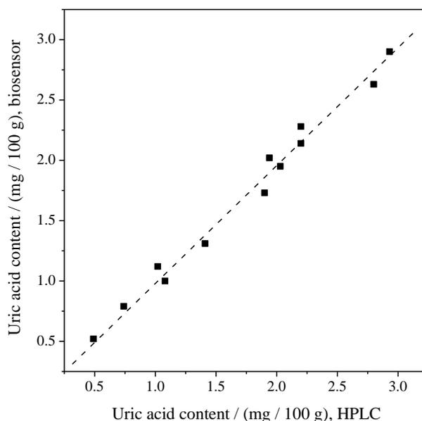
**Figure 6.** Correlation between the uric acid contents in commercial dairy products determined by the developed uric acid biosensor and the ion-exclusion HPLC method. The regression line is indicated by dashed trace.
