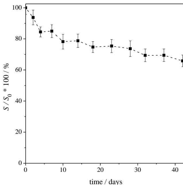
**Figure 5.** Long-term stability of the uric acid biosensor. The points represent the mean sensitivity towards uric acid of five biosensors, normalized with respect to the mean sensitivity of the biosensors measured on the first day of use. Error bars indicate the standard deviation of the measured sensitivities. Supporting electrolyte: 0.1 M Britton-Robinson buffer/0.1 M KCl, pH = 9.0; operating potential:  $-0.05$  V.
