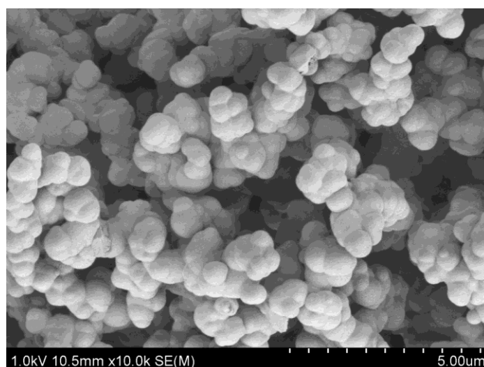
Figure 4. SEM image of PMCzP deposited on ITO electrode potentiostatically at 1.3 V.
