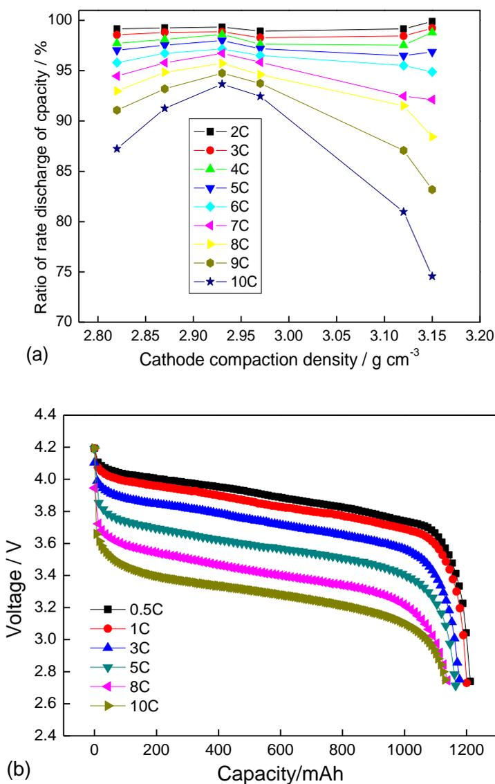
**Figure 1.** Relationship between rate discharge performance and compaction density of spinel LiMn<sub>2</sub>O<sub>4</sub> electrode in 18650 LiMn<sub>2</sub>O<sub>4</sub>/graphite high power batteries (a); rate discharge performance of 18650 spinel LiMn<sub>2</sub>O<sub>4</sub>/graphite power batteries at 25 °C (b).
