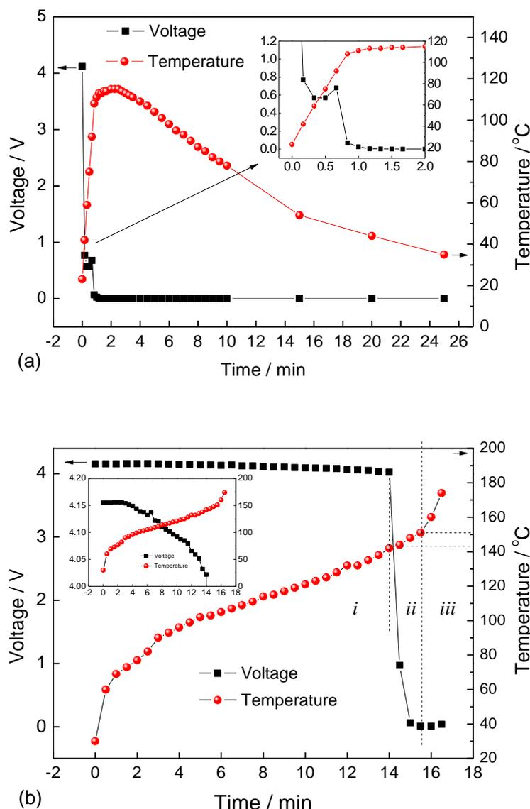
**Figure 6.** Voltage and temperature curves of fully charged 18650  $\text{LiMn}_2\text{O}_4$ /graphite high power batteries during short current (a) and oven test at 150 °C (b).
