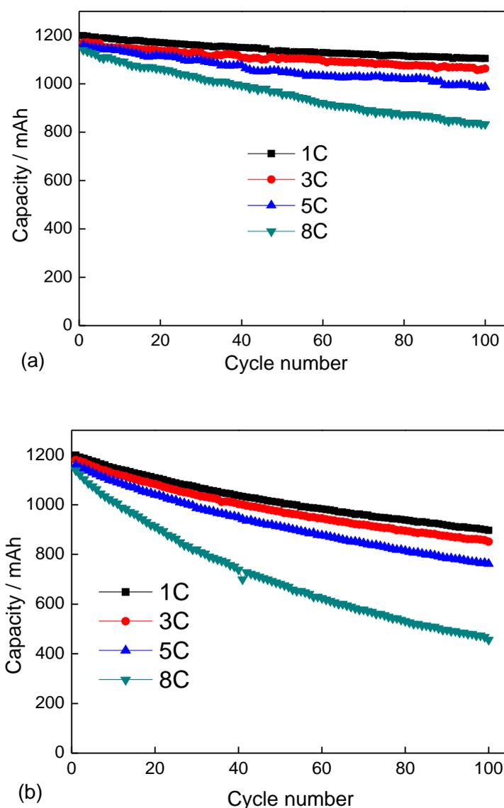
**Figure 2.** Cycling performance of 18650 spinel  $\text{LiMn}_2\text{O}_4$ /graphite power batteries with various discharge rates at 25 °C (a) and 55 °C (b).
