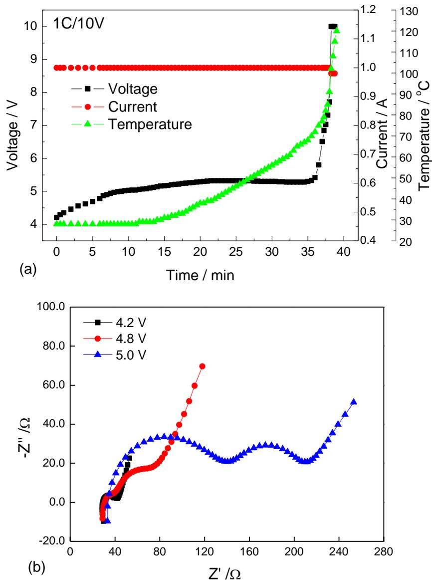
**Figure 5.** Voltage, current and temperature curves of 18650  $\text{LiMn}_2\text{O}_4$ /graphite high power batteries during 1 C/10 V overcharge test (a); EIS of power batteries before (4.2 V) and after overcharge(4.8 and 5.0 V) (b).
