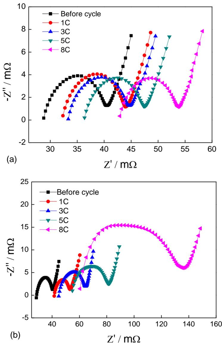
**Figure 4.** EIS of 18650 spinel  $\text{LiMn}_2\text{O}_4$ /graphite power batteries with 50% SOC, which were cycled 100 times with various discharge rates at 25 °C (a) and 55 °C (b).
