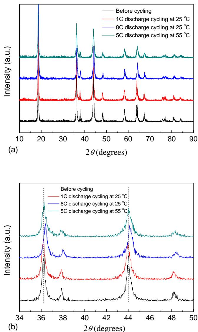
**Figure 3.** XRD patterns of  $\text{LiMn}_2\text{O}_4$  materials before and after 100 cycles at 25 °C and 55 °C within the  $2\theta$  angles range of 10~90° (a) and 34~50°(b).
