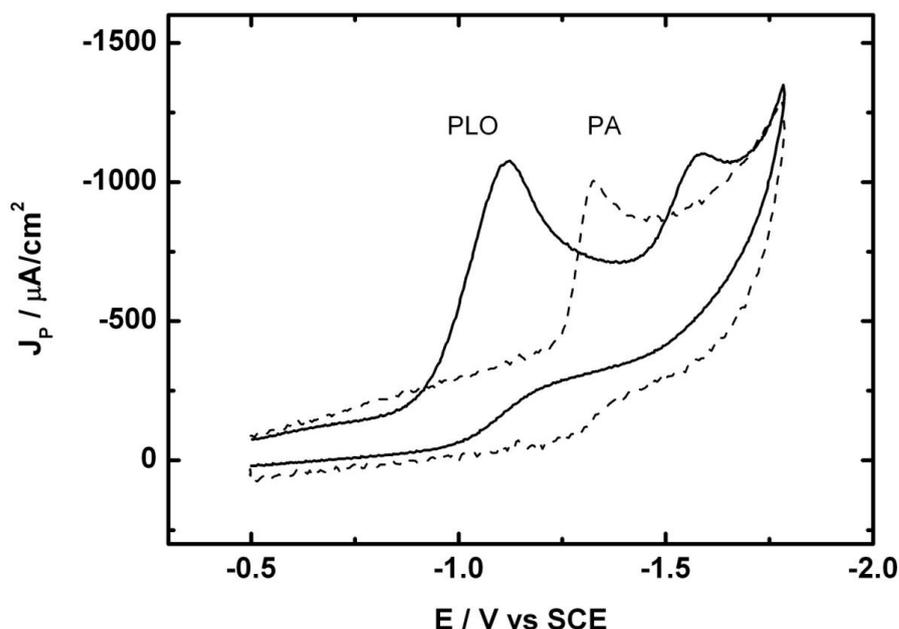
**Figure 1.** Cyclic Voltammety. Pyridoxal oxime (—) and pyridoxic acid (- - -).  $c=1\text{mM}$  and  $V=01.\text{V/s}$
