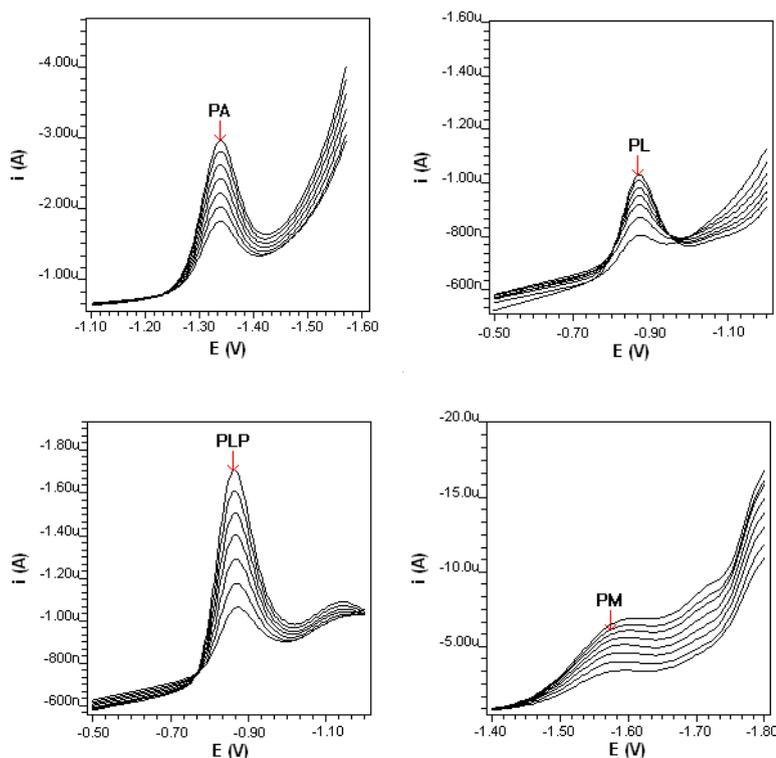
**Figure 2.** Cocentration study of the main B-6 vitamers using Diferential Pulse Voltammetry: (a) PA (b) PL (c) PLP and (d) PM
