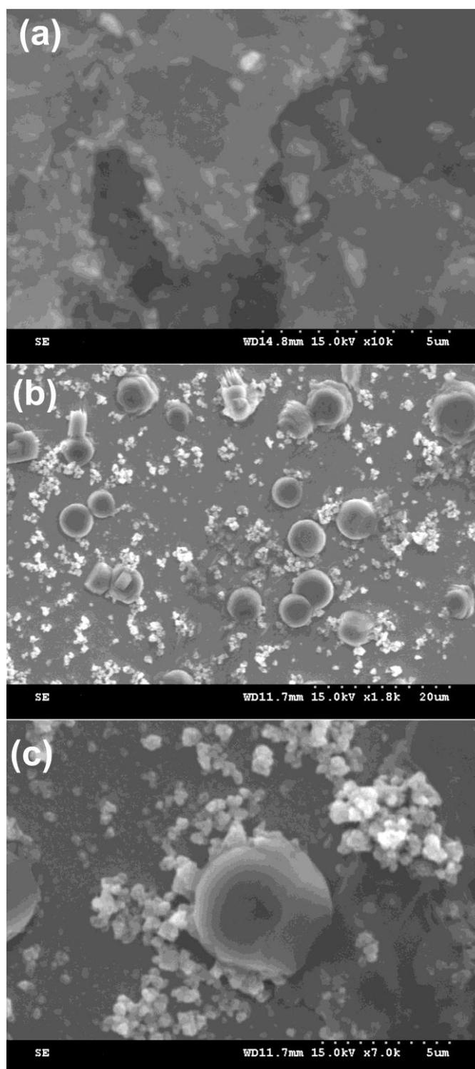
**Figure 3.** SEM images of (a) PEDOT, (b) nano TiO<sub>2</sub>-PEDOT (lower magnification) and (c) nano TiO<sub>2</sub>-PEDOT (higher magnification) modified ITO.
