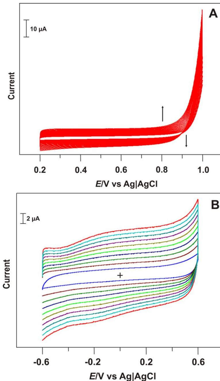
**Figure 1.** (A) Continuous CVs of PEDOT film growth on the nano TiO<sub>2</sub> particles modified GCE in pH 1.5 H<sub>2</sub>SO<sub>4</sub> solution containing 0.01 M EDOT in the potential scan between 0.2 to 1 for twenty cycles at the scan rate of 0.1 V/s. (B) Different scan studies of the nano TiO<sub>2</sub>-PEDOT film modified GCE in pH 7 PBS solution at the scan rate of 0.01 to 0.1 V/s.
