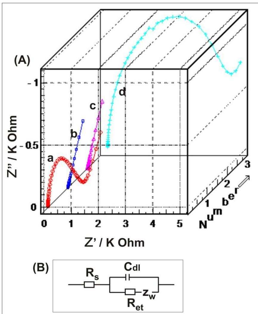
**Figure 2.** (A) EIS three dimensional view of (a) bare, (b) nano  $\text{TiO}_2$ -PEDOT film, (c) PEDOT film and (d) nano  $\text{TiO}_2$  modified GCE in pH 7.0 PBS containing 5 mM  $[\text{Fe}(\text{CN})_6]^{3-/4-}$ . (B) Randles equivalent circuit model for the proposed films.
