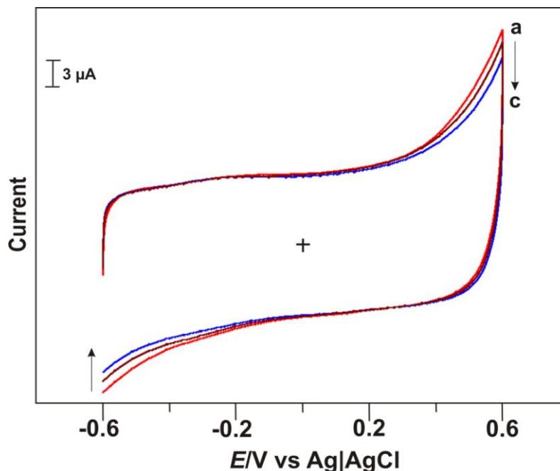
**Figure 7.** CV response of nano TiO<sub>2</sub>-PEDOT film modified GCE in the pH 7 PBS: (a) at the initial stage, (b) after 6 hours, and (c) second day.
