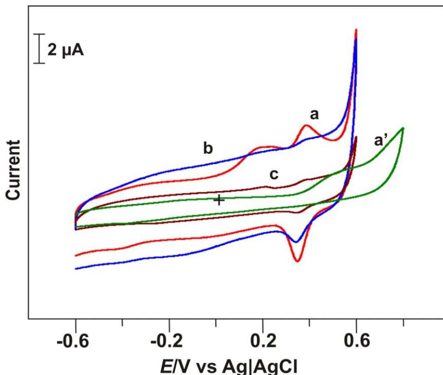
**Figure 4.** CV response in pH 7 PBS at (a) nano TiO<sub>2</sub>-PEDOT film, (b) PEDOT film, (c) nano TiO<sub>2</sub> particles modified and, (a') Bare GCE for the simultaneous detection of AA and diclofenac (AA and diclofenac concentration was  $4.2 \times 10^{-5}$  M).
