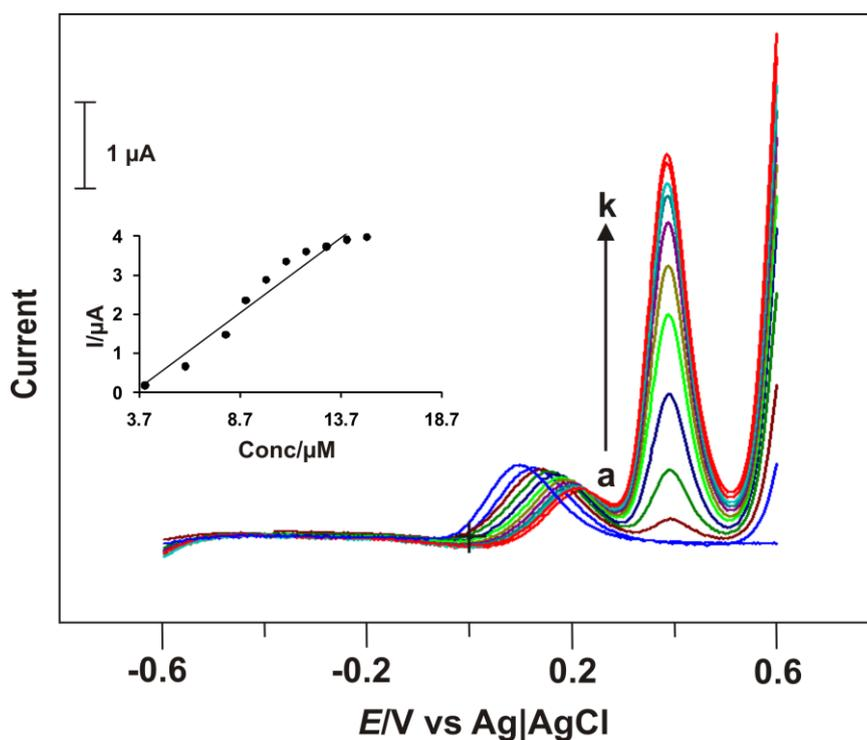
**Figure 6.** DPV response of nano TiO<sub>2</sub>-PEDOT film modified GCE for the selective detection of AA and diclofenac. In the DPV curve a denotes the electrooxidation signal of AA (40  $\mu\text{M}$ ) and curve b-k shows the DPV responses for the detection of diclofenac in the range of 4, 6, 8, 9, 10, 11, 12, 13, 14 and 15  $\mu\text{M}$  in the presence of AA (40  $\mu\text{M}$ ).
