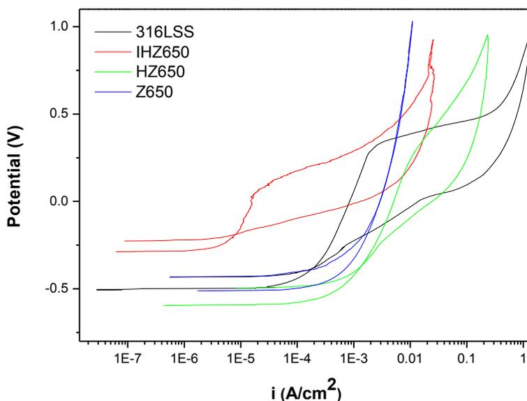
**Figure 1.** Cyclic polarization plots of 316L, Z650, HZ650 and IHZ650 samples.
