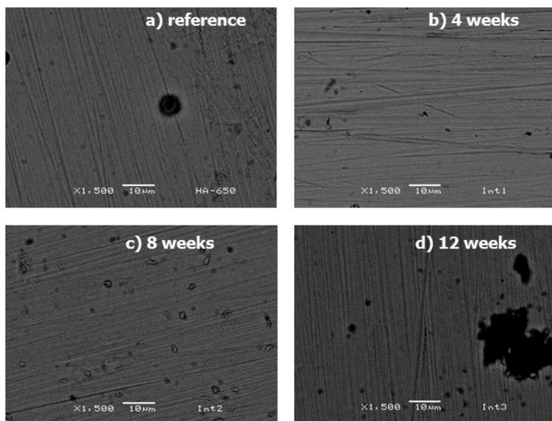
**Figure 6.** SEM images of IHZ650 sample tested in Ringer solution during a) zero weeks as a reference, b) 4 weeks, c) 8 weeks and d) 12 weeks.
