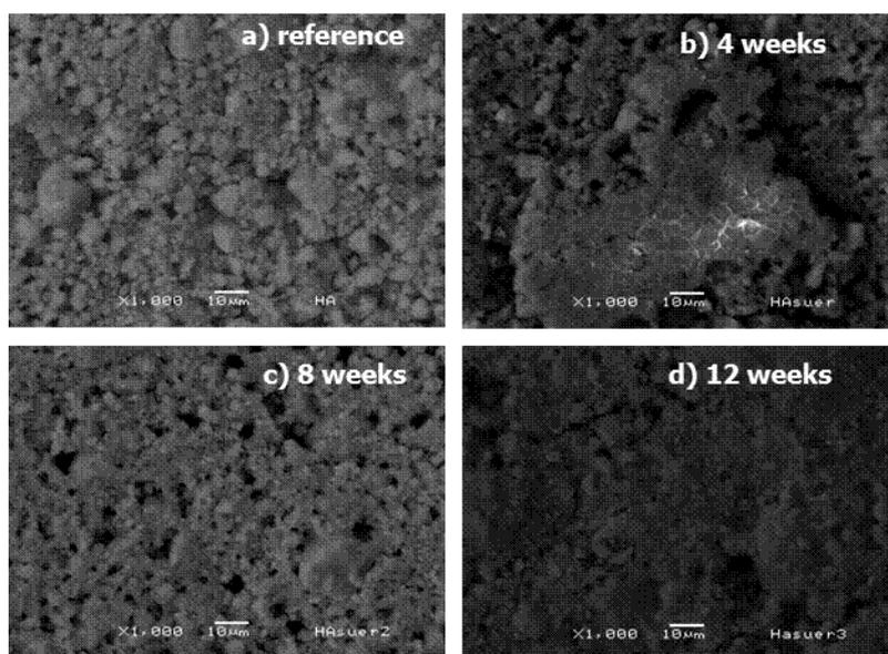
**Figure 5.** SEM images of HZ650 sample tested in Ringer solution during a) zero weeks as a reference, b) 4 weeks, c) 8 weeks and d) 12 weeks.
