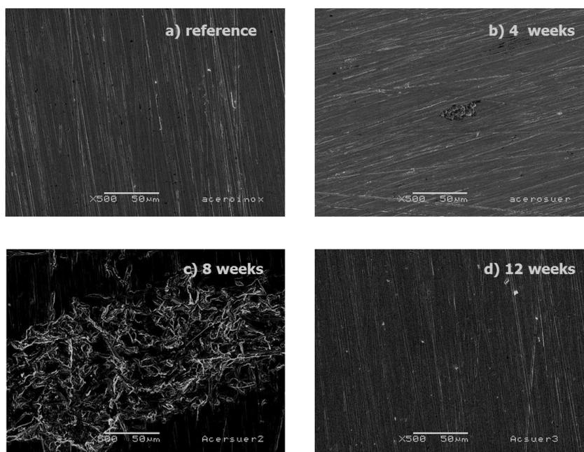
**Figure 3.** SEM images of 316LSS substrates tested in Ringer solution during a) zero weeks as a reference, b) 4 weeks, c) 8 weeks and d) 12 weeks.
