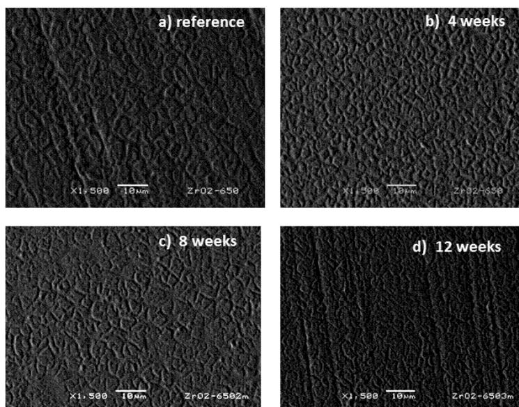
**Figure 4.** SEM images of Z650 sample tested in Ringer solution during a) zero weeks as a reference, b) 4 weeks, c) 8 weeks and d) 12 weeks.
