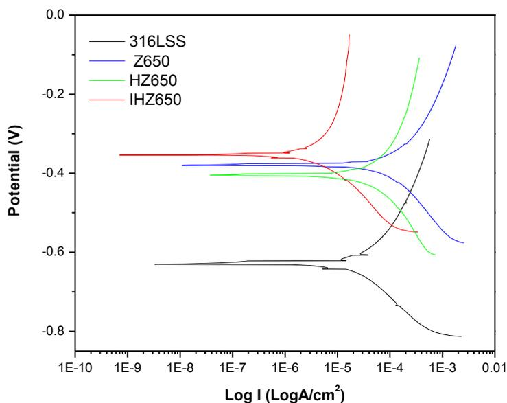
**Figure 2.** Tafel extrapolation plots of 316LSS, Z650, HZ650 and IHZ650 samples.
