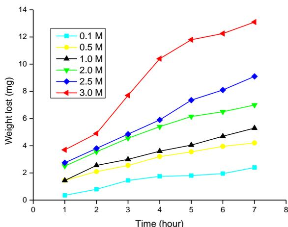
**Figure 1.** Weight loss of aluminum sheet in different concentrations of HCl for 7 hours
