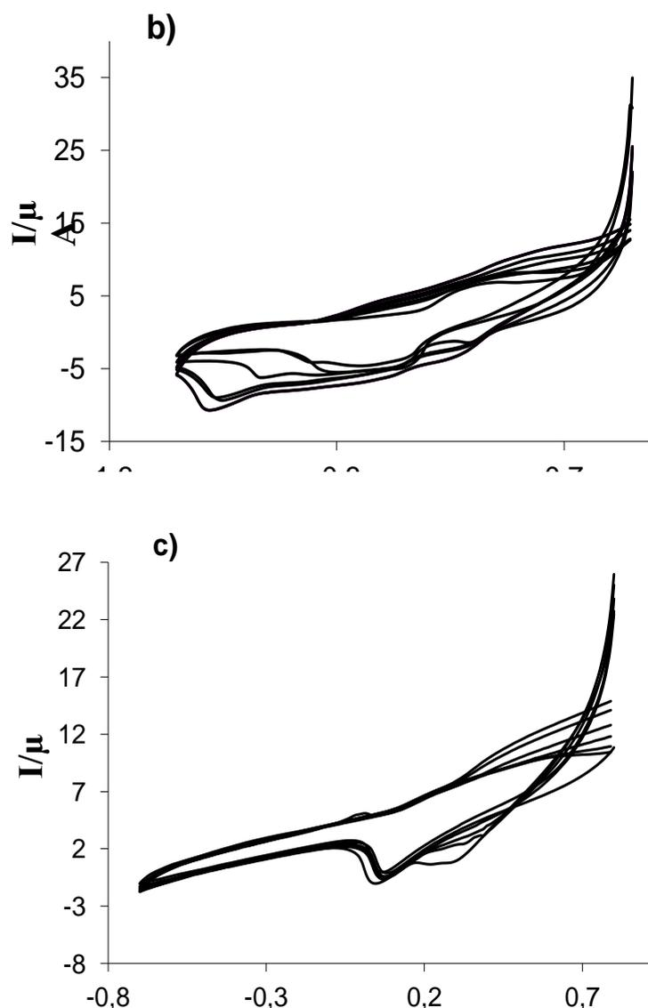
**Figure 1.** Voltammograms of CPE containing  $0.01 \text{ mol dm}^{-3}$  Fc solution in a) [OMIM]BF<sub>4</sub> b) [Bpy]BF<sub>4</sub> c) [HMIM]BF<sub>4</sub>, immersed in  $0.1 \text{ mol dm}^{-3}$  aqueous KClO<sub>4</sub>. The 1st, 2nd, 4th, 7th, 8th and 10th scan are shown. The arrow indicates the increasing number of scans; scan rate  $10 \text{ mV s}^{-1}$ .
