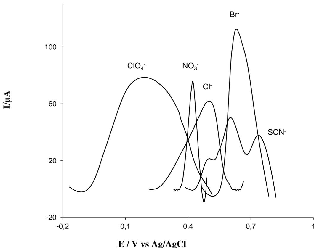
**Figure 3.** SW voltammetric responses ( frequency 10 Hz, amplitude 50 mV and scan increment 1 mV) of MWCNT modified CPE containing  $0.01 \text{ mol dm}^{-3}$  Fc immersed in different anion solutions.
