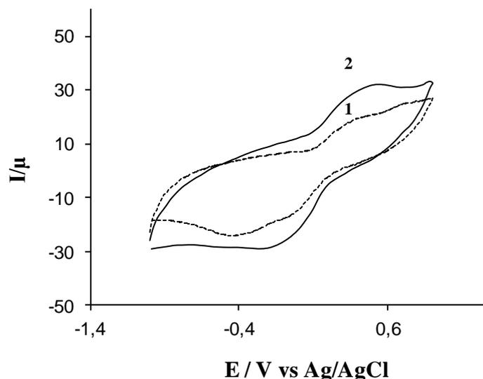
**Figure 2.** CVs of 2nd, 4th, 6th, 8th and 10th scan of CPE containing  $0.01 \text{ mol dm}^{-3}$  solution of Fc in [OMIM]BF<sub>4</sub> in absence (---) and present (—) of MWCNT, the CPE immersed in  $0.1 \text{ mol dm}^{-3}$  aqueous solution of KClO<sub>4</sub>. Scan rate is  $10 \text{ mV s}^{-1}$ .
