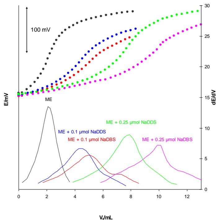
**Figure 4.** Titration curves of model effluent (ME, diluted solution of NaDBS-based powder detergent) and the corresponding first derivatives with the addition of known concentrations of NaDBS and NaDDS, using the DMI-TPB surfactant sensor as the indicator and DMIC ( $c = 5 \times 10^{-5}$  M) as the titrant.
