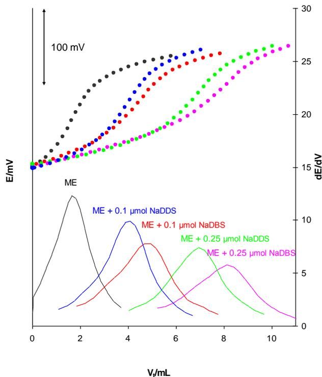
**Figure 5.** Titration curves of model effluent (ME, diluted solution of NaDBS-based powder detergent) and the corresponding first derivatives with the addition of known concentrations of NaDBS and NaDDS, using the DMI-TPB surfactant sensor as the indicator and CPC ( $c = 5 \times 10^{-5}$  M) as the titrant.
