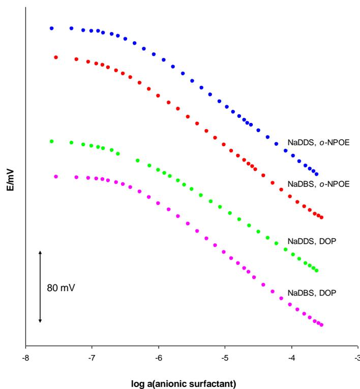
**Figure 1.** Influence of the plasticizer type on the response characteristics of the DMI-TPB sensor toward NaDBS and NaDDS. Here and in the following figures, some curves are displaced laterally or vertically for clarity.
