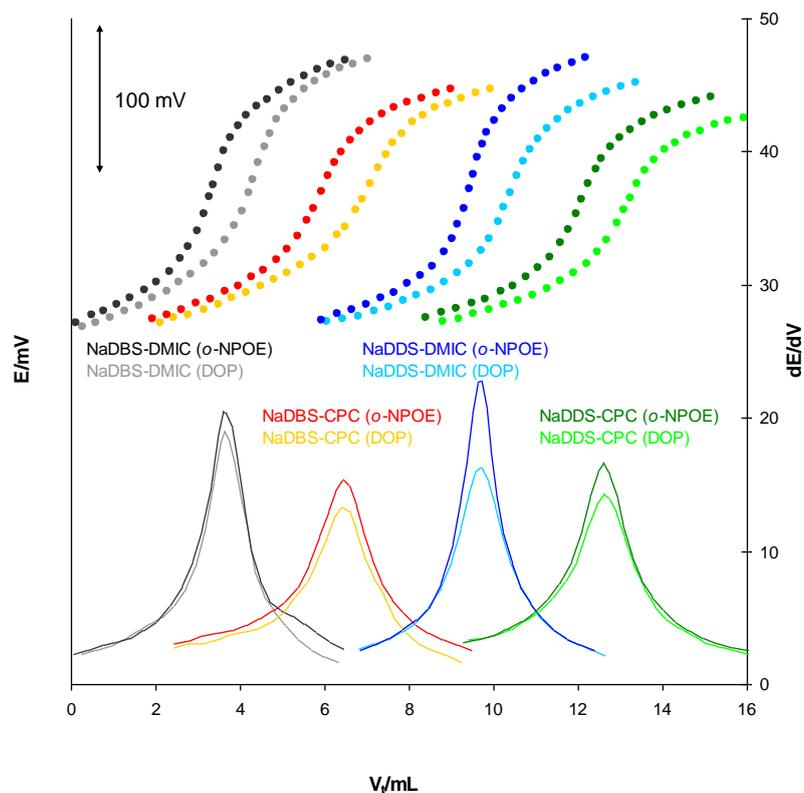
**Figure 2.** Potentiometric titration curves and their derivatives of NaDBS and NaDDS obtained with DMI-TPB sensors containing different plasticizers (DOP and *o*-NPOE) and DMIC and CPC as the titrants at concentrations of  $1 \times 10^{-4}$  M.
