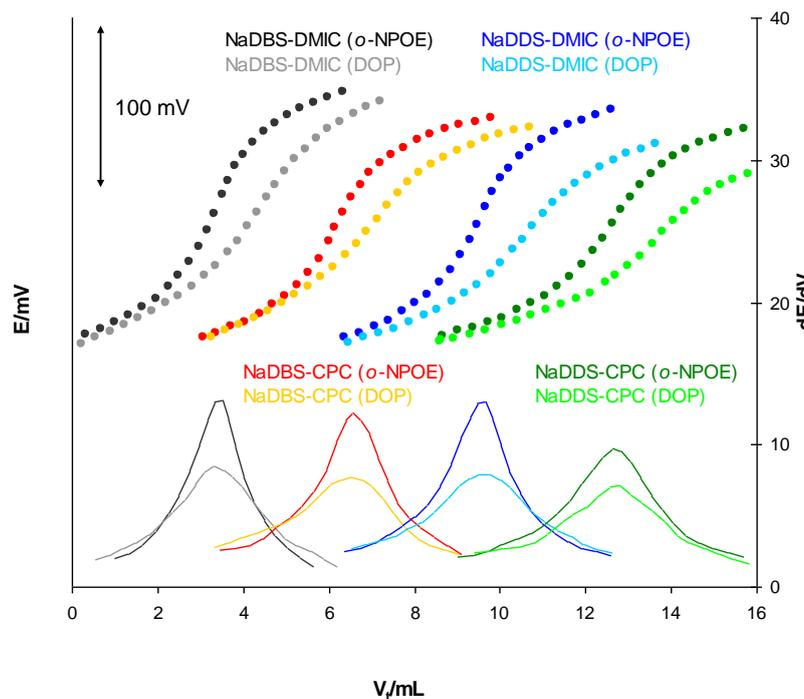
**Figure 3.** Potentiometric titration curves and their derivatives of NaDBS and NaDDS obtained with DMI-TPB sensors containing different plasticizers (DOP and *o*-NPOE) and DMIC and CPC as the titrants at concentrations of  $5 \times 10^{-5}$  M.
