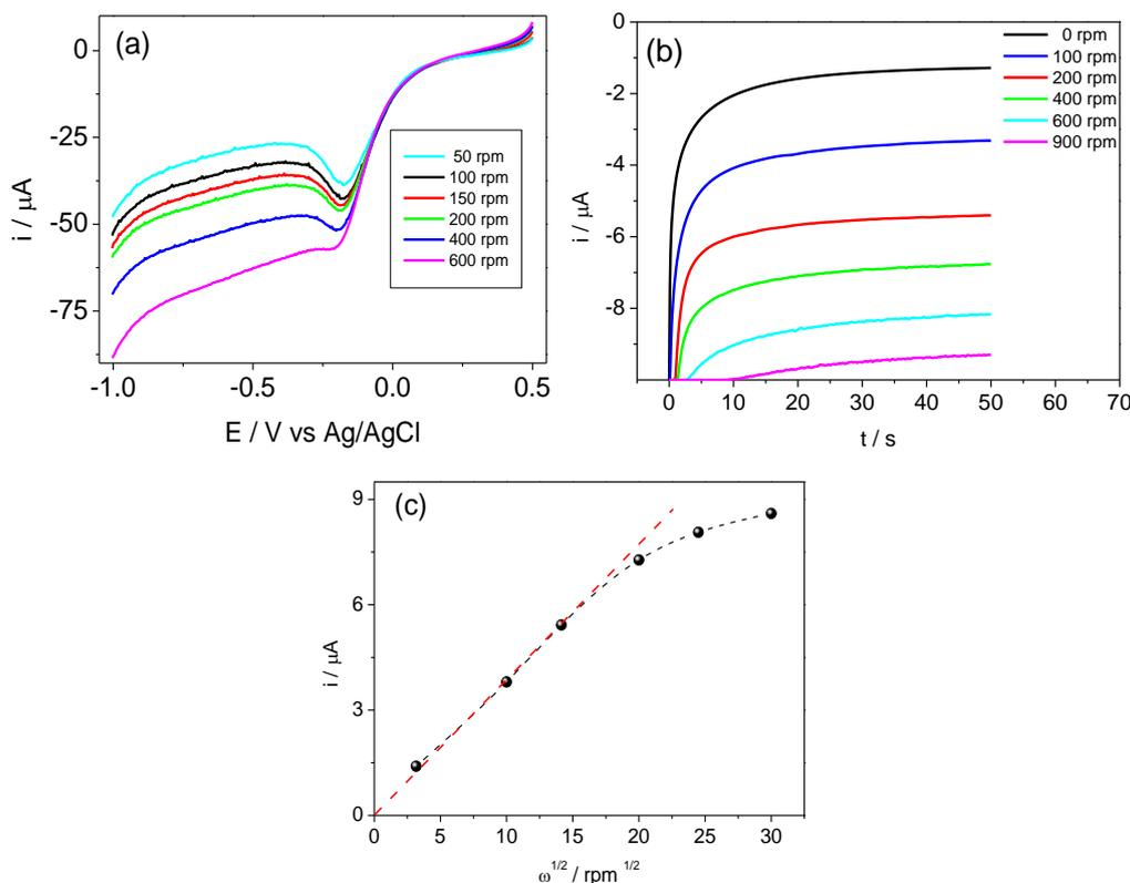
**Figure 1.** (a) Linear sweep voltammograms for glassy carbon electrode modified with HRP/MWCNT in  $50\mu\text{molL}^{-1}$  of  $\text{H}_2\text{O}_2$  at various rotation rates of the electrode and (b) Hydrodynamic amperometry for a glassy carbon electrode modified with HRP/MWCNT in  $10\mu\text{molL}^{-1}$  of  $\text{H}_2\text{O}_2$  at various rotation rates of the electrode. Applied potential,  $-0.25\text{ V/ Ag/AgCl}$ . (c) Levich Plot from plots in (b).
