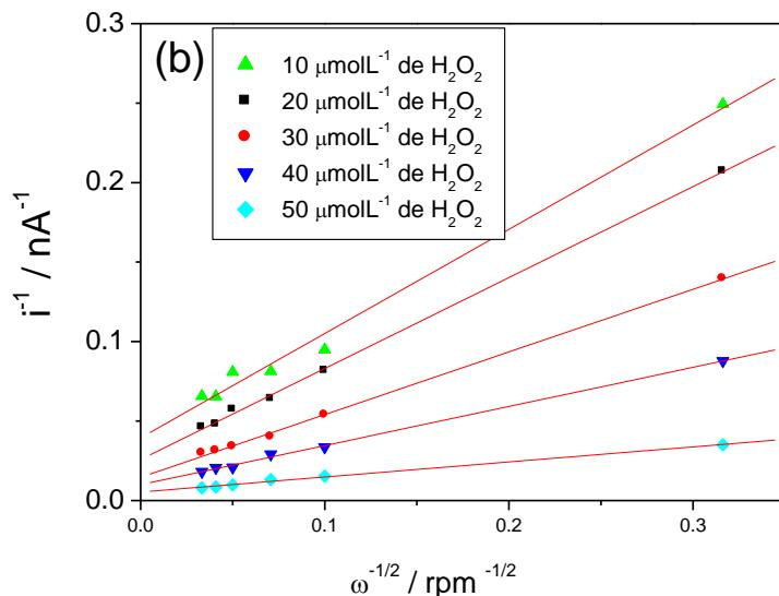
**Figure 2.** (a) Koutecky-Levich plots of  $\text{H}_2\text{O}_2$  reduction at: (a) HRP/MWCNT and (b) HRP/MPy/AuNP/MWCNT modified electrode at various  $\text{H}_2\text{O}_2$  concentrations: (1)  $10 \mu\text{molL}^{-1}$ ; (2)  $20 \mu\text{molL}^{-1}$ ; (3)  $30 \mu\text{molL}^{-1}$ ; (4)  $40 \mu\text{molL}^{-1}$  and (5)  $50 \mu\text{molL}^{-1}$  in 0.1 M phosphate buffer solution, (pH 7.0). Applied potential, -0.25 V/ Ag/AgCl.
