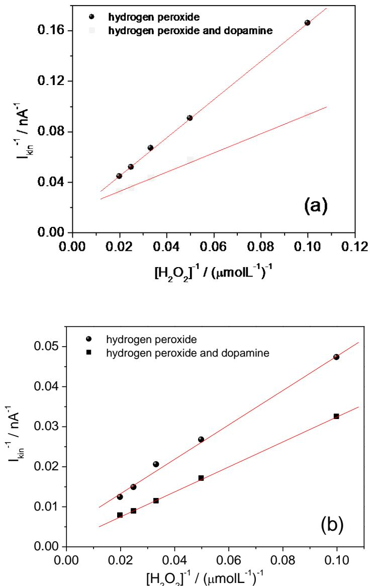
**Figure 3.** The kinetically limited currents (from the intercepts of Koutecky–Levich plots of Figure 2a-b) plotted versus the hydrogen peroxide concentration in inverted co-ordinates for: 0; 100  $\mu$  molL $^{-1}$ dopamine using (a) the HRP/MWCNT and (b) HRP/MPy/AuNP/MWCNT modified electrode.
