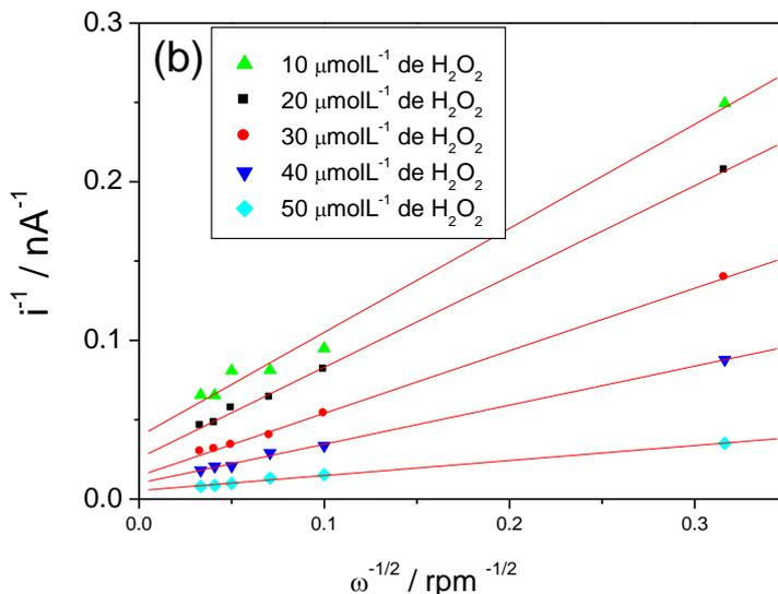
**Figure 2.** (a) Koutecky-Levich plots of H<sub>2</sub>O<sub>2</sub> reduction at: (a) HRP/MWCNT and (b) HRP/MPy/AuNP/MWCNT modified electrode at various H<sub>2</sub>O<sub>2</sub> concentrations: (1) 10 μmolL<sup>-1</sup>; (2) 20 μmolL<sup>-1</sup>; (3) 30 μmolL<sup>-1</sup>; (4) 40 μmolL<sup>-1</sup> and (5) 50 μmolL<sup>-1</sup> in 0.1 M phosphate buffer solution, (pH 7.0). Applied potential, -0.25 V/ Ag/AgCl.
