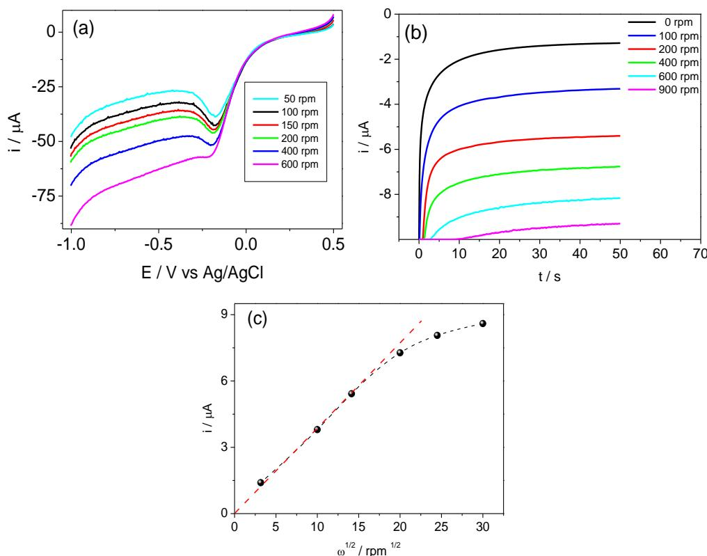
**Figure 1.** (a) Linear sweep voltammograms for glassy carbon electrode modified with HRP/MWCNT in  $50\mu\text{molL}^{-1}$  of  $\text{H}_2\text{O}_2$  at various rotation rates of the electrode and (b) Hydrodynamic amperometry for a glassy carbon electrode modified with HRP/MWCNT in  $10\mu\text{molL}^{-1}$  of  $\text{H}_2\text{O}_2$  at various rotation rates of the electrode. Applied potential, -0.25 V/ Ag/AgCl. (c) Levich Plot from plots in (b).
