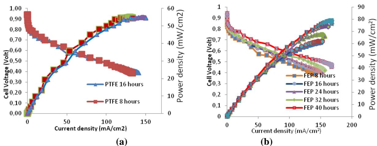
**Figure 6.** Polarization curves; (a) MPL-PTFE, (b) MPL-FEP
