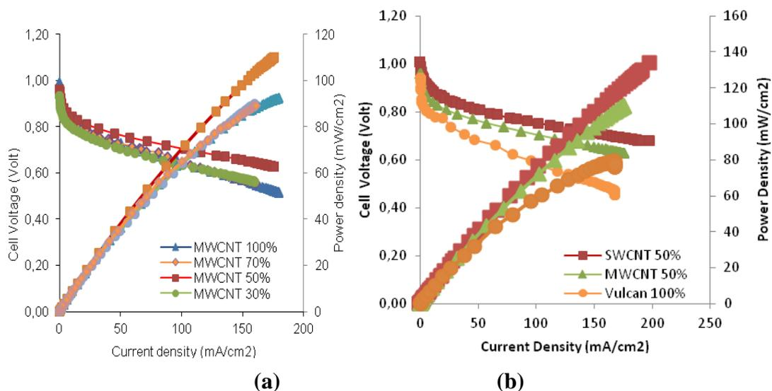
**Figure 7.** Polarization and power density MEA; (a) MWCNT varied composition; (b) comparison MWCNT, SWCNT and Vulcan
