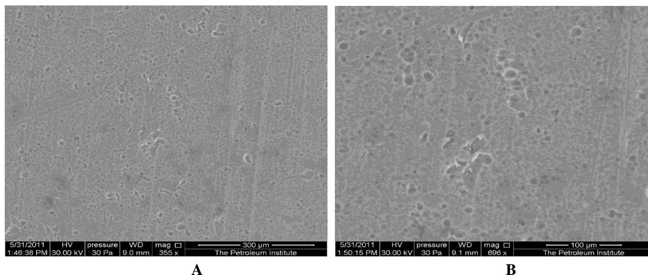
**Figures 3 A-C.** ESEM images of the Indian aluminum sample after exposure to red cabbage solution at boiling temperature for 20 minutes.
