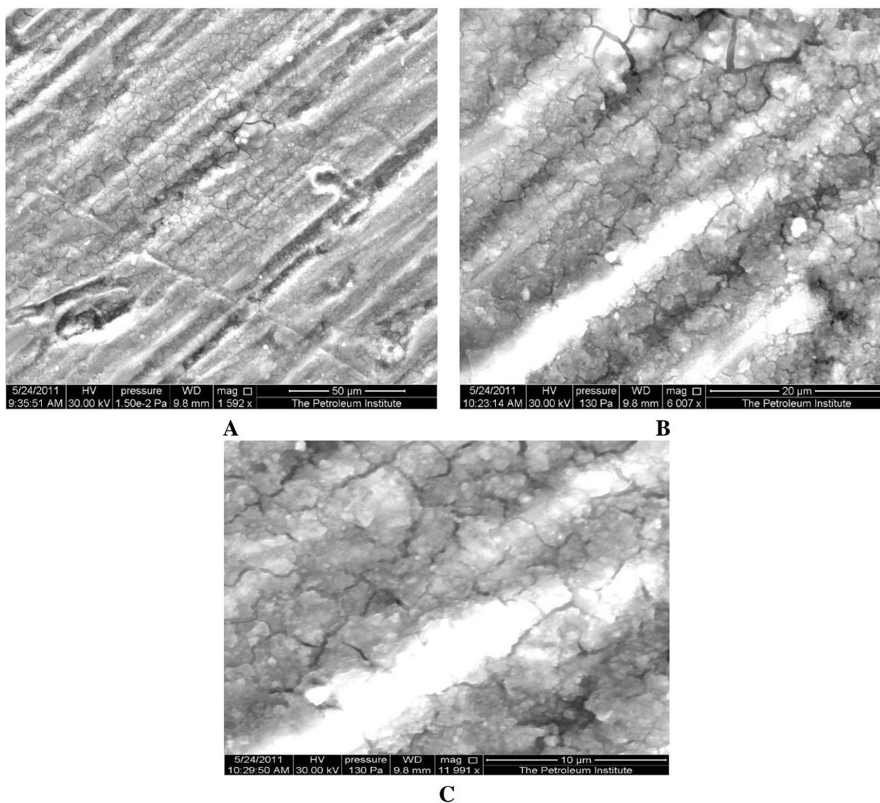
**Figures 1 A-C.** ESEM images of the Indian aluminum sample after exposure to green cabbage solution at boiling temperature for 20 minutes.
