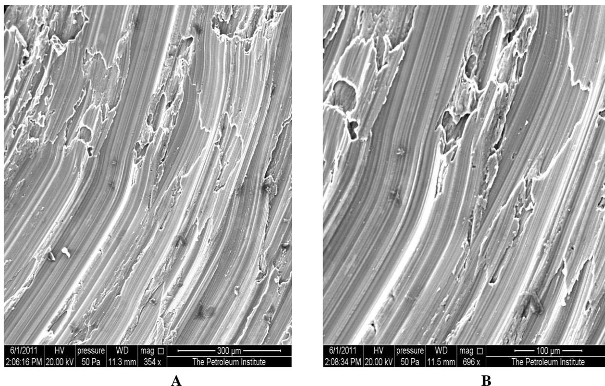
**Figures 5 A-B.** ESEM images of the Indian sample after exposure to peeled eggplant solution at boiling temperature for 20 minutes
