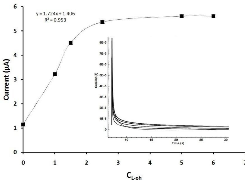
**Figure 3.** Amperometric curve for the enzyme electrode at constant voltage of 1 mV, L-phe concentration increases respectively by 0.0, 1, 1.5, 2.5, 5 and 6 mM of L-phe.
