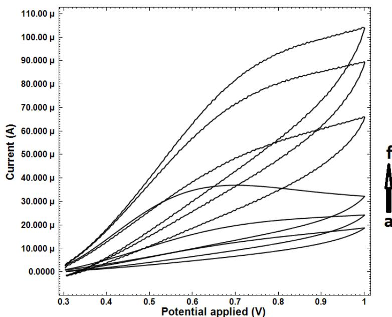
**Figure 8.** Cyclic voltammetry curves of enzyme electrode in the presence of both BSA and glutaraldehyde at scan rate of 20 mV/s containing 2.5 mM NAD<sup>+</sup>, a) without L-phe, b) 0.5, c) 1, d) 2.5, e) 4.5, f) 5 mM, of L-phe.
