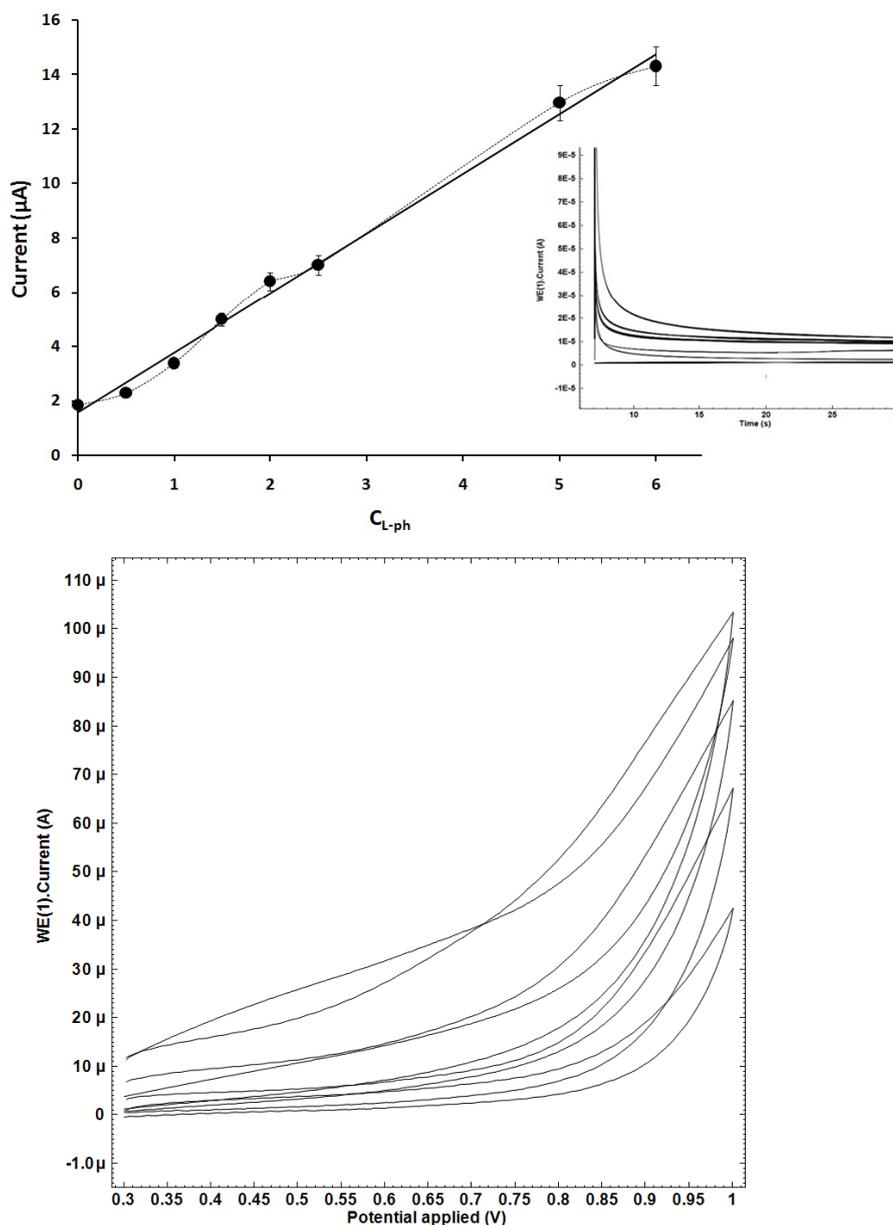
**Figure 12.** (A) Cyclic voltammograms of immobilized enzyme after 16 days at scan rate of 20 mV/s containing 2.5 mM  $\text{NAD}^+$  respectively in the absence and presence of L-Phe at 0.5, 1.0, 1.5, 2.0, 2.5 mM (B) Chronoamperometric curve for enzyme-functionalized electrode after 16 days at constant potential of 1.0V which rise respectively at: 0.5, 1, 1.5, 2, 3 mM concentrations.
