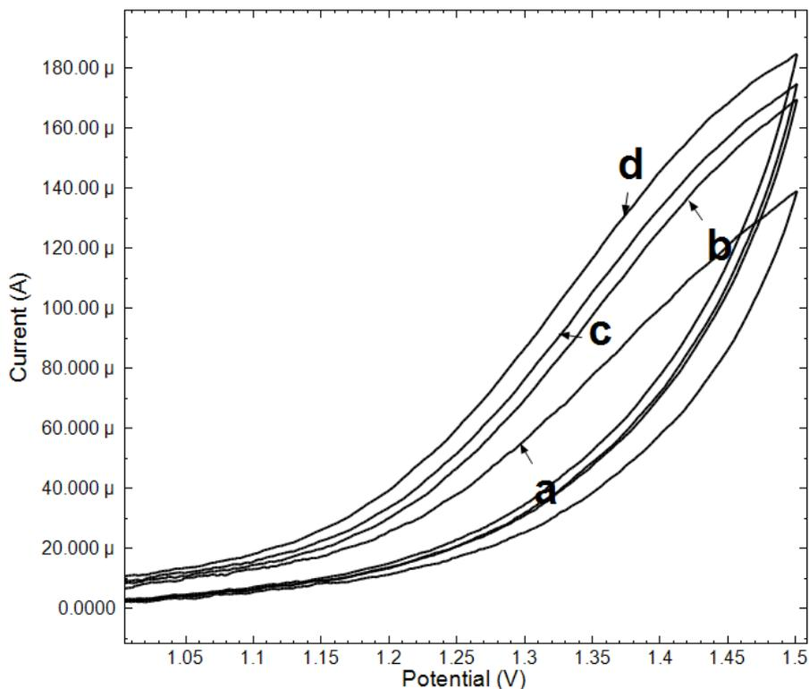
**Figure 6.** Cyclic voltammetry curves of enzyme electrode in the presence of glutaraldehyde at scan rate of 20 mV/s containing 2.5 mM NAD<sup>+</sup>, a) without L-phe, b) 1 mM, c) 1.5 mM, d) 2.5 mM of L-phe.
