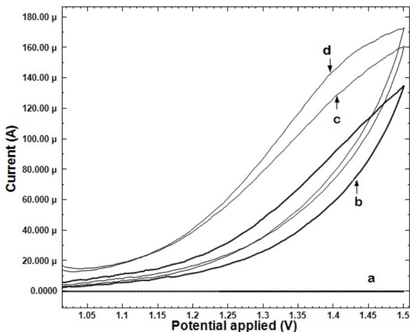
**Figure 2.** Cyclic voltammetry curve of enzyme electrode at scan rate of 20 mV/s containing 2.5 mM  $\text{NAD}^+$ : a) No electrodes, b) without L - phe, c) 1.5 mM of L - phe, d) 2.5 mM of L-phe.
