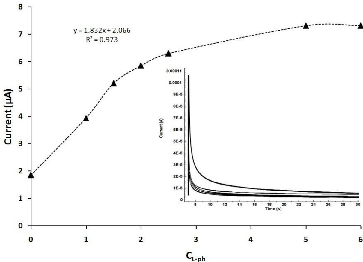
**Figure 5.** Amperometric curve for enzyme electrode in the presence of BSA protein at the constant voltage of 1 mV, L-phe concentration increases respectively by 0.0, 1, 1.5, 2, 2.5, 5 and 6 mM of L-phe.
