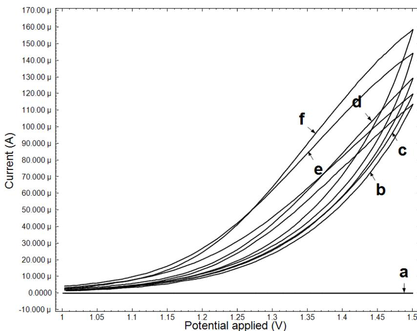
**Figure 9.** Cyclic voltammograms of enzyme electrode in the presence of both BSA and glutaraldehyde at scan rate of 20 mV/s containing 2.5 mM  $\text{NAD}^+$ , a) No electrode, b) without L-phe, c) 0.5, d) 1, e) 2 mM of L-phe.
