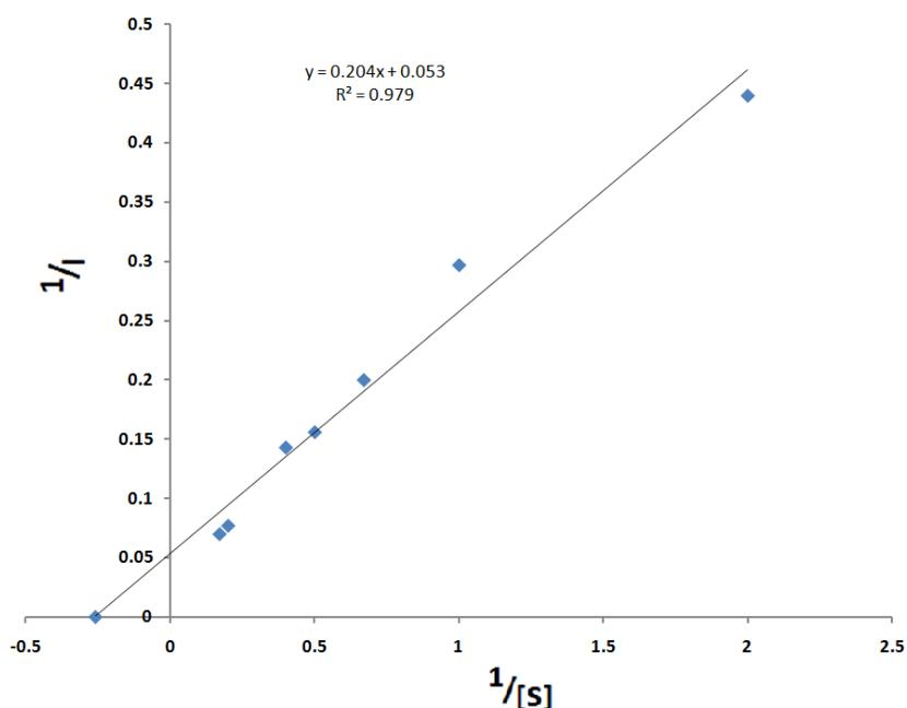
**Figure 11.** Lineweaver–Burk plot for coated glassy carbon electrode at constant potential of 1.0V at L-phe concentrations of: 0.5, 1.0, 1.5, 2.0, 2.5, 5, 6 mM respectively.
