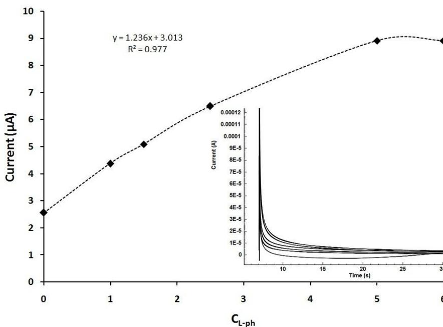
**Figure 7.** Amperometric curve for enzyme electrode in the presence of BSA protein at the constant voltage of 1 mV, L-phe concentration increases respectively by 0.0, 1, 1.5, 2, 2.5, 5 and 6 mM of L-phe.
