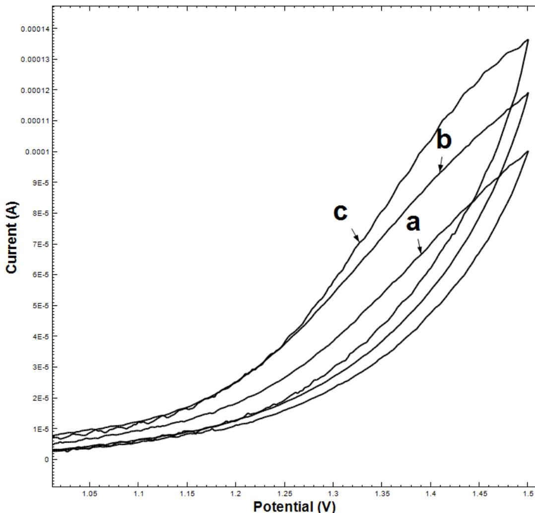
**Figure 4.** Cyclic voltammetry curves of enzyme electrode in the presence of BSA protein at scan rate of 20 mV/s containing 2.5 mM  $\text{NAD}^+$ , a) without L-phe, b) 2.5 mM, c) 5 mM of L-phe.
