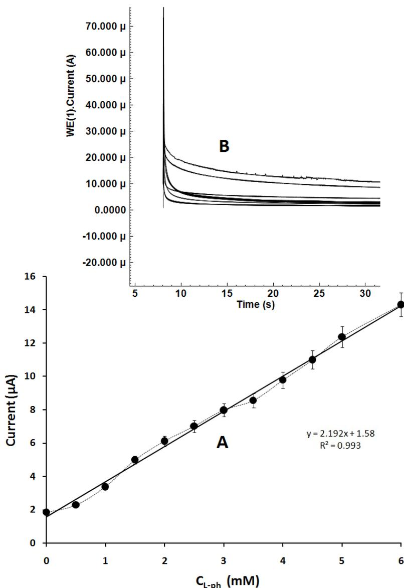
**Figure 10.** A) Amperometric curve for enzyme electrode in the presence of both GA and BSA protein at the constant voltage of 1 mV, L-phe concentration increases respectively B) by 0, 0.5, 1, 1.5, 2, 2.5, 5 and 6 mM of L-phe.
