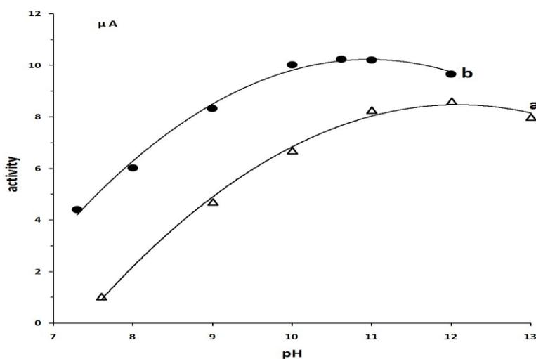
**Figure 1.** Effect of pH on catalytic activity (amperometric response) of the native enzyme (a) and that of the enzyme electrode (b). Applied potential: 1.0V; temperature: 23 °C; initial working volume: 12ml; supporting electrode: 100mM Gly/KOH/KCl buffer pH 10.5 containing 2.5mM  $\text{NAD}^+$ .
