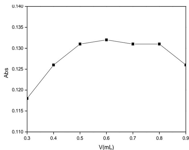
**Figure 4.** Effect of the volume of carboxylic CNTs on the absorbance
