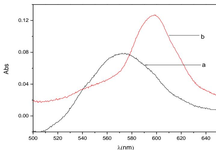
**Figure 1.** Absorption spectra of different chromogenic system a.  $\text{Pb}^{2+}$ -PF complex measured against blank PF b.  $\text{Pb}^{2+}$ -PF-carboxylic CNTs-CTMAB complex measured against blank PF-carboxylic CNTs-CTMAB
