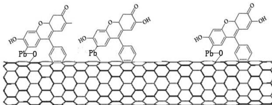
**Figure 2.** The  $Pb^{2+}$ -PF complex absorbing onto the sidewall of carboxylic CNTs
