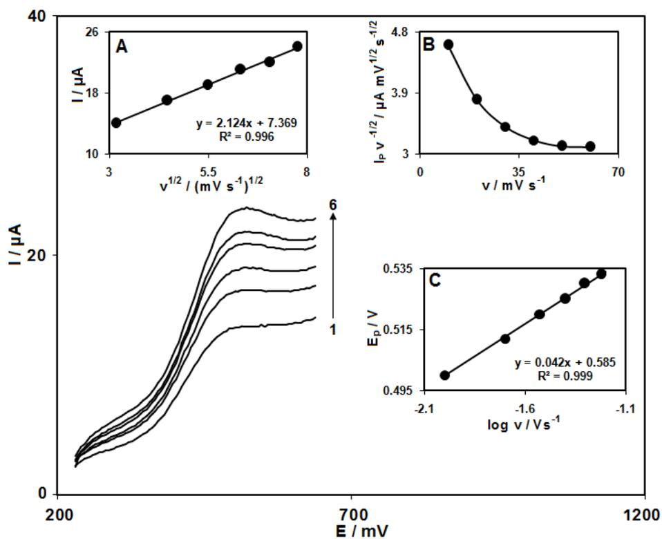
**Figure 2.** Linear sweep voltammograms of FCDCNPE in 0.1 M phosphate buffer solution (pH 5.0) containing 200.0  $\mu\text{M}$  NE at various scan rates; From inner to outer scan rates of 10, 20, 30, 40, 50 and 60  $\text{mV s}^{-1}$ , respectively. Insets: Variation of (A) anodic peak current vs.  $v^{1/2}$ ; (B) normalized current ( $I_p/v^{1/2}$ ) vs.  $v$ ; (C) anodic peak potential vs.  $\log v$ .
