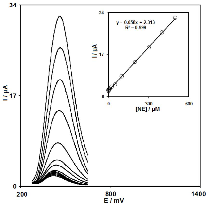
**Figure 4.** Differential pulse voltammograms of FCDCNPE in 0.1 M phosphate buffer solution (pH 5.0) containing different concentrations of NE. From inner to outer correspond to 0.03, 0.1, 0.5, 1.0, 5.0, 10.0, 25.0, 50.0, 100.0, 200.0, 300.0, 400.0 and 500.0  $\mu\text{M}$  of NE. Inset show the plots of the electrocatalytic peak current as a function of NE concentration in the range of 0.03 to 500.0  $\mu\text{M}$ .
