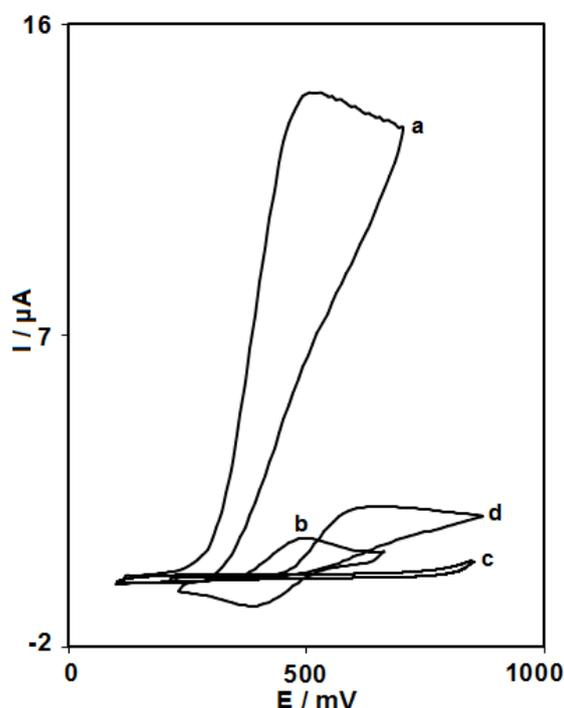
**Figure 1.** Cyclic voltammograms of FCDCNPE at  $10 \text{ mV s}^{-1}$  in 0.1M phosphate buffer (pH 5.0): (a) In the presence and (b) in the absence of  $200.0 \text{ }\mu\text{M}$  NE; (c) and (d) for an unmodified carbonpaste electrode in the absence and presence of  $200.0 \text{ }\mu\text{M}$  NE, respectively.
