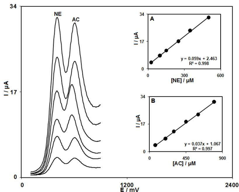
**Figure 5.** DPVs of FCDCNPE in 0.1 M phosphate buffer solution (pH 5.0) containing different concentrations of NE+AC in  $\mu\text{M}$ , from inner to outer: 25.0+75.0, 100.0+200.0, 150.0+300.0, 250.0+450.0, 350.0+600.0 and 500.0+800.0 respectively. Insets (A) and (B) are plots of  $I_p$  vs. NE and AC concentrations, respectively.
