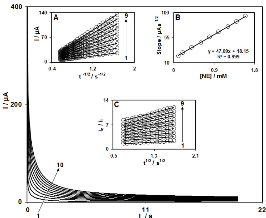
**Figure 3.** (A) Chronoamperograms obtained at FCDCNPE in 0.1 M phosphate buffer solution (pH 5.0) for different concentration of NE. The numbers 1–10 correspond to 0.0, 0.1, 0.2, 0.4, 0.6, 0.8, 1.0, 1.2, 1.4 and 1.6 mM of NE. Insets: (A) Plots of  $I$  vs.  $t^{-1/2}$  obtained from chronoamperograms 2–10. (B) Plot of the slope of the straight lines against NE concentration; (C) dependence of  $I_{cat}/I_l$  on  $t^{1/2}$  derived from the data of chronoamperograms 1-10.
