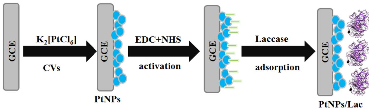
**Scheme 1.** Construction of the PtNPs/laccase modified electrodes.
