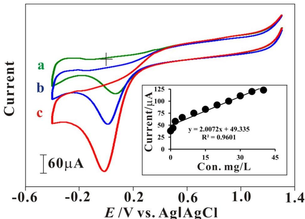
**Figure 3.** CVs recorded at a PtNPs/laccase modified electrode in 0.1M PBS (pH 7.0 containing 1 mM ABTS ) saturated with nitrogen (curve a), ambient air (curve b) and oxygen (curve c). Scan rate  $100 \text{ mVs}^{-1}$  in the potential range of 1.3 to -0.4 V. Inset shows a current vs. concentration plot of oxygen at PtNPs/laccase electrode.
