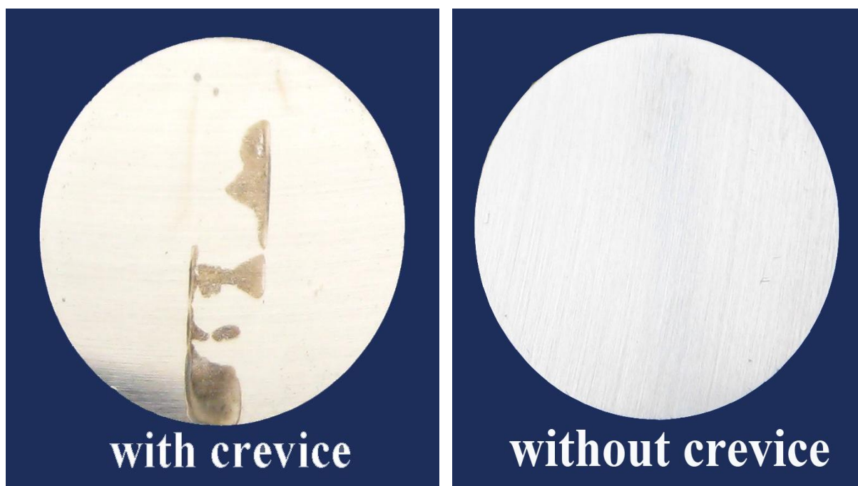
Figure 5. The macroscopic corrosion morphology of 316L SS with and without crevice after potentiostatic polarization measurement.
