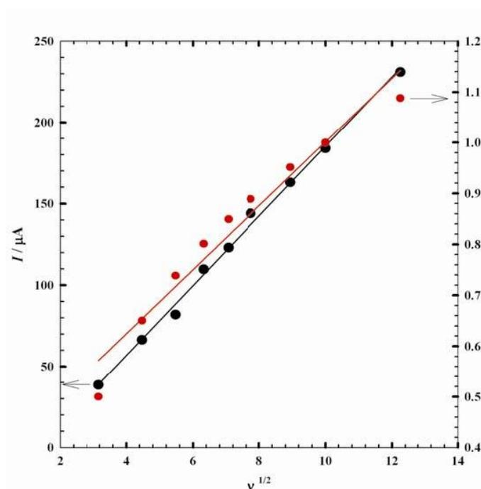
**Figure 3.** A plot of the anodic peak current values as a function of the square root of the scan rate at PEDOT/Pt electrode (a) in presence and (b) in absence of SDS.
