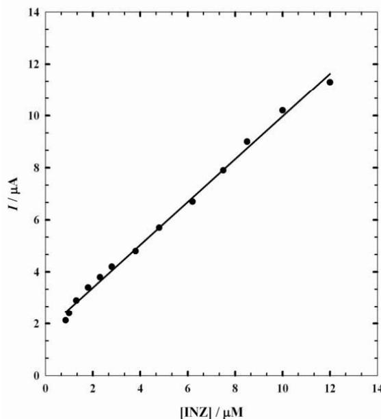
**Figure 10.** Calibration curve for successive additions of 10 μL of 5 mmol L<sup>-1</sup> INH in urine to the buffer pH 2.3 containing 150 μL SDS.
