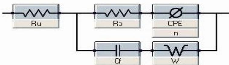
**Figure 9.** Equivalent circuit
