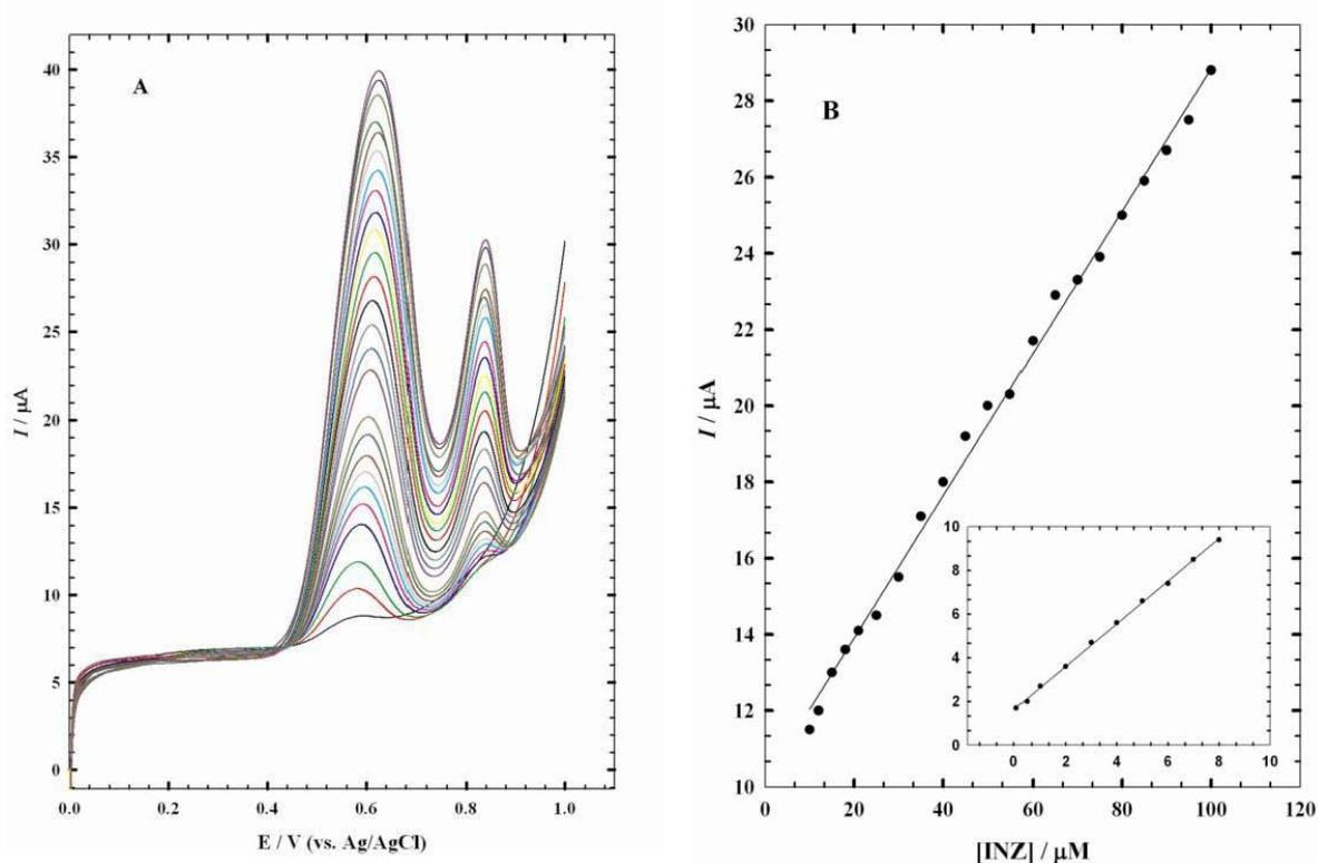
**Figure 5 A.** LSVs of different concentrations of INH ( $0.1 \mu\text{mol L}^{-1}$  -  $0.1 \text{ mmol L}^{-1}$ ) in  $10 \text{ mL}$  of  $0.1 \text{ mol L}^{-1}$  B-R pH 2.3 containing  $150 \mu\text{L}$   $0.1 \text{ mol L}^{-1}$  SDS at PEDOT/Pt electrode. **(B)** Calibration curve for INH of different concentrations from ( $10 \mu\text{mol L}^{-1}$  to  $0.1 \text{ mmol L}^{-1}$ ) and from ( $0.1 \mu\text{mol L}^{-1}$  to  $8 \mu\text{mol L}^{-1}$ ) (inset).
