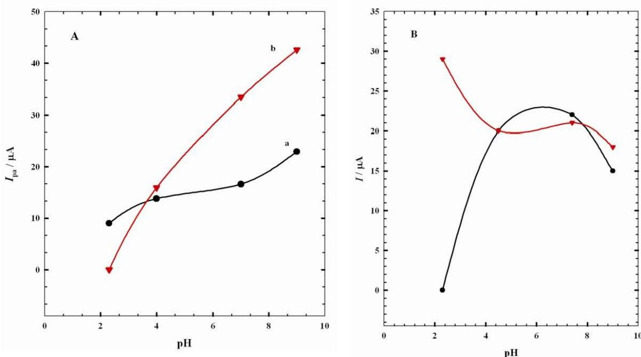
**Figure 4.** A plot of the anodic peak current values as a function of the pH value of the solution at PEDOT/Pt electrode (a) in absence and (b) in presence of (A) CTAB and (B) SDS.
