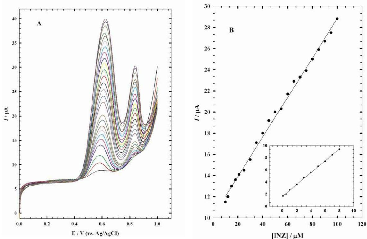
**Figure 5 A.** LSVs of different concentrations of INH ( $0.1 \mu\text{mol L}^{-1}$  -  $0.1 \text{ mmol L}^{-1}$ ) in  $10 \text{ mL}$  of  $0.1 \text{ mol L}^{-1}$  B-R pH 2.3 containing  $150 \mu\text{L}$   $0.1 \text{ mol L}^{-1}$  SDS at PEDOT/Pt electrode. **(B)** Calibration curve for INH of different concentrations from ( $10 \mu\text{mol L}^{-1}$  to  $0.1 \text{ mmol L}^{-1}$ ) and from ( $0.1 \mu\text{mol L}^{-1}$  to  $8 \mu\text{mol L}^{-1}$ ) (inset).
