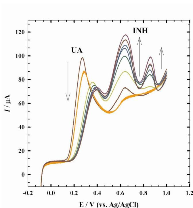
**Figure 6.** LSV for 50 mmol  $\text{L}^{-1}$  AA, 5 mmol  $\text{L}^{-1}$  UA and 0.5 mmol  $\text{L}^{-1}$  INH in B-R (0.1 mol  $\text{L}^{-1}$ ), at PEDOT/Pt with successive additions of ( 0 -150  $\mu\text{L}$ ) 0.1 mol  $\text{L}^{-1}$  SDS , at pH 2.3
