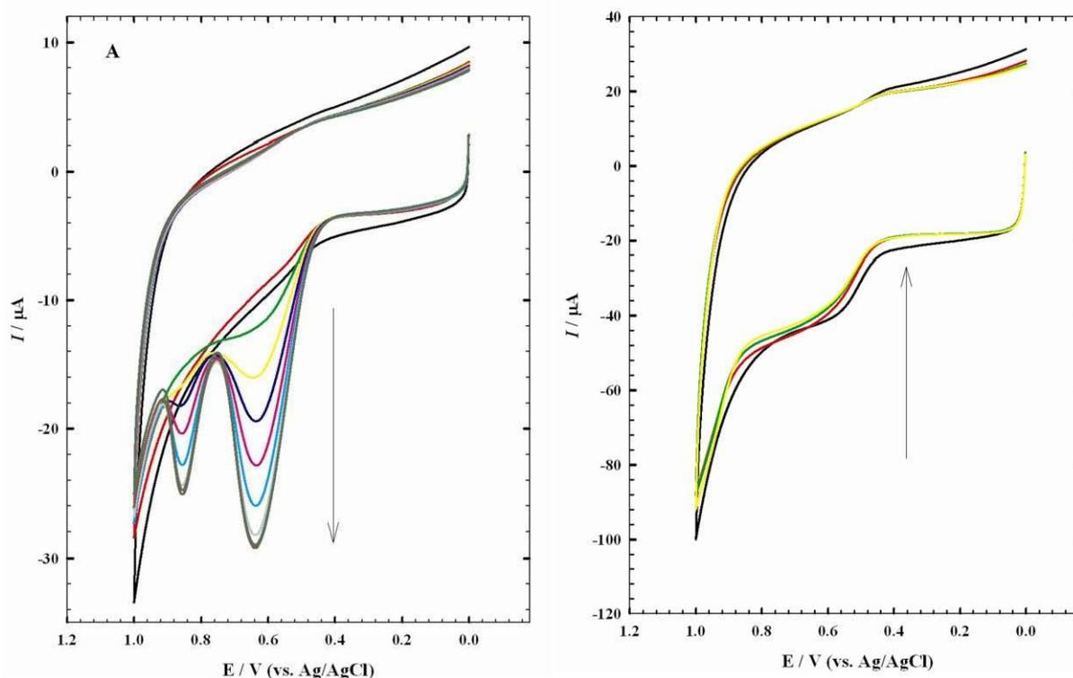
**Figure 1.** Cyclic voltammograms of  $5.0 \times 10^{-4}$  mol L<sup>-1</sup> INH / 0.1 mol L<sup>-1</sup> B-R, scan rate  $50 \text{ mV s}^{-1}$  at PEDOT/Pt electrode at pH 2.3 with successive additions (0  $\mu\text{L}$  – 150  $\mu\text{L}$ ) of 0.1 mol L<sup>-1</sup> (A) SDS, (B) CTAB.
