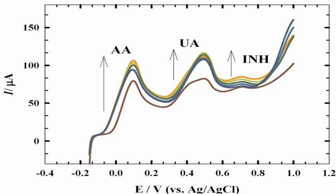
**Figure 7.** LSV for  $50 \text{ mmol L}^{-1}$  AA,  $5 \text{ mmol L}^{-1}$  UA and  $0.5 \text{ mmol L}^{-1}$  INH in B-R ( $0.1 \text{ mol L}^{-1}$ ), at PEDOT/Pt with successive additions of ( $0$  -  $150 \mu\text{L}$ )  $0.1 \text{ mol L}^{-1}$  CTAB, at pH 7.3.
