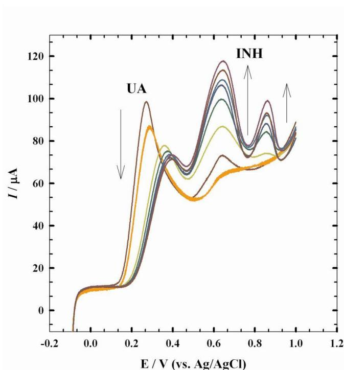
**Figure 6.** LSV for 50 mmol  $\text{L}^{-1}$  AA, 5 mmol  $\text{L}^{-1}$  UA and 0.5 mmol  $\text{L}^{-1}$  INH in B-R (0.1 mol  $\text{L}^{-1}$ ), at PEDOT/Pt with successive additions of ( 0 -150  $\mu\text{L}$ ) 0.1 mol  $\text{L}^{-1}$  SDS , at pH 2.3
