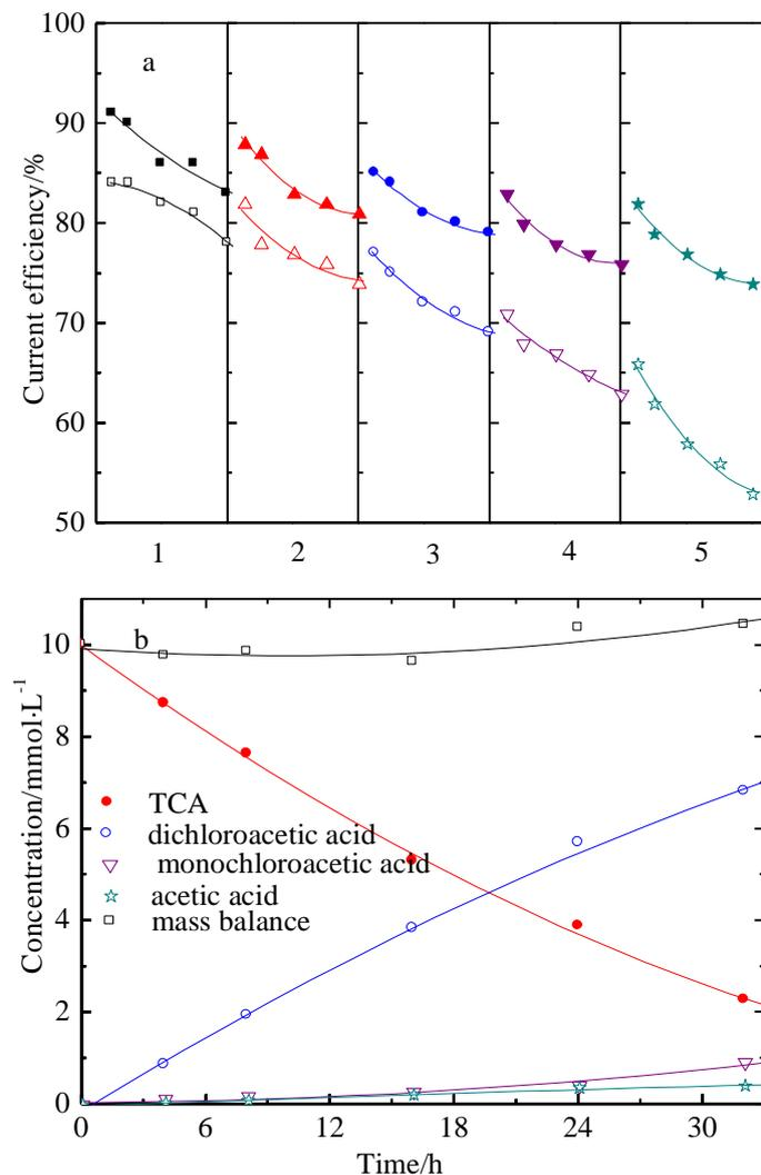
**Figure 3.** (a) Hb-MWCNT-GE (open symbols) and Hb/SA-MWCNT-GE (filled symbols) stability test registered during the reaction conducted one, two, three, four and five times using the same electrode corresponding respectively to (1), (2), (3), (4) and (5) in abscissa; (b) the intermediate products analysis of TCA dechlorination on Hb/SA-MWCNT-GE. Conditions: TCA, 10 mM; T, 25 °C; current, 2 mA; supporting electrolyte, 0.1 M pH 7.0 PBS.
