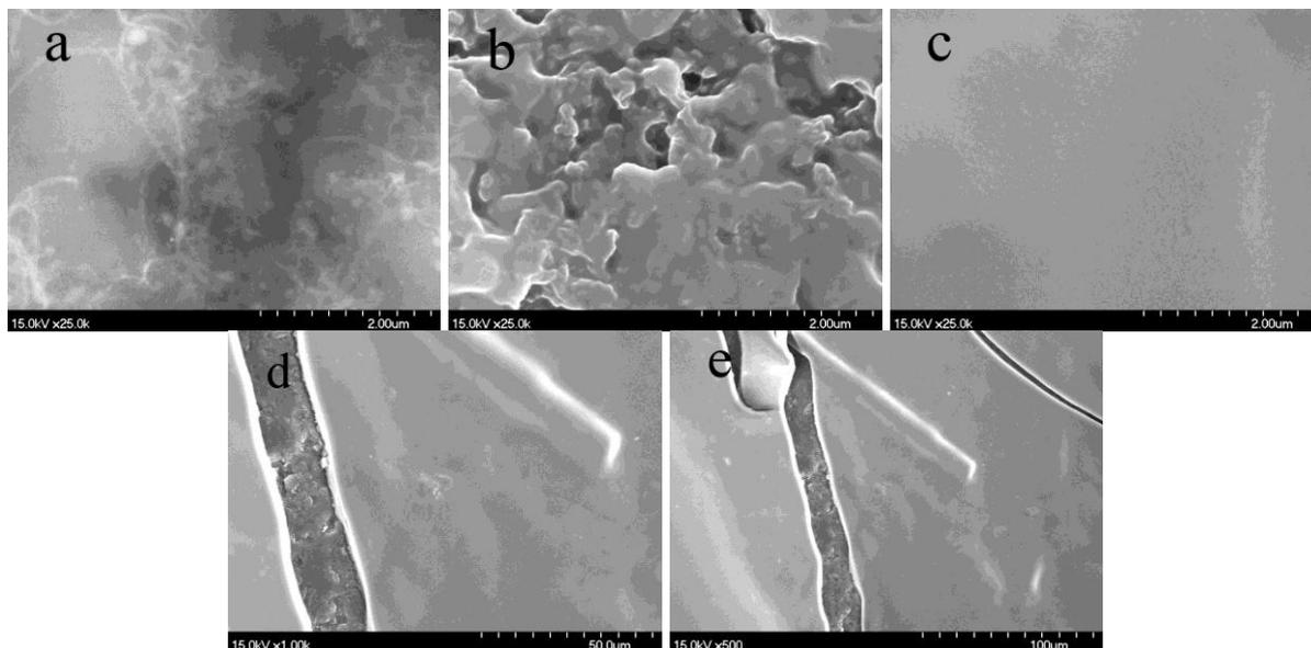
**Figure 1.** SEM image of MWCNTs (a), Hb-MWCNT (b), and Hb/SA-MWCNT (c, d, e).
