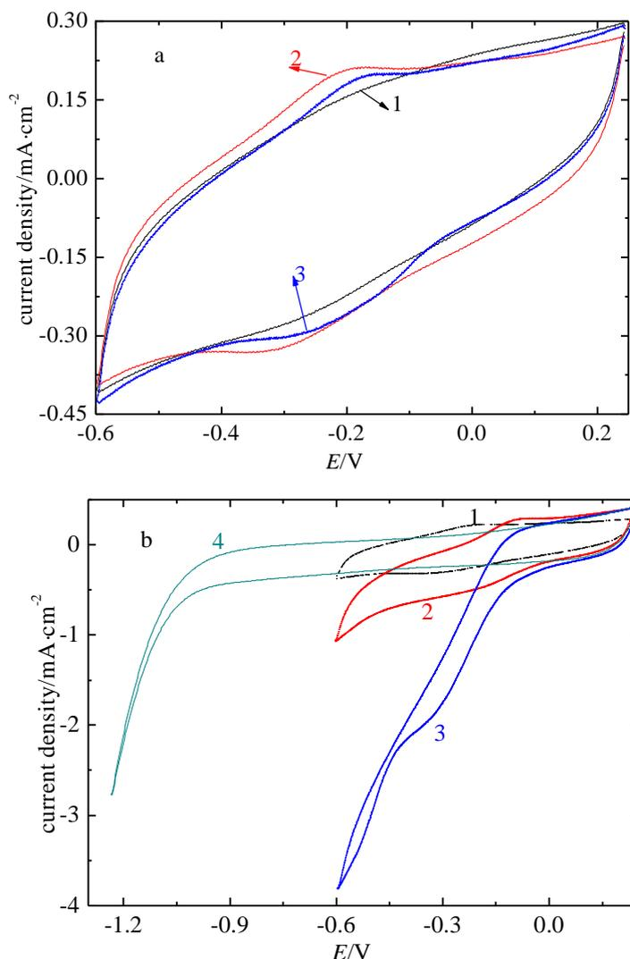
**Figure 2.** (a) Cyclic voltammograms of the SA-MWCNT-GE (curve 1), Hb/SA-MWCNT-GE (curve 2), and Hb-MWCNT-GE (curve 3) in 0.1 M pH 7.0 PBS at a scan rate of  $300 \text{ mV}\cdot\text{s}^{-1}$ . (b) Cyclic voltammograms at a scan rate of  $300 \text{ mV}\cdot\text{s}^{-1}$  in 0.1 M pH 7.0 PBS: Hb/SA-MWCNT-GE with no TCA (curve 1), Hb/SA-MWCNT-GE containing 0.1 M TCA (curve 2), Hb/SA-MWCNT-GE containing 0.2 M TCA (curve 3), SA-MWCNT-GE containing 0.1 M TCA (curve 4).
