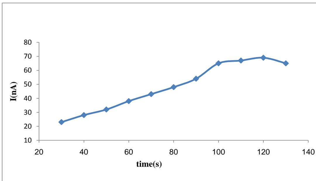
**Figure 3.** Peak heights in dependence on the accumulation time. Conditions: :  $1 \times 10^{-7}$  M GA, accumulation potential, +50 mV; sweep rate, 60 mV/s.
