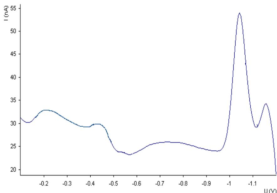
**Figure 1.** Differential plus voltammogram for determination of GA. Conditions:  $1 \times 10^{-7}$  M GA, initial potential, +100 mV: final potential, -1200 mV; accumulation potential, +50 mV; accumulation time, 50 s and sweep rate, 60 mV/s.
