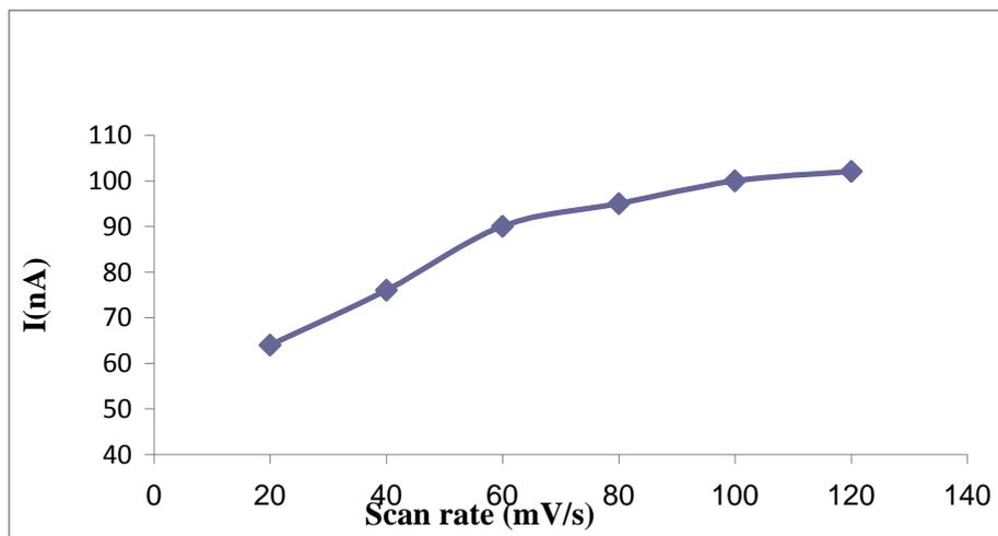
**Figure. 5.** Effect of Scan rate on the peak current. Conditions:  $1 \times 10^{-7}$  M GA, accumulation potential, +50 mV; accumulation time, 100 s.
