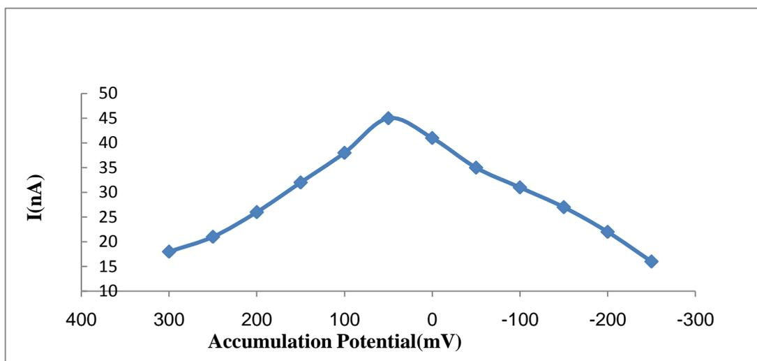
**Figure 4.** Peak heights in dependence on the accumulation potential. Conditions: :  $1 \times 10^{-7}$  M GA, accumulation time, 50 s and sweep rate, 60 mV/s.
