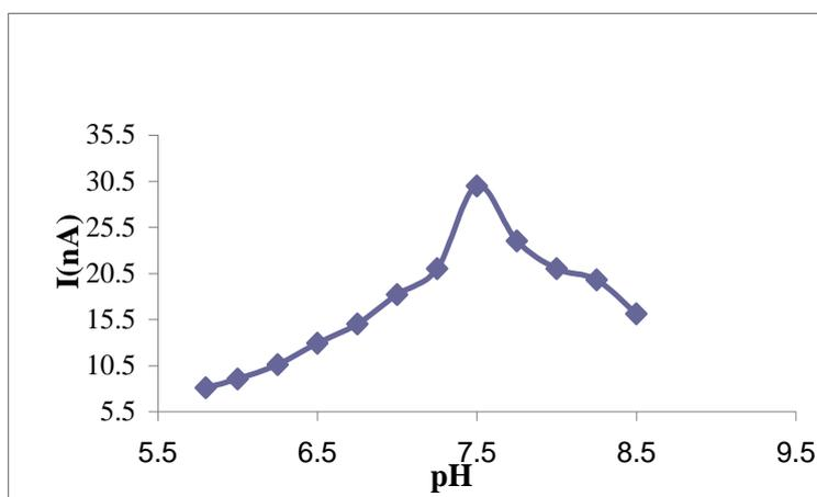
**Figure.2.** Dependence of peak heights on the pH value. Conditions:  $1 \times 10^{-7}$  M GA, accumulation potential +50 mV; accumulation time 50 s and sweep rate 60 mV/s.
