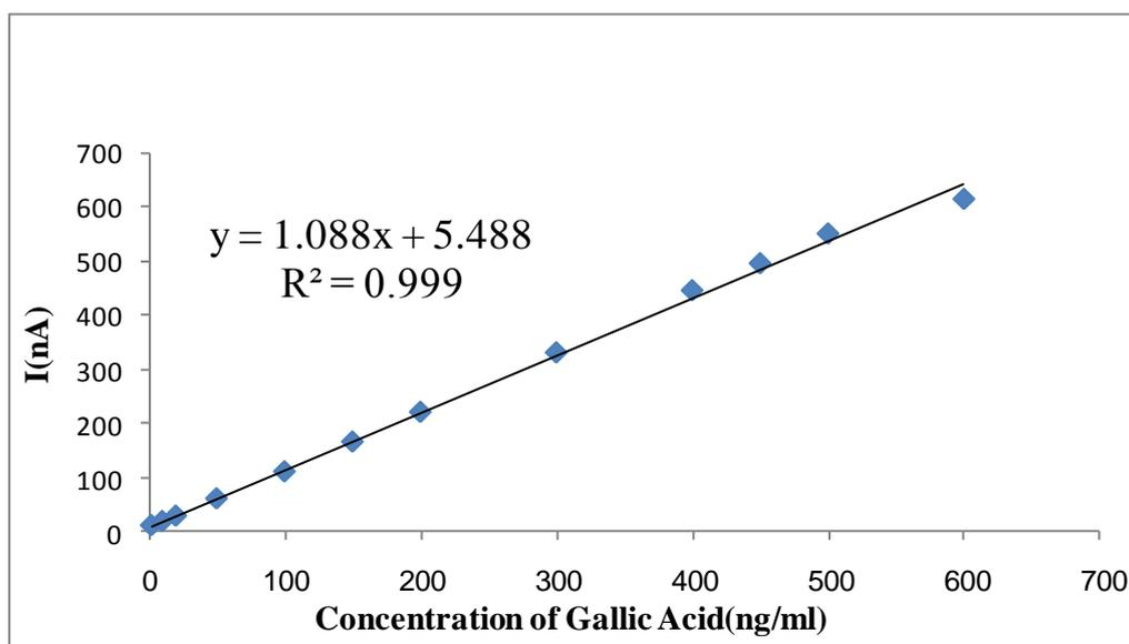
**Figure.6.** Calibration curve for determination of GA from 0.1 to 600 ng/ml. Conditions: accumulation potential, +50 mV; accumulation time, 100 s; scan rate 80 mV/s.
