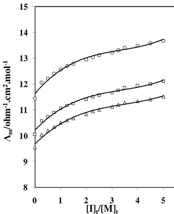
**Figure 4.** Molar conductance-mole ratio plots for (meso-octamethylcalix[4]pyrrole.[Ti(OH)-(H<sub>2</sub>O)<sub>5</sub>])<sup>2+</sup> complexes in EtOH-AN binary system (mol% EtOH=4.5) at different temperatures (Δ= 25°C, □= 35°C, ○= 45°C).
