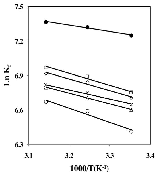
**Figure 5.** Van't Hoff plots for (meso-octamethylcalix[4]pyrrole. $[\text{Ti}(\text{OH})-(\text{H}_2\text{O})_5]^{2+}$  complexes in EtOH-AN binary systems (mol% EtOH:  $\Delta=100$ ,  $\circ=78.2$ ,  $\times=57.3$ ,  $\square=37.4$ ,  $\diamond=18.3$ ,  $\bullet=4.5$ ).
