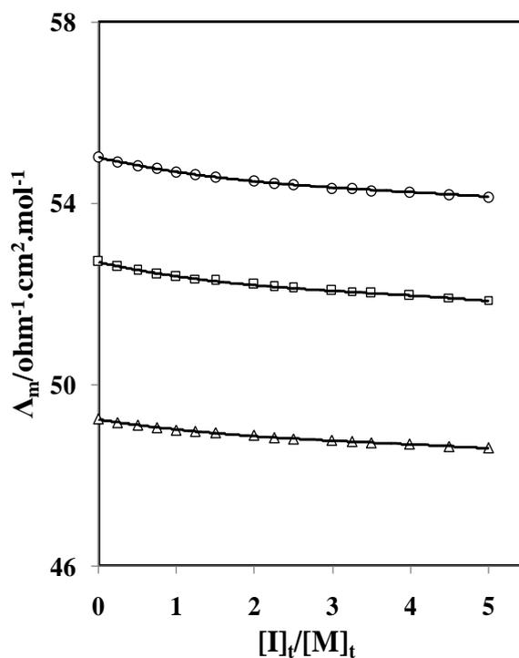
**Figure 2.** Molar conductance-mole ratio plots for (meso-octamethylcalix[4]pyrrole.[Ti(OH)-(H<sub>2</sub>O)<sub>5</sub>]<sup>2+</sup> complexes in EtOH-AN binary system (mol% EtOH=78.2) at different temperatures (Δ= 25°C, □= 35°C, ○= 45°C).
