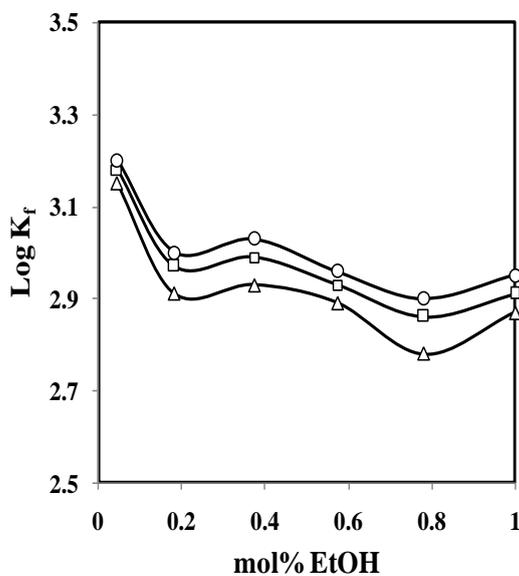
**Figure 6.** Changes of the stability constant ( $\log K_f$ ) of (meso-octamethylcalix[4]pyrrole. $[\text{Ti}(\text{OH})-(\text{H}_2\text{O})_5]^{2+}$  complexes with the composition of EtOH-AN binary systems at different temperatures ( $\Delta=25^\circ\text{C}$ ,  $\square=35^\circ\text{C}$ ,  $\circ=45^\circ\text{C}$ ).
