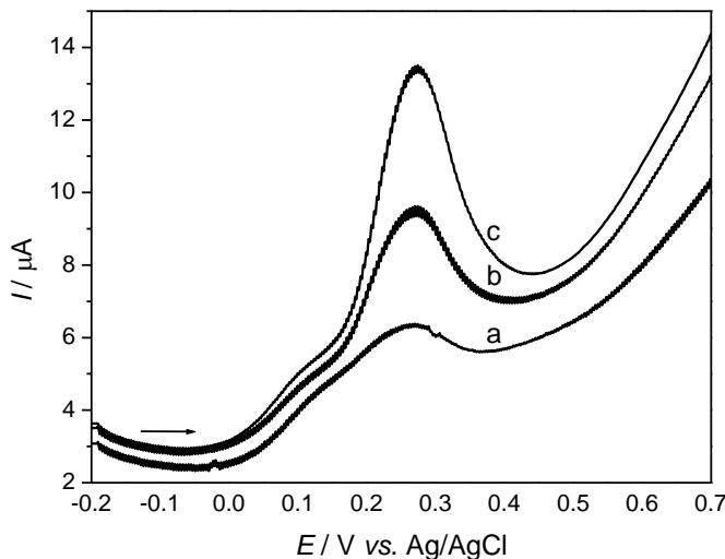
**Figure 6.** Square-wave voltammograms of raspberry extract diluted 100-fold (a), with 3  $\mu\text{mol/L}$  (b) and 5  $\mu\text{mol/L}$  (c) additions of EA made to the solution. All experimental conditions are as in Fig. 4.
