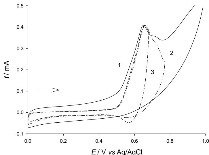
**Figure 1.** Cyclic voltammetry of  $5 \times 10^{-4}$  mol/L ellagic acid on the paraffin impregnated graphite electrode in 0.1 mol/L KNO<sub>3</sub> at pH 2. The scan rate is 25 mV/s and the reversing potential is 1 V (1), 0.772 V (2) and 0.680 V (3).
