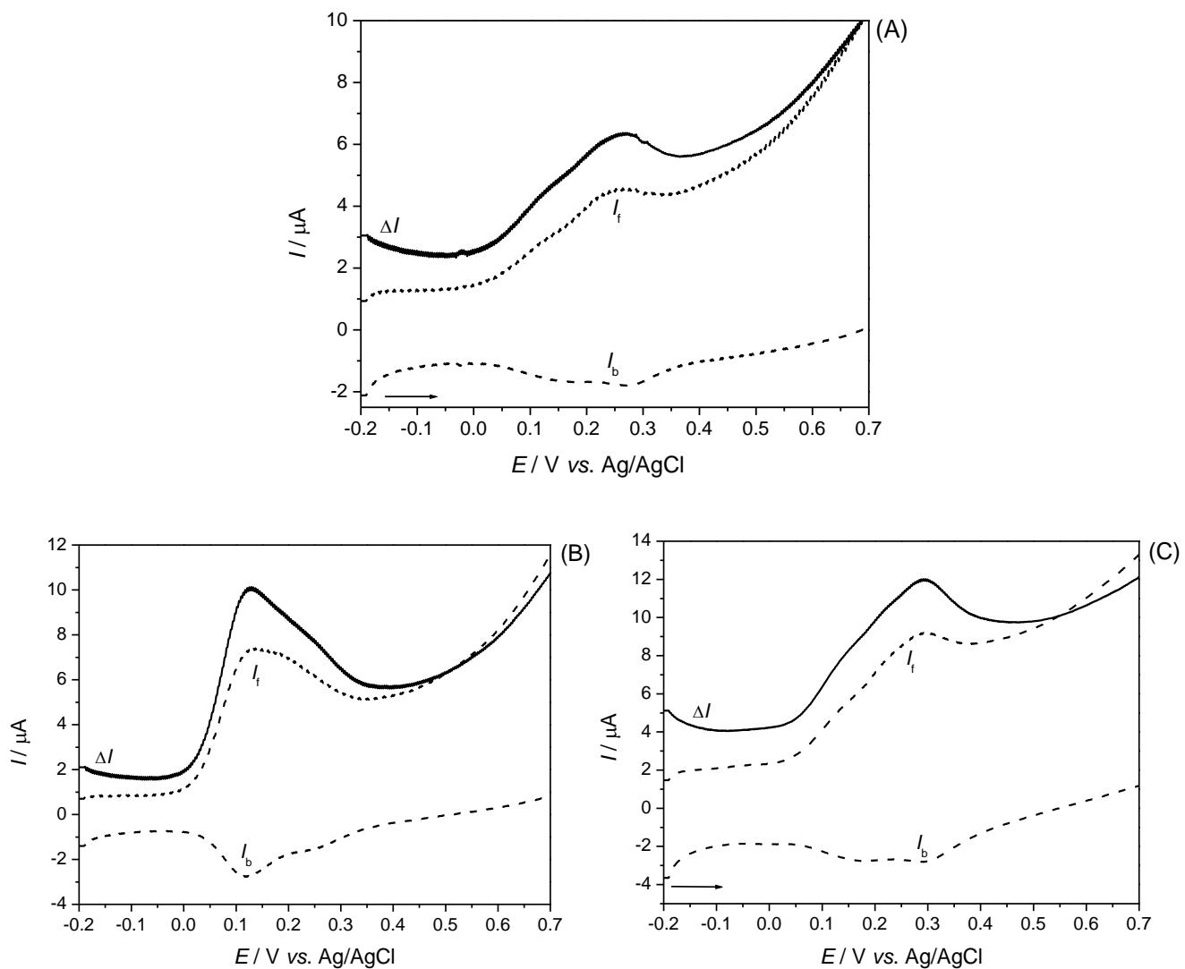
**Figure 4.** Square-wave voltammograms obtained for raspberry (A), blackberry (B) and strawberry (C) extracts. Experimental conditions: pH 6.5, pulse amplitude 50 mV, frequency 100 Hz and step potential 2 mV.
