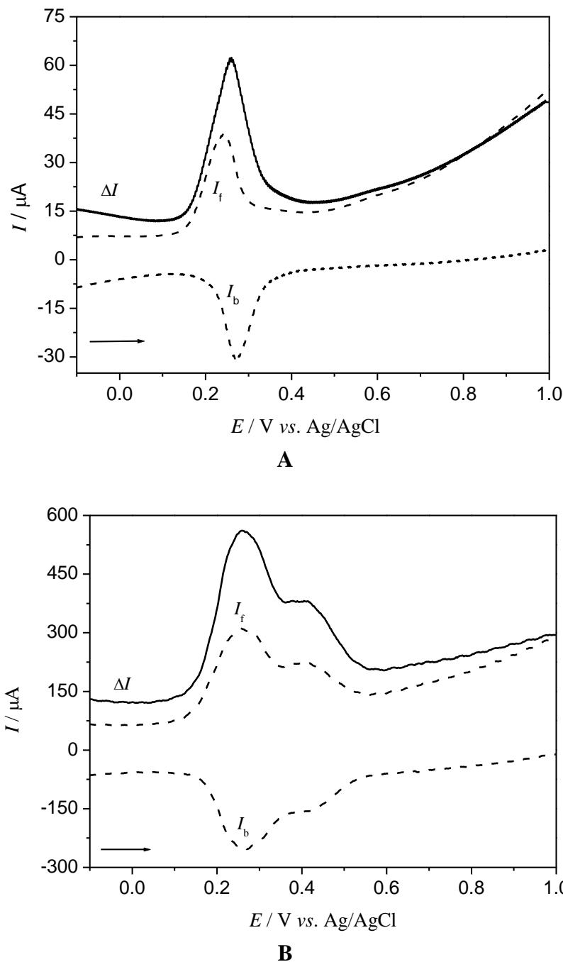
**Figure 2.** Square-wave voltammetry of  $1 \times 10^{-5}$  mol/L ellagic acid on glassy-carbon electrode in 0.1 mol/L KNO<sub>3</sub> at pH 7.  $E_{sw} = 50$  mV,  $dE = 2$  mV and  $f/s^{-1} = 100$  (A) and 1000 (B).
