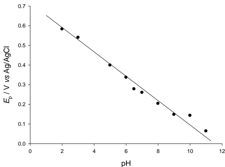
**Figure 3.** Square-wave voltammetry of ellagic acid on GCE. Dependence of peak potentials of the net response (circles) on pH of supporting electrolyte;  $f = 100 \text{ s}^{-1}$  and all other data are as in Figure 2. The straight line is the first approximation:  $E_p = 0.715 - 0.062 \times \text{pH}$  (V).
