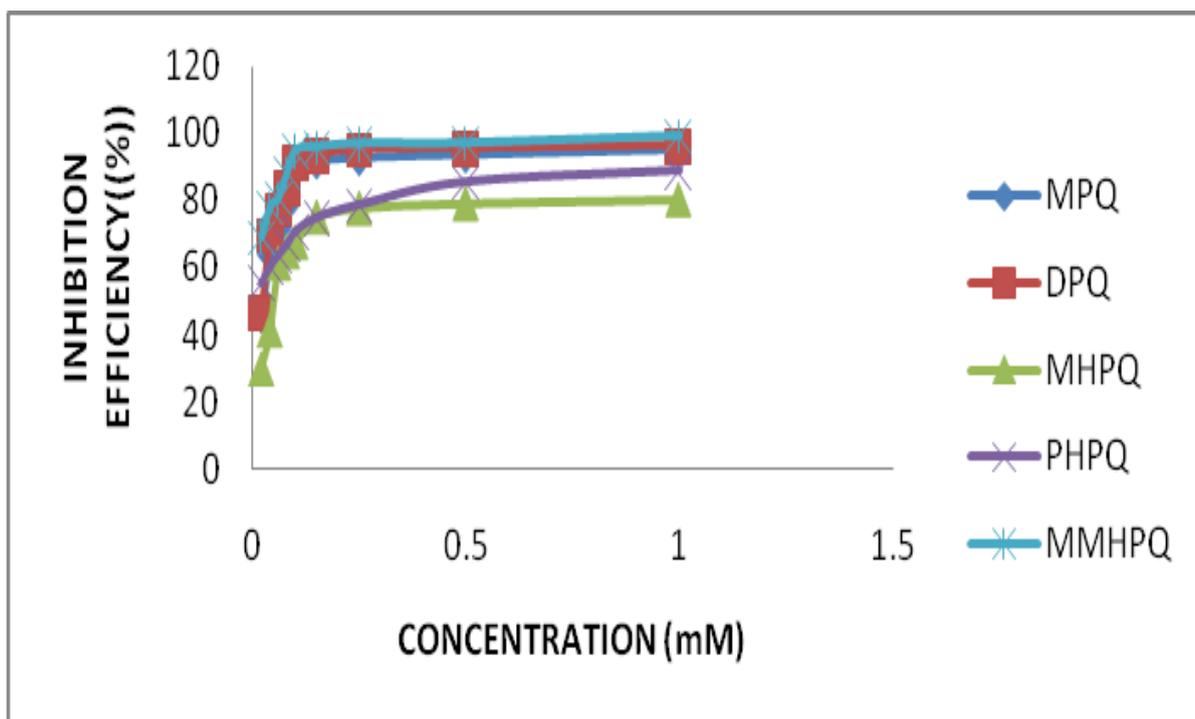
Figure 2. Plot of Inhibition efficiency (%) Vs concentration (mM) for the inhibition of corrosion of mild steel in 1M H<sub>2</sub>SO<sub>4</sub>
