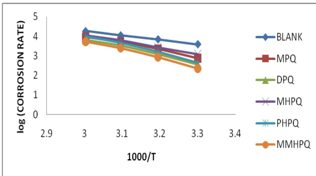
**Figure 3.** Arrhenius plot of corrosion of mild steel in 1M H<sub>2</sub>SO<sub>4</sub> solution in the absence and presence of inhibitors
