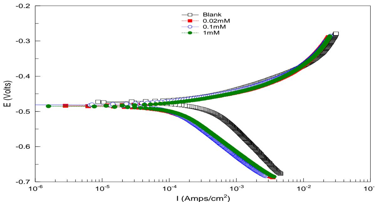
**Figure 6.** Polarization curves for mild steel in 1M H<sub>2</sub>SO<sub>4</sub> for selected concentrations of inhibitor MMHPQ
