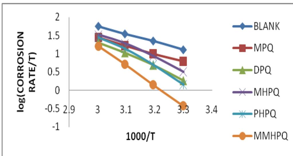
**Figure 4.** Transition state plot for mild steel corrosion in 1M H<sub>2</sub>SO<sub>4</sub> in the absence and presence of 1mM concentration of the inhibitors
