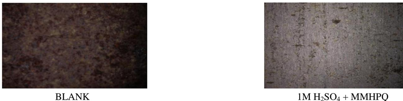
**Figure 8.** Optical Microscope images of mild steel surface without and with the addition of MMHPQ
