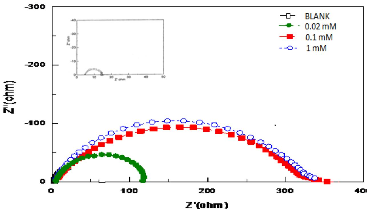
**Figure 7.** Nyquist diagram for mild steel in 1M H<sub>2</sub>SO<sub>4</sub> for the selected concentrations of inhibitor MMHPQ
