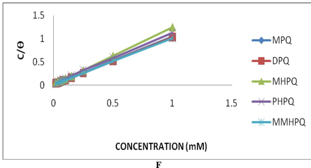
figure 5. Langmuir plot of inhibitors in 1M H<sub>2</sub>SO<sub>4</sub>
