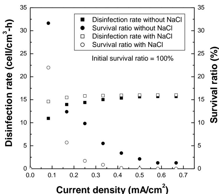
**Figure 4** Effect of current density on  $R_d$  and  $R_s$  in both presence/absence of 3 mg/l sodium chloride salt in raw water disinfected using ACF electrodes.
