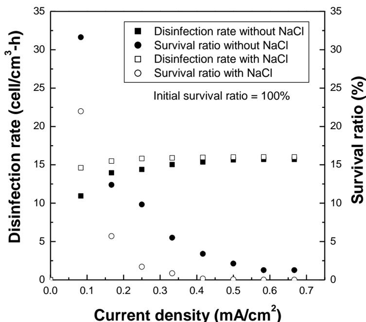
**Figure 4** Effect of current density on  $R_d$  and  $R_s$  in both presence/absence of 3 mg/l sodium chloride salt in raw water disinfected using ACF electrodes.
