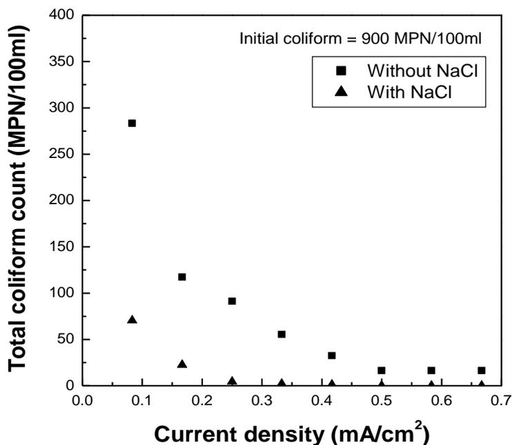
**Figure 2.** Effect of current density on TCC in both presence/absence of 3 mg/l sodium chloride salt in raw water disinfected using ACF electrodes.
