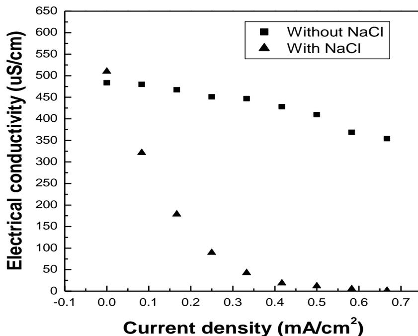
**Figure 3** Effect of current density on EC in both presence/absence of 3 mg/l sodium chloride salt in raw water disinfected using ACF electrodes.
