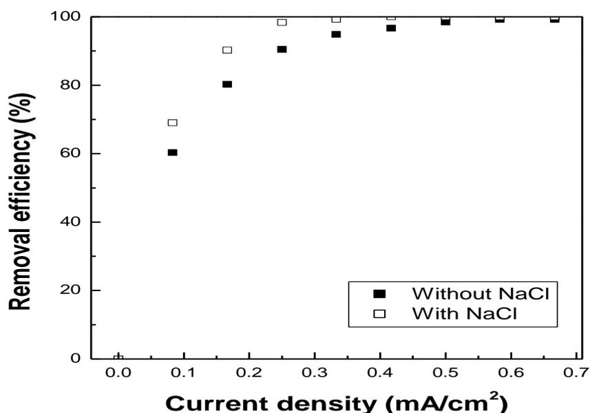
**Figure 5** Effect of current density on  $\eta$  in both presence/absence of 3 mg/l sodium chloride salt in raw water disinfected using ACF electrodes.
