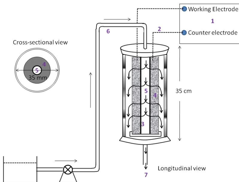
**Figure 1.** Schematic diagram of the electrochemical disinfection tubular reactor. Purple numbers represent the following: 1- DC power supply, 2- copper wires, 3- ion exchange membrane, 4- ACF electrodes, 5- glass bar, 6 – water inlet, 7- treated water outlet.
