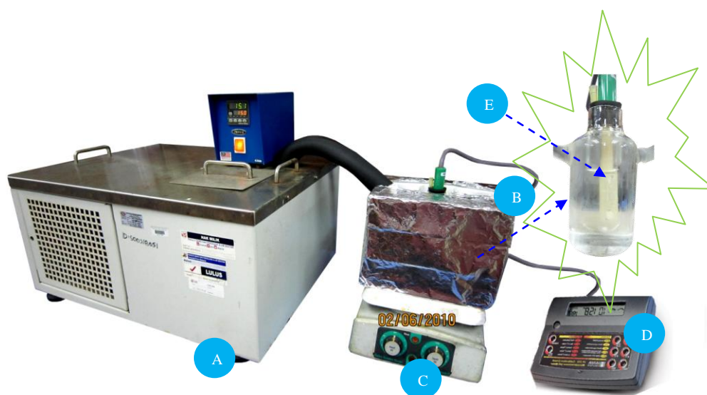
Scheme 2. Conductometric instruments. A) water bath, B) water-jacketed cell, C) magnetic mixer, D) conductometer, E) conductivity electrode
