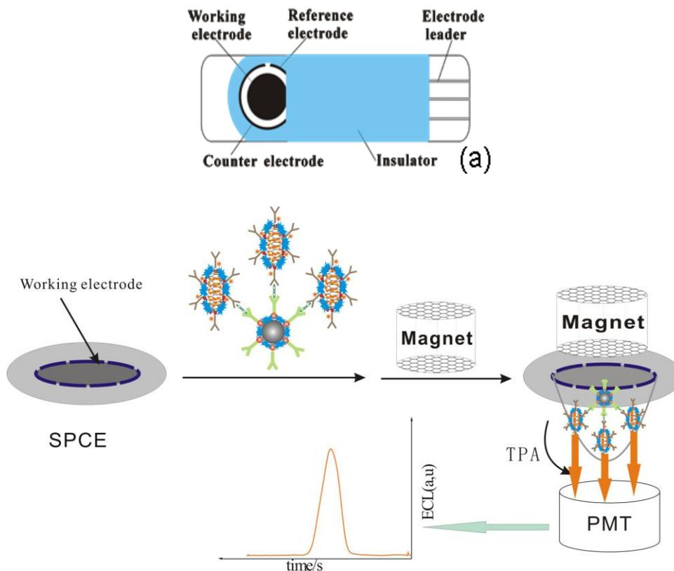
**Scheme 4.** (a) Schematic illustration of three-electrode SPCE system; (b) The process of ECL measurements
