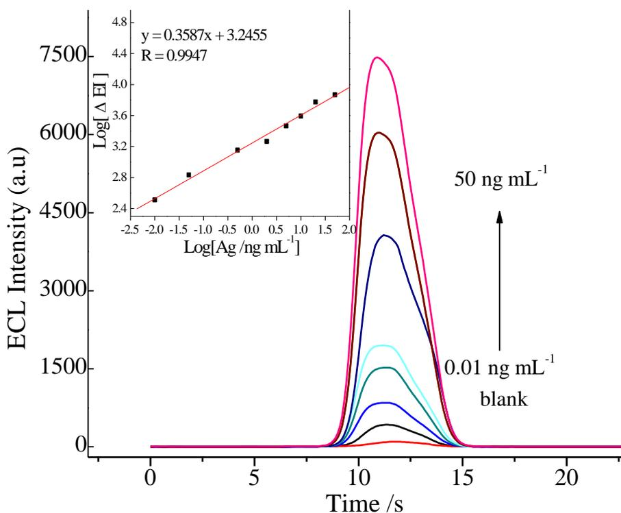
**Figure.4.** The schematic illustration of the ECL profiles of the immunosensor before (0.00 ng·mL<sup>-1</sup>) and after (0.01 ng·mL<sup>-1</sup>-50 ng·mL<sup>-1</sup>) incubating in different concentration of AFP. Insert: the relationship between log of  $\Delta\text{ECL}$  signal towards log of different AFP concentrations
