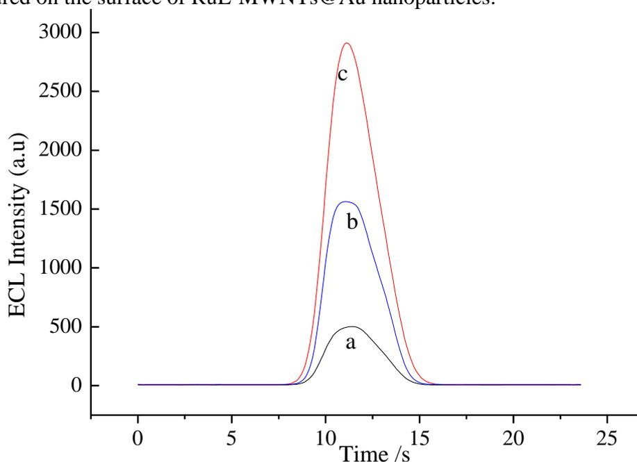
**Figure.3.** ECL-time curves for (a) RuL-Ab2, (b) RuL-MWNTs@Au~Ab2 and (c) RuL-MWNTs@Au~RuL-Ab2 modified electrodes in PBS (pH 7.4) containing  $10^{-5}$  M TPA.
